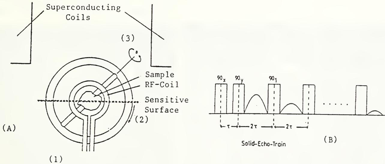
Fig. 1 (A) Schematics of probe movement: (1)linear motion along Z-axis, (2) sample rotation in YZ-plane,(3) second rotation of the sample to get a three-dimensional imaging; (B) multipulse train to detect solid echoes.
