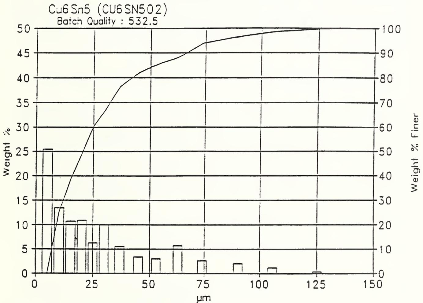
Fig. 1 Particle size distribution for atomization of Cu<sub>6</sub>Sn<sub>5</sub>
