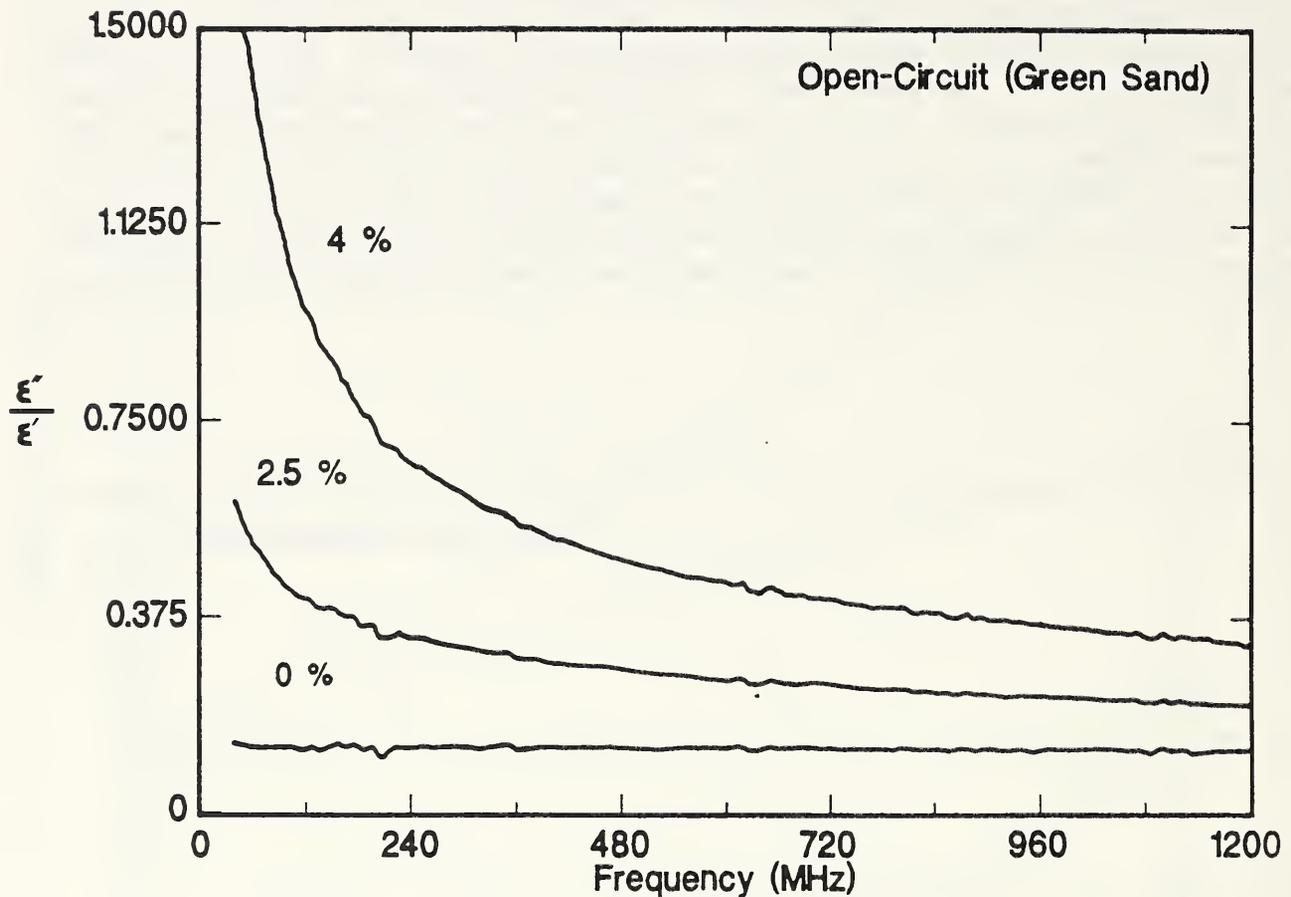
Fig. 4 Loss tangent,  $\epsilon''/\epsilon'$ , versus frequency using an open-circuit sample holder for greensand samples prepared with 0, 2.5, and 4 percent moisture content.
