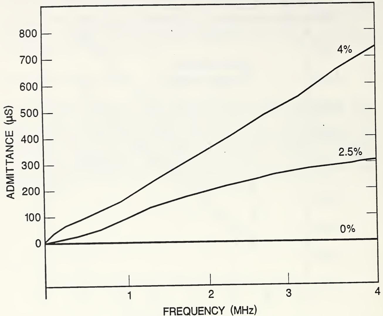
Fig. 2  $\text{Re}(Y)$  (real part of capacitive probe admittance) versus frequency for several values of greensand moisture content.
