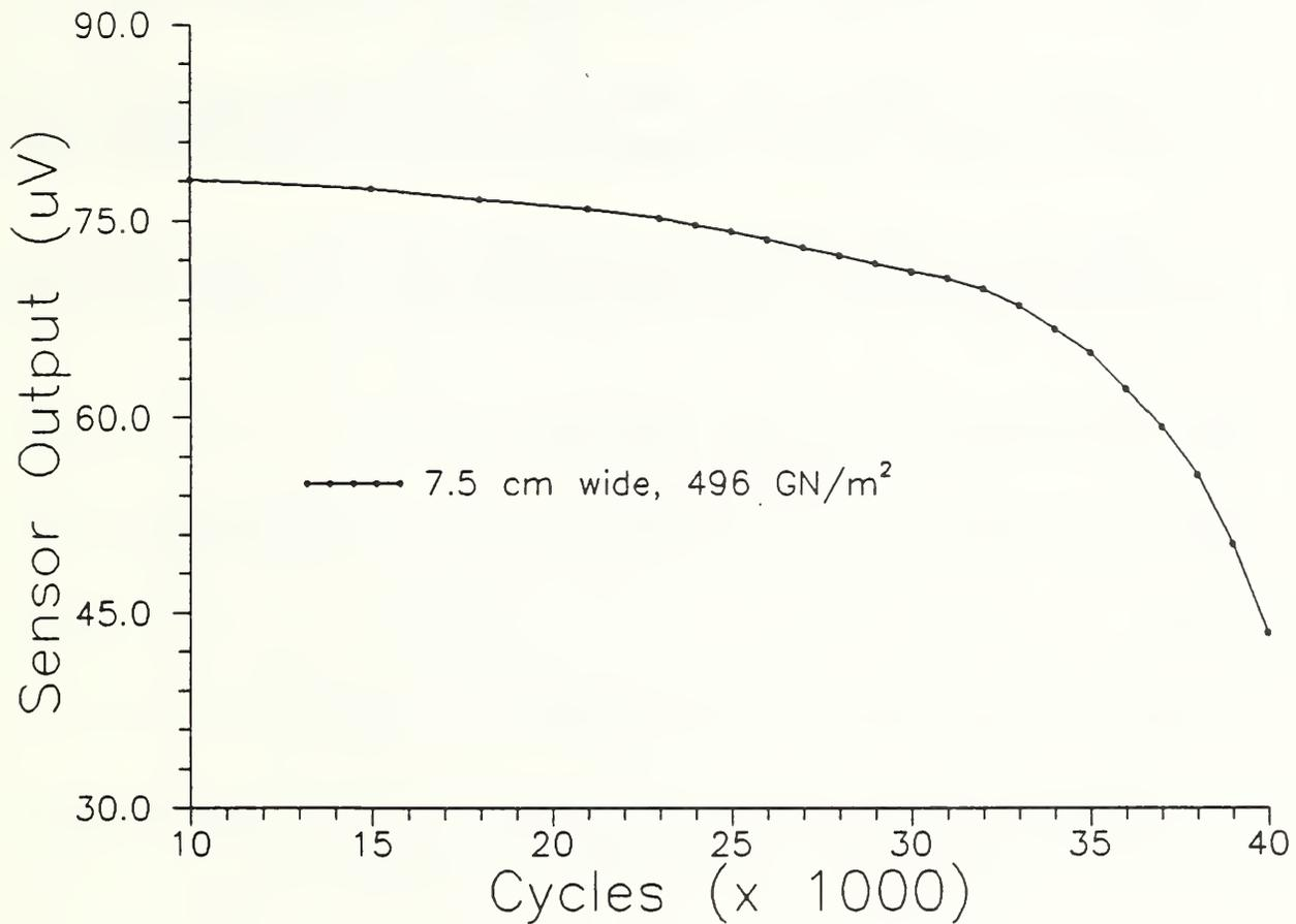
Fig. 2 Sensor output vs load cycles for 7075-T6 aluminum four-point bend specimen containing a stress concentration.
