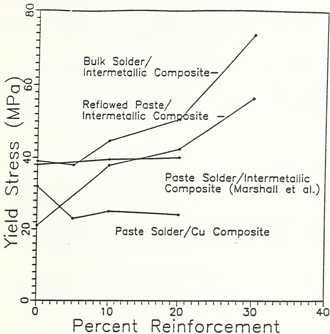
Fig. 2 Compressive yield strength of particulate composite solders as a function of reinforcement level
