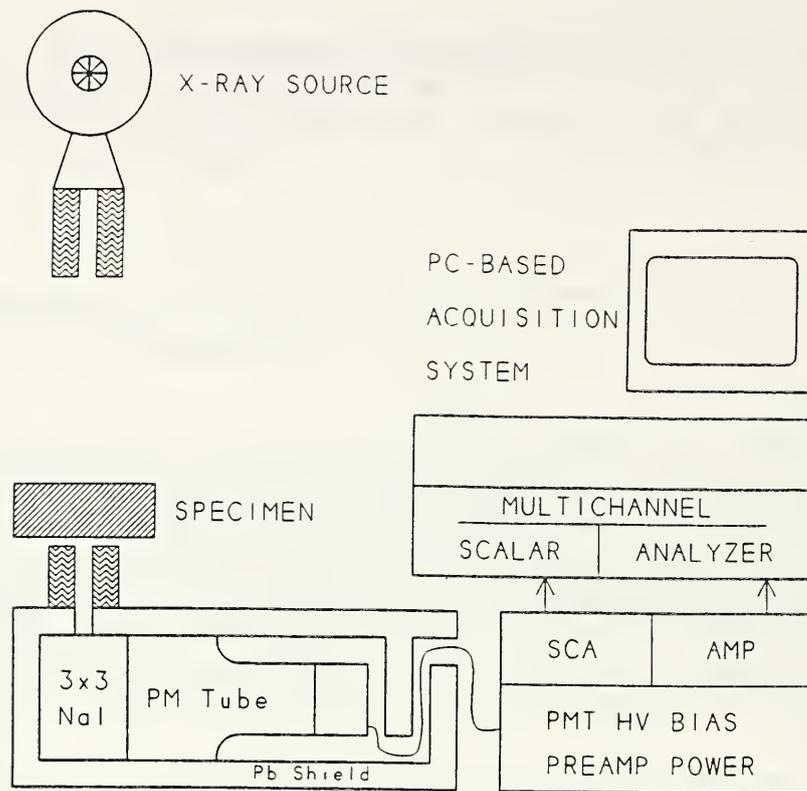
Fig. 2 Schematic of NIST prototype system for in-situ measurement of fiber-volume in composite materials.
