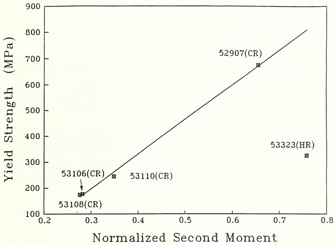
Fig. 2. Correlation between yield strength and a characteristic of the curves in Fig. 1.
