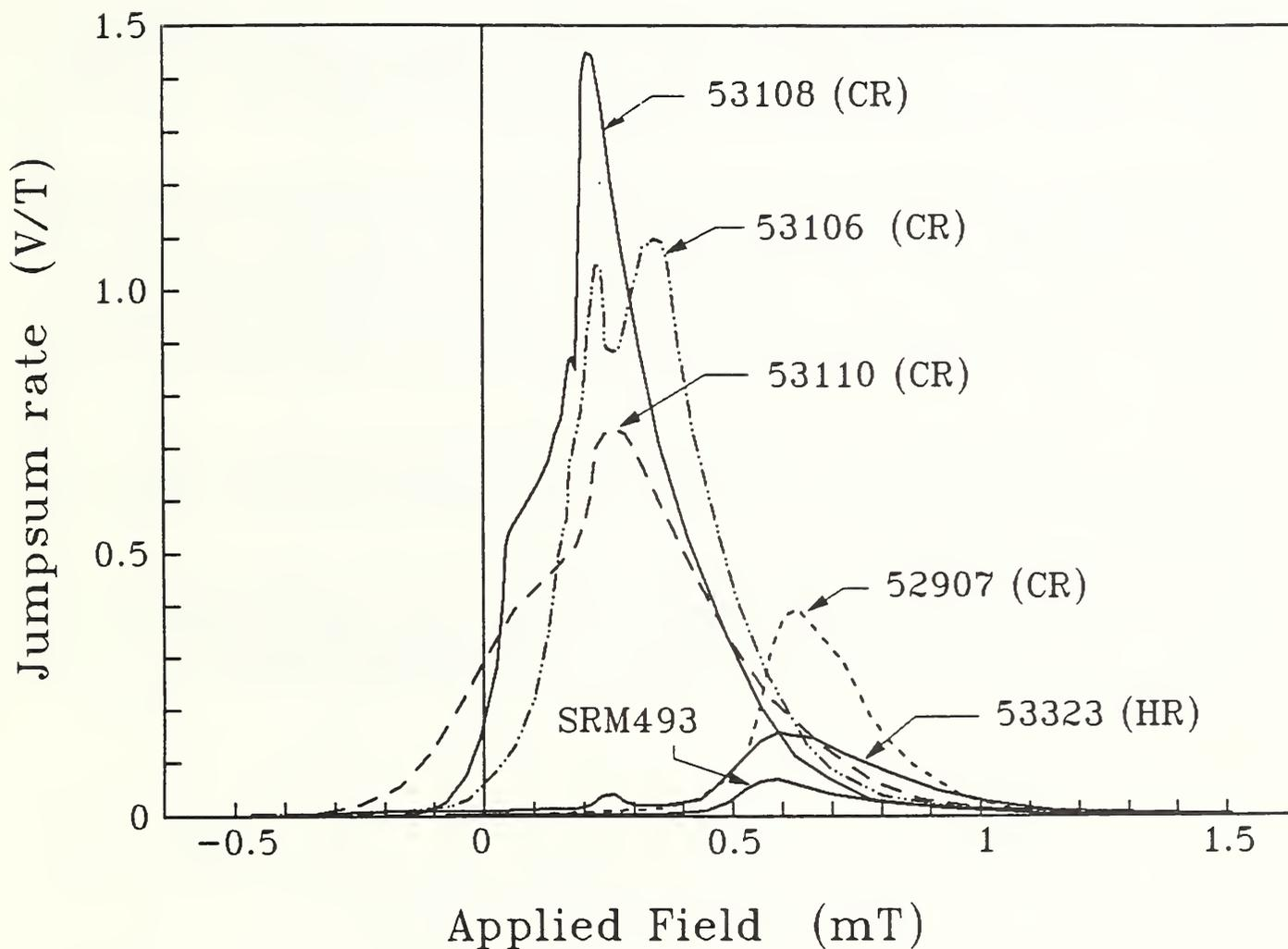
Fig. 1 Barkhausen noise data obtained during analysis of cold rolled (CR) and hot rolled (HR) mild steel sheet and standard reference material SRM 493
