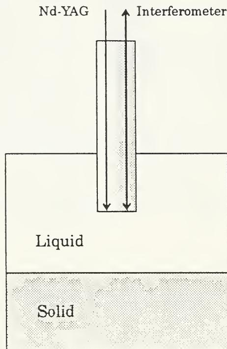
Fig. 2 Laser-ultrasonic configuration consisting of a Nd-YAG pulsed laser for ultrasonic generation and an interferometer for detection where laser light is passed through a transparent rod to the liquid metal.
