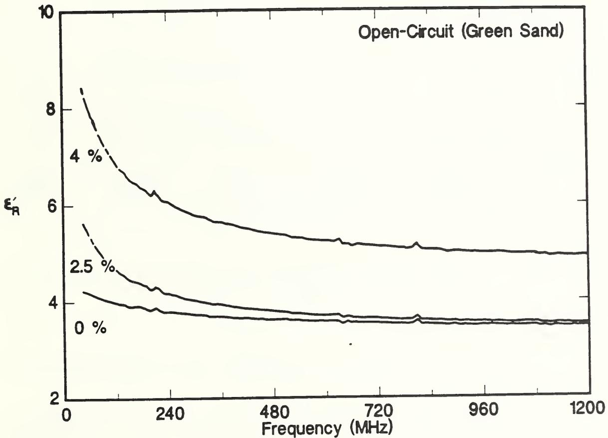
Fig. 3  $\epsilon'_R$  for versus frequency using an open-circuit sample holder in greensand samples prepared with 0, 2.5, and 4 percent moisture content.
