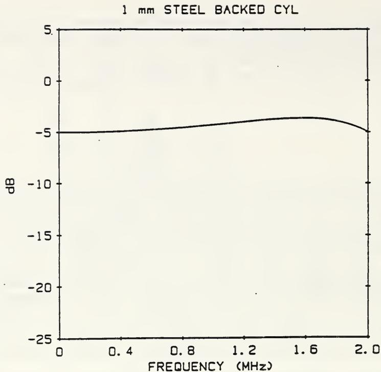
Fig. 2 Calculated response of a transducer having PZT element 1 mm in diameter and 1 mm long with a steel backing.
