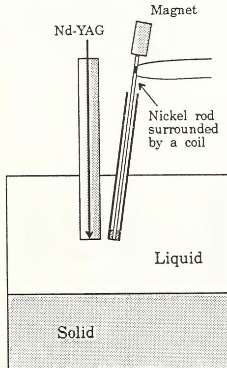
Fig. 1 Ultrasonic configuration consisting of an immersed magnetostrictive waveguide for ultrasonic reception and an immersed transparent rod through which pulsed Nd-YAG laser light is passed to generate ultrasonic pulses in the liquid metal.
