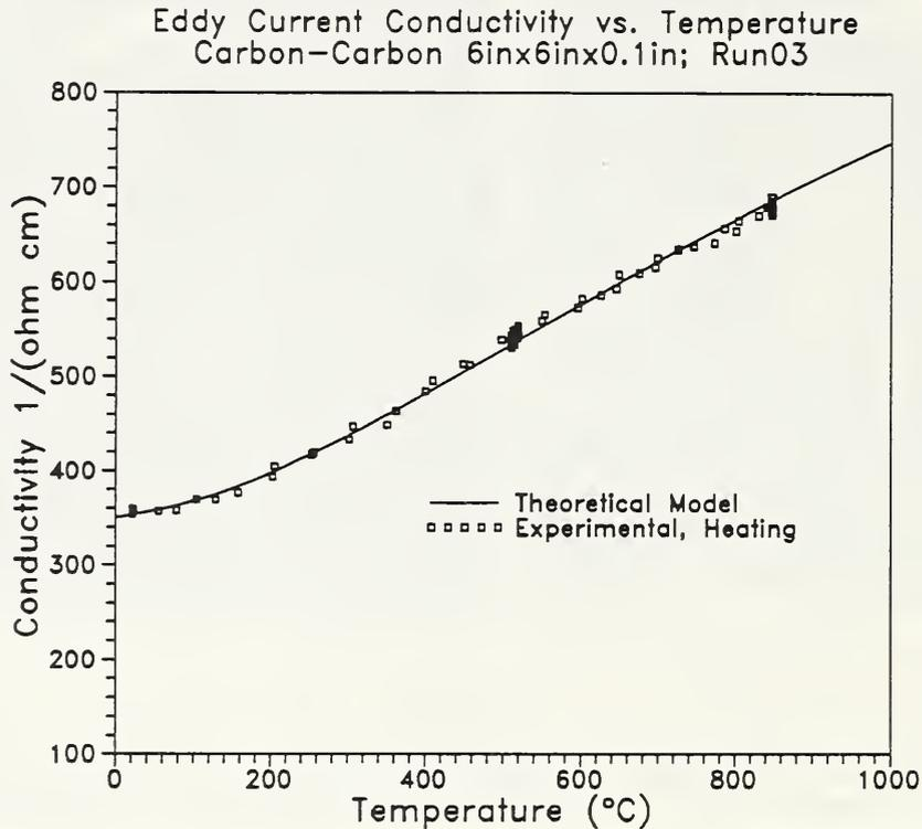
Fig. 1 Comparison between fitted model and eddy current conductivity of coated carbon-carbon plate.
