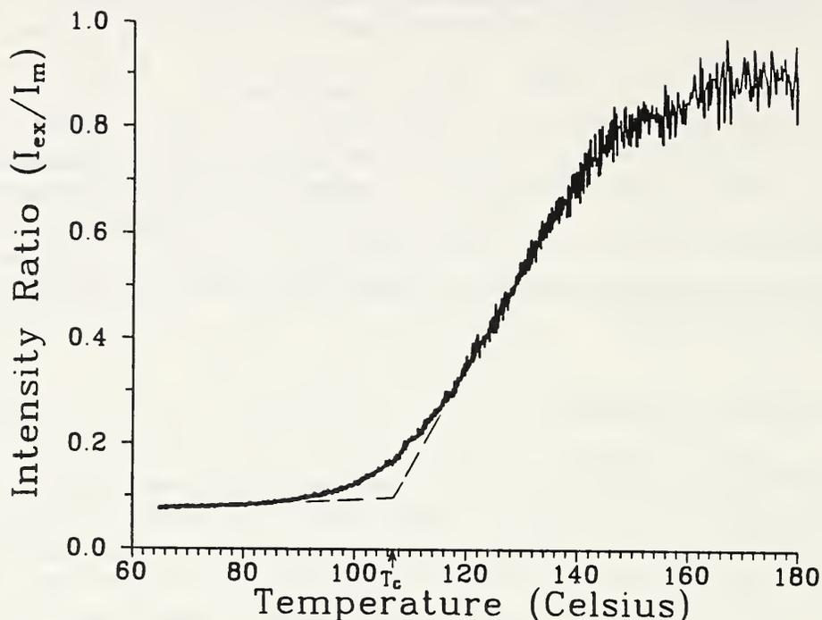
Fig. 1 The ratio of excimer to monomer fluorescence plotted versus temperature for polystyrene doped with BPP and excited with an excitation wavelength of 340 nm.
