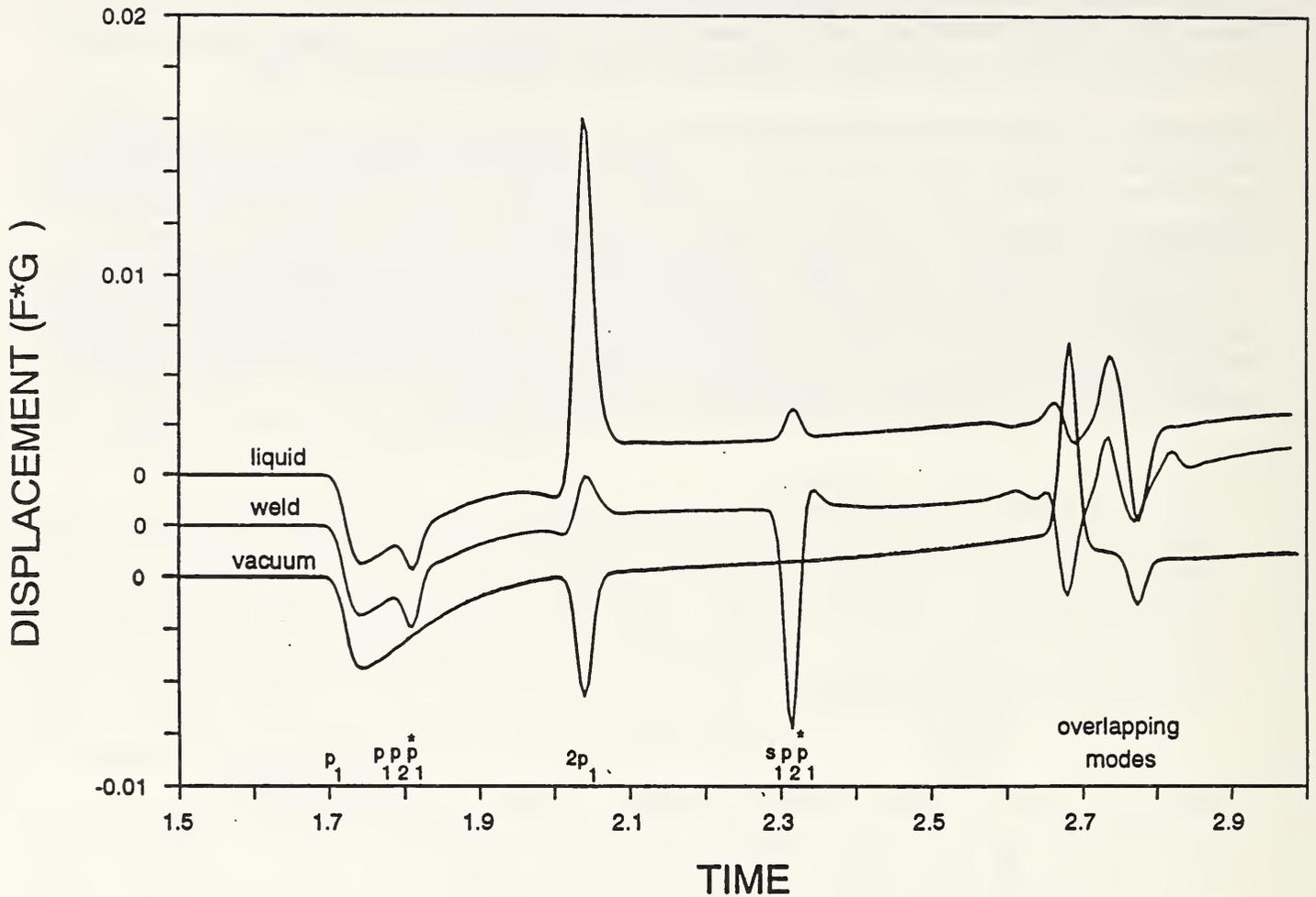
Fig. 2 Calculated vertical displacement waveform due to a pair of dipoles (laser source) for the configuration of Fig. 1: Liquid layer interface - transmits normal stress only. Vacuum interface - no interaction at interface. Welded interface - both stress and displacement are continuous.
