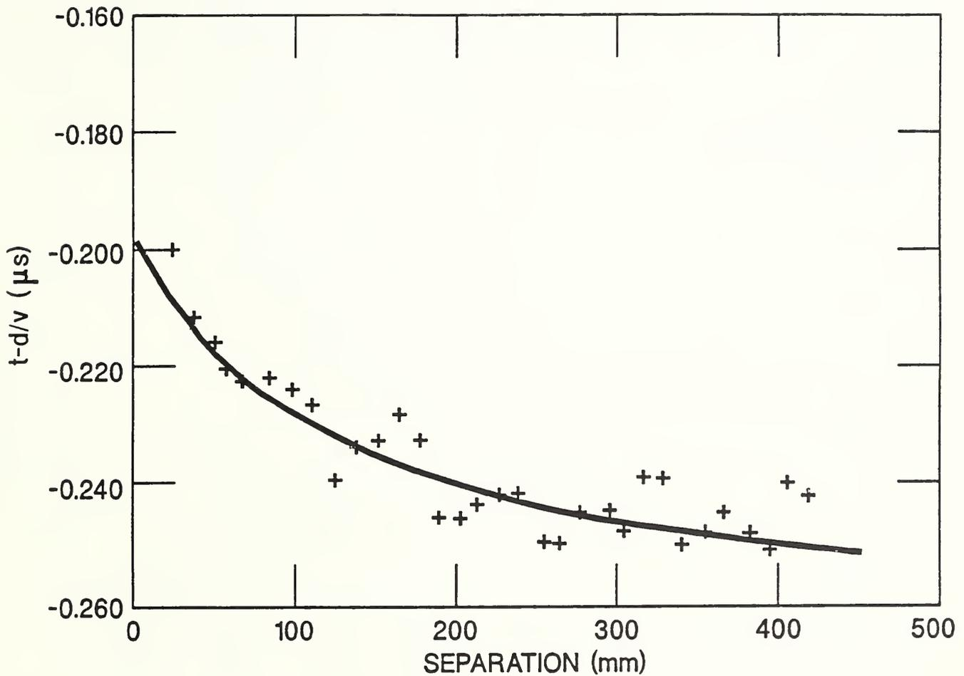
Fig. 1 Difference between measured arrival time,  $t$ , and diffraction and time,  $d/v$ , for a plane wave (solid line is theory)
