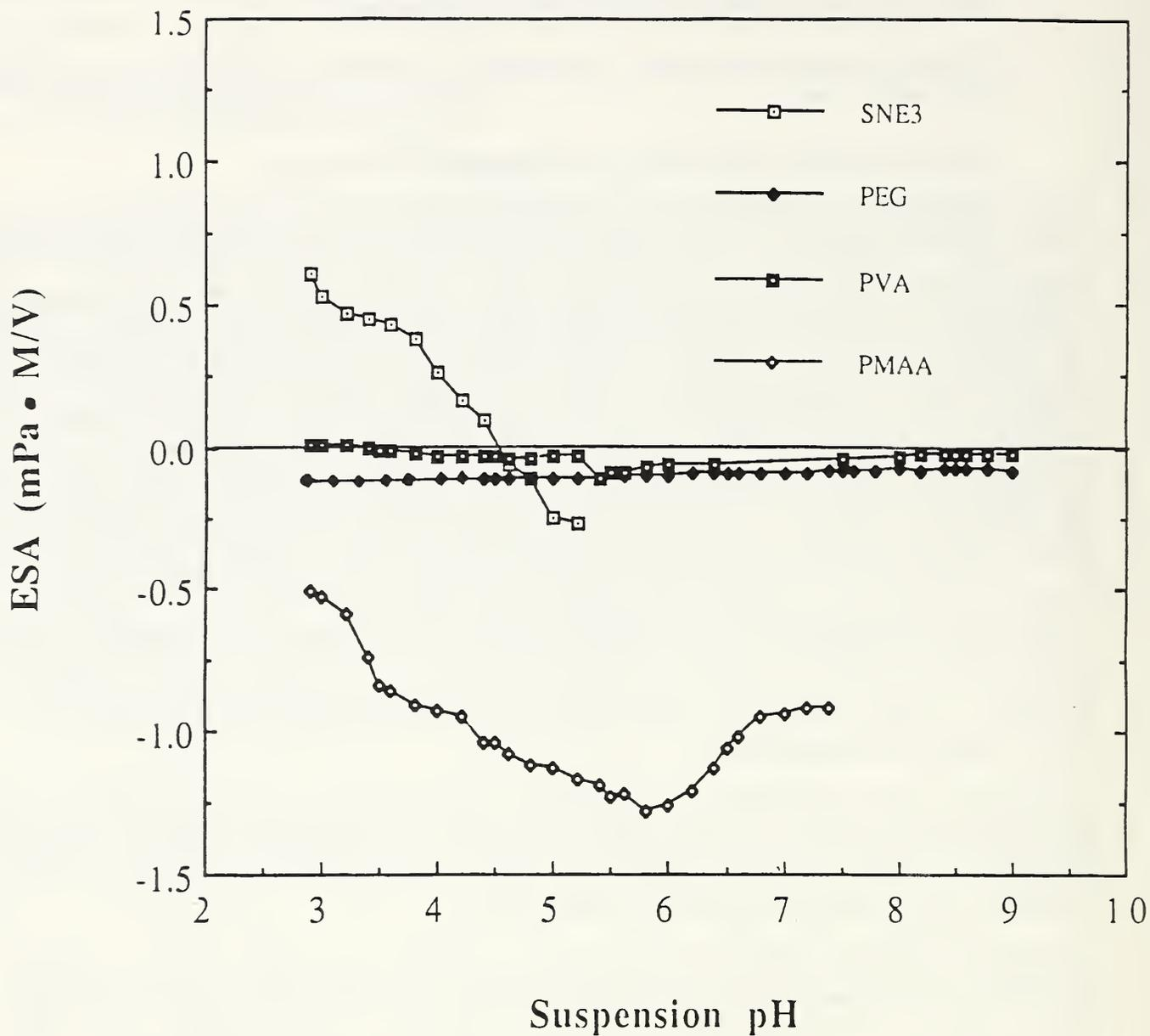
Fig. 1 Variation of ESA as a function of suspension pH for SNE-3 silicon nitride powder, polyethylene glycol (PEG, molecular wt. 3,400), polyvinyl alcohol (PVA, molecular wt. 50,000), and polymethacrylic acid (PMAA, molecular wt. 10,000).
