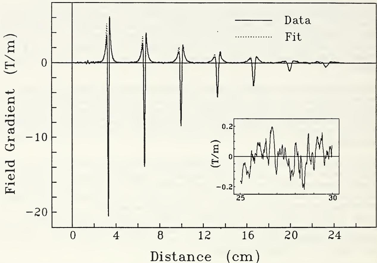
Fig. 1 Magnetic leakage field gradient from a magnetic particle test ring where the solid line represents the measured values and the dotted line represents a least squares fit to the data
