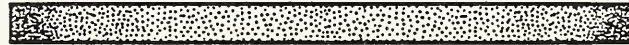
Figure 13. Edge-on view of plate showing increased current density concentration at edges of plate.
