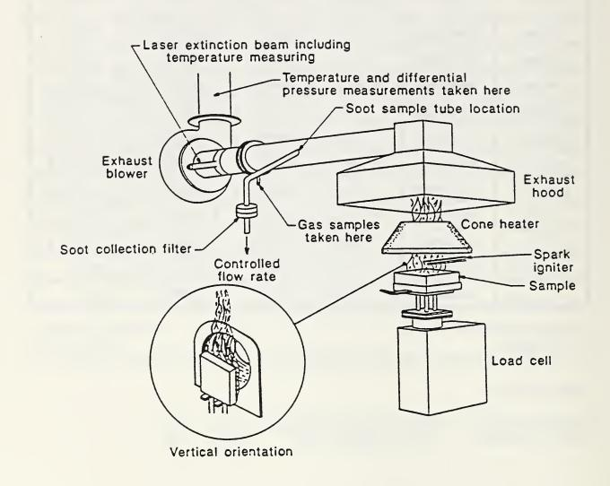
Figure 1. Schematic Diagram of the Cone Calorimeter.
