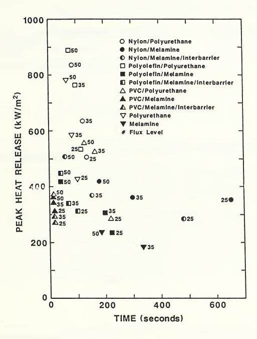
Figure 8. Peak Heat Release versus Time of Peak for 3 Flux Levels (25, 35, 50 kW/m<sup>2</sup>).
