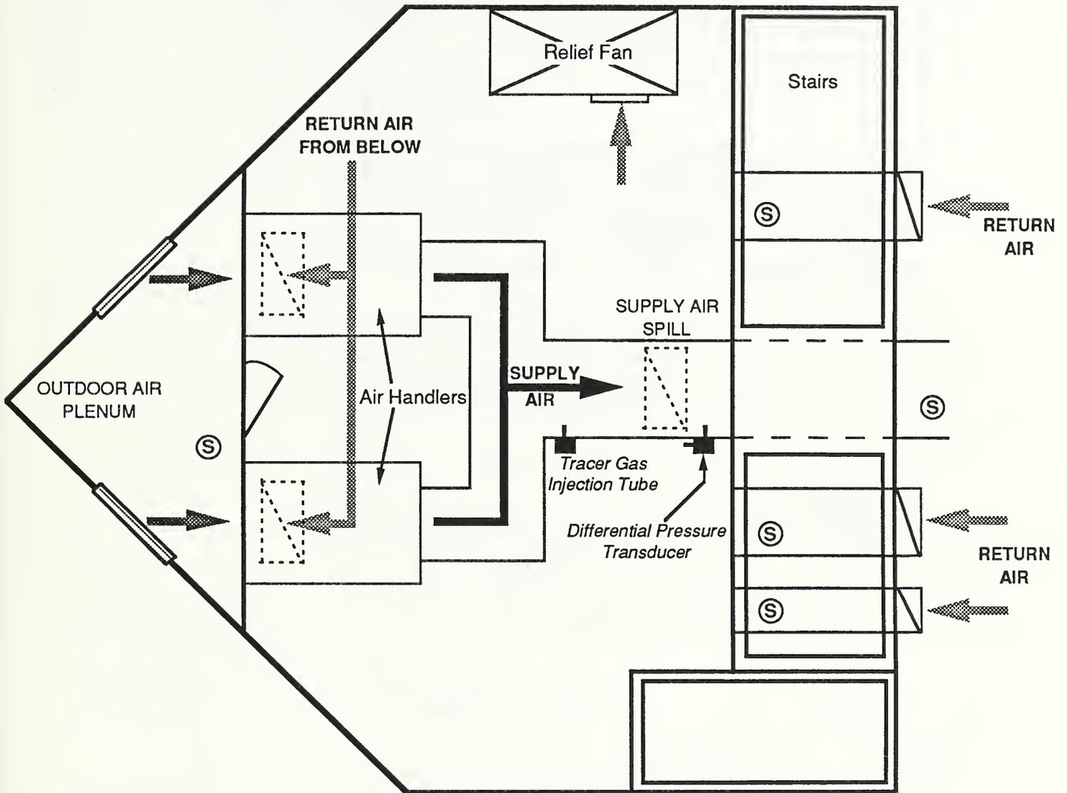
Figure 9 Schematic of Typical Mechanical Room
