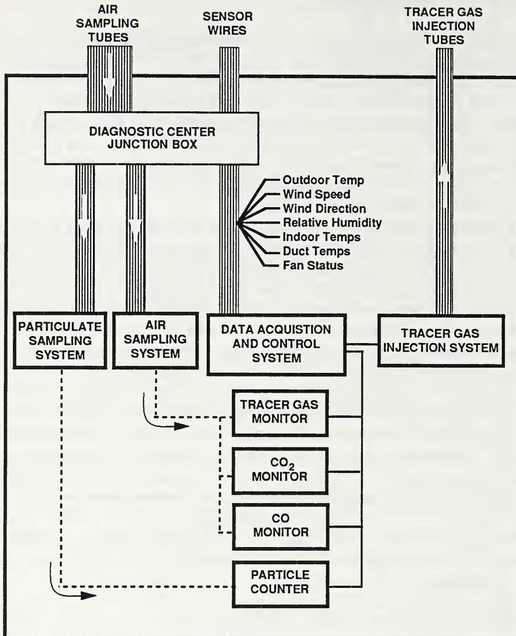
Figure 12 Schematic of Diagnostic Center
