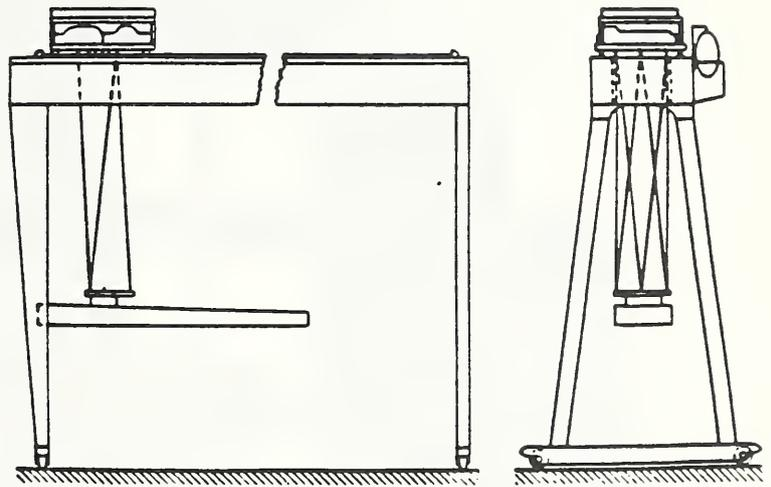
c) Gantry Bridge Crane (with extended reach)
