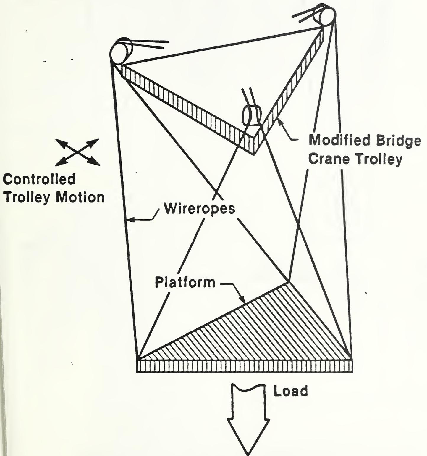
Figure 2. Design Concept for Improving Stiffness of Crane Suspension Mechanisms
