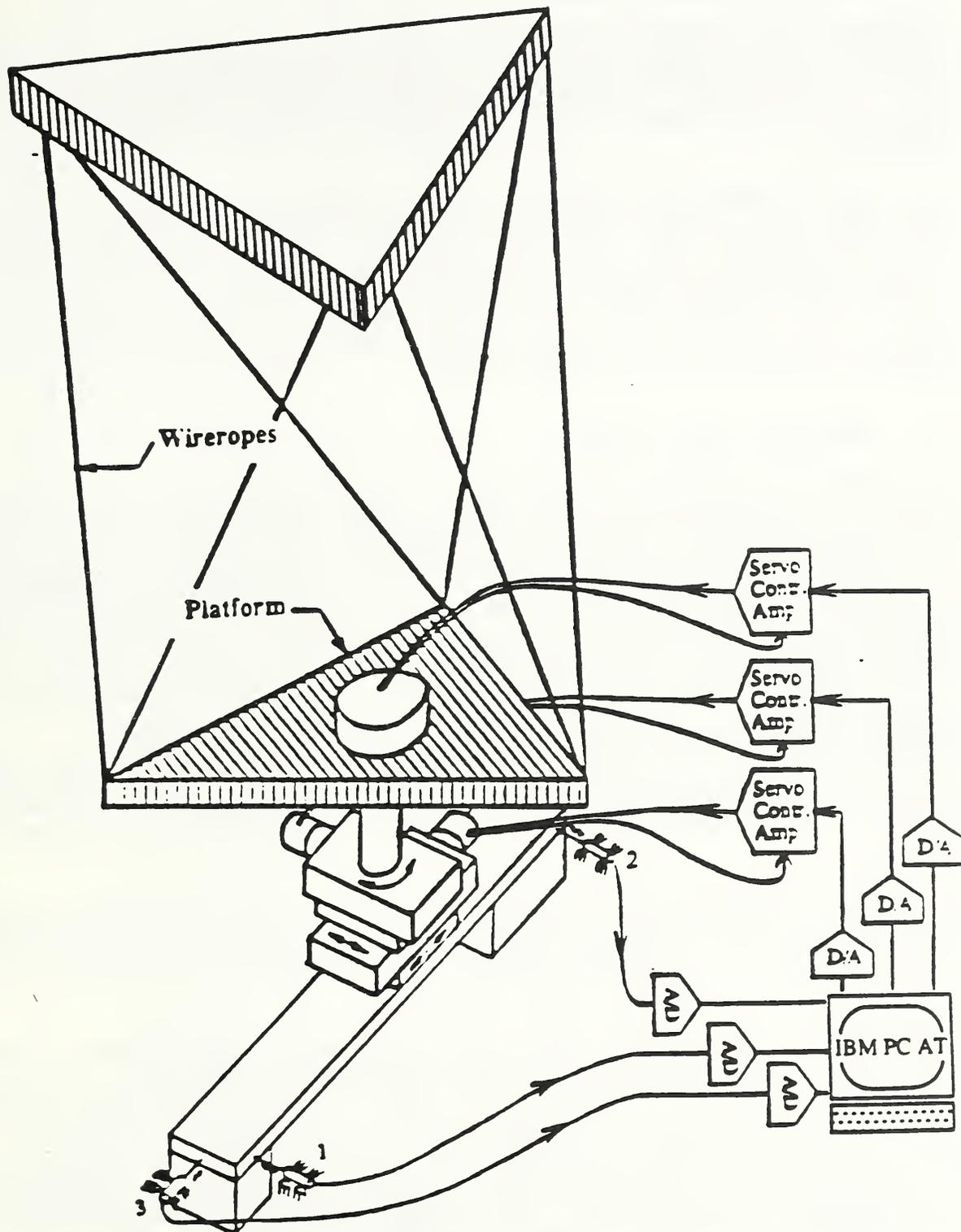
Figure 7. Schematic of the Vibration Compensation System
