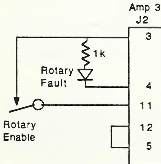
**FAULT AND ENABLE WIRING
