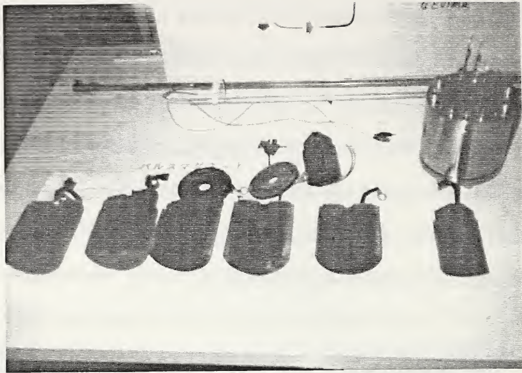
Figure 2. Cross sections of several magnet coils plus one complete coil (upper right) being studied at NRIM for use in construction of a several-millisecond, pulsed-field magnet.
