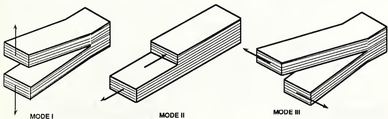
Figure 8 Fracture Toughness Testing
