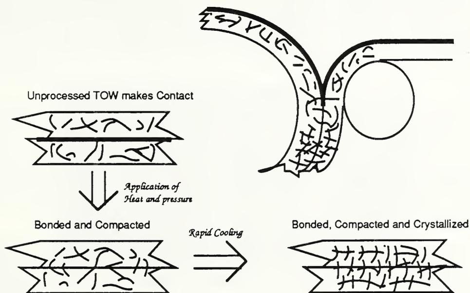
Figure 2 Thermoplastic Processing
