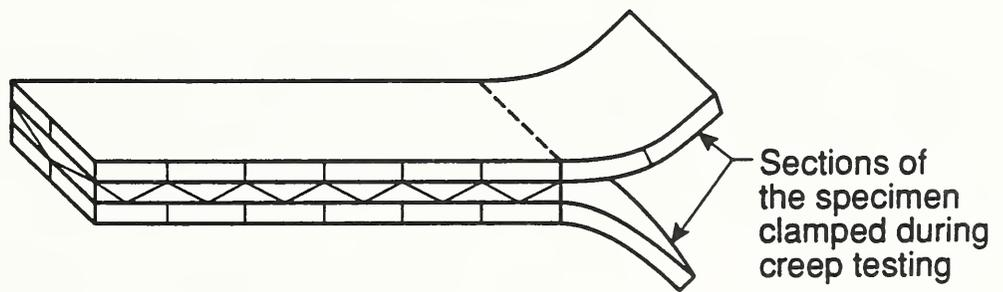
B. View of the Completed Test Specimen
