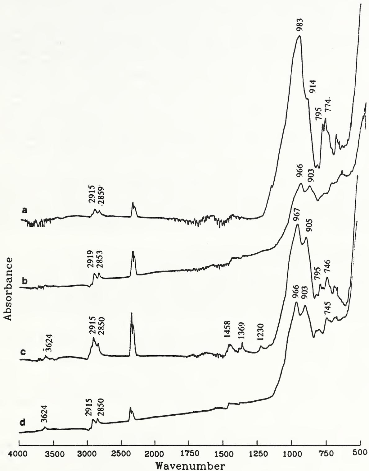
Figure 11. FTIR-ATR spectra of aged EPDM rubber: (a) uncleaned, (b) heptane cleaned (Method No. 1), (c) proprietary wash solution cleaned (Method No. 4), and (d) tap-water cleaned (Method No. 5)
