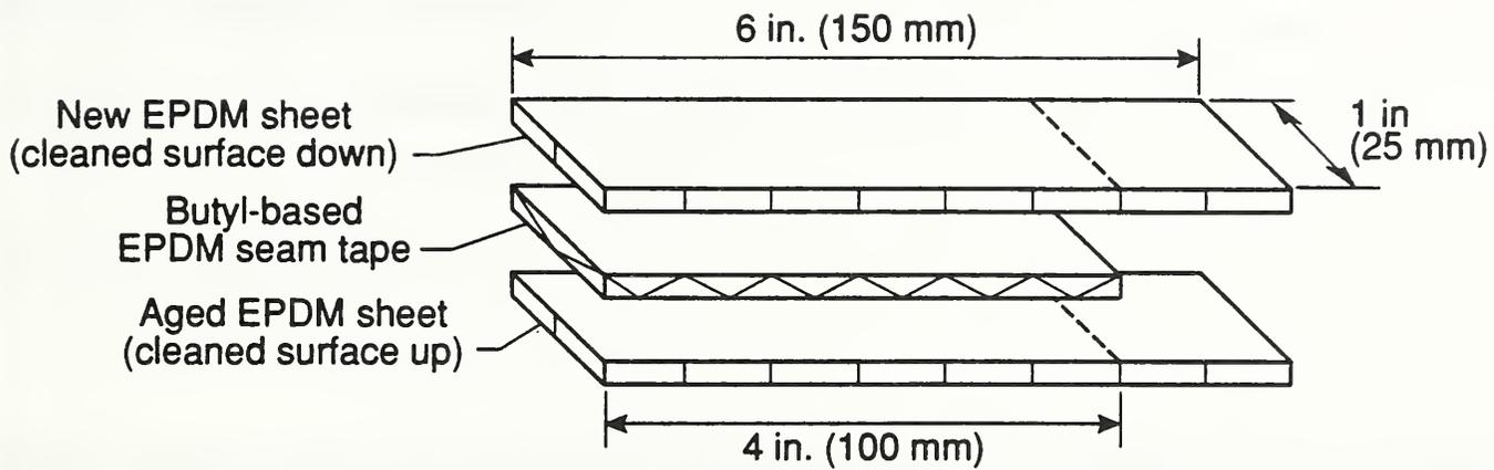
A. Exploded View of the Test Specimen
