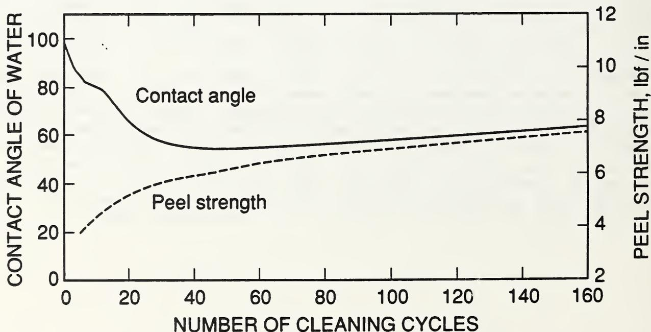
Figure 14. Relationship between peel strength and water contact angle as a function of cleaning cycles
