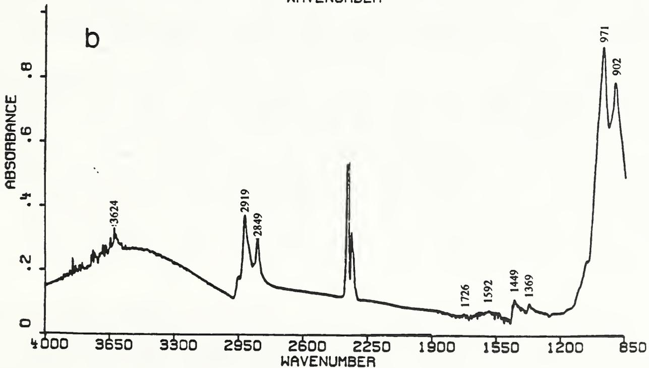
Figure 10. FTIR spectra: (a) transmission spectrum of the contaminants removed from aged EPDM rubber, and (b) ATR spectrum of cleaned (Method No. 11) aged EPDM
