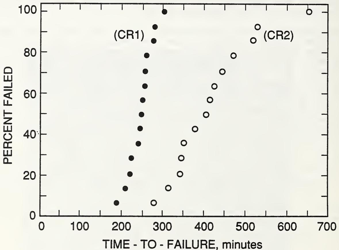
Figure 13. Results of the creep-rupture experiments: (CR1) new rubber bonded to aged rubber, and (CR2) new rubber bonded to new rubber
