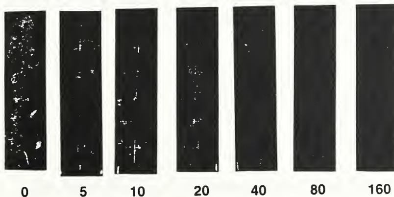
Figure 3. Surface appearance of the cleaned (Method No. 1) aged EPDM as a function of cycles
