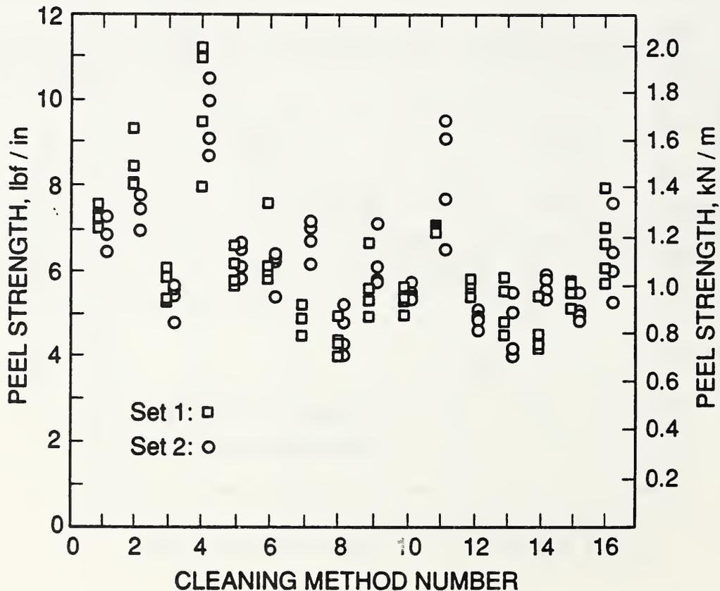
Figure 5. Peel strength as related to the surface cleaning method
