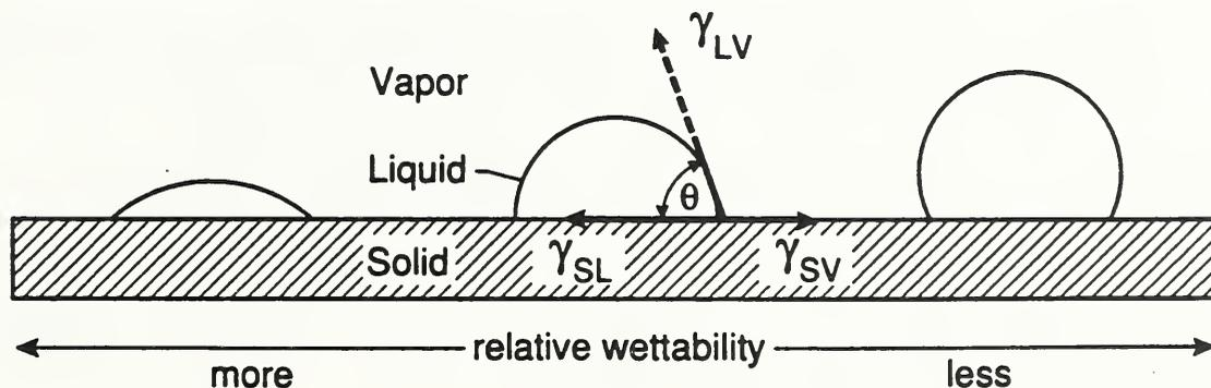
Figure 6. Contact angle and interfacial tensions for a drop of liquid resting on a solid surface:  $\theta$  - contact angle,  $\gamma_{LV}$  - liquid/vapor interfacial tension,  $\gamma_{SV}$  - solid/vapor interfacial tension,  $\gamma_{SL}$  - solid/liquid interfacial tension
