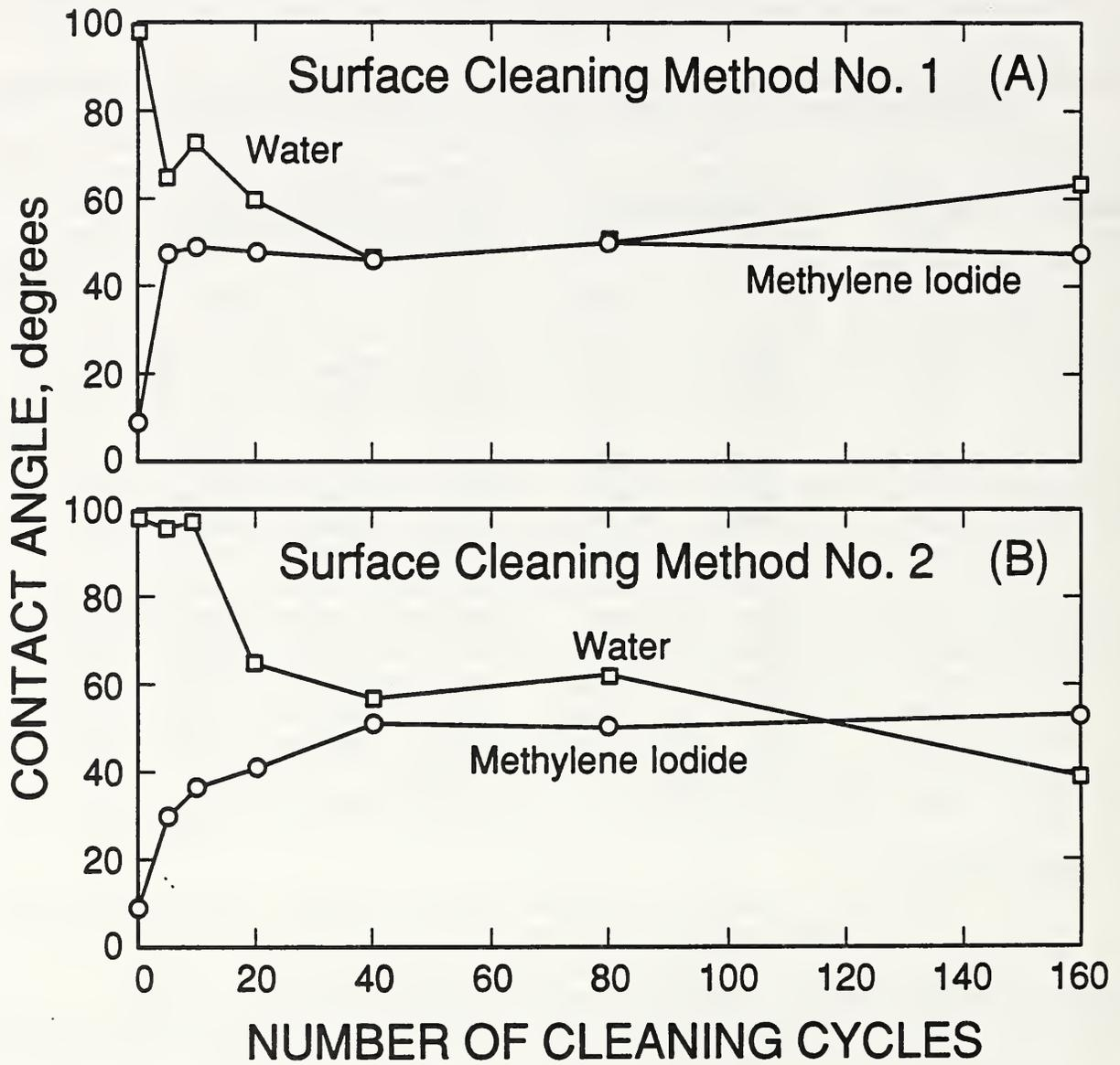
Figure 7. Water and methylene iodide contact angles of the aged EPDM as a function of the number of cleaning cycles: (a) surface cleaned with Method No. 1 and (b) surface cleaned with Method No. 2
