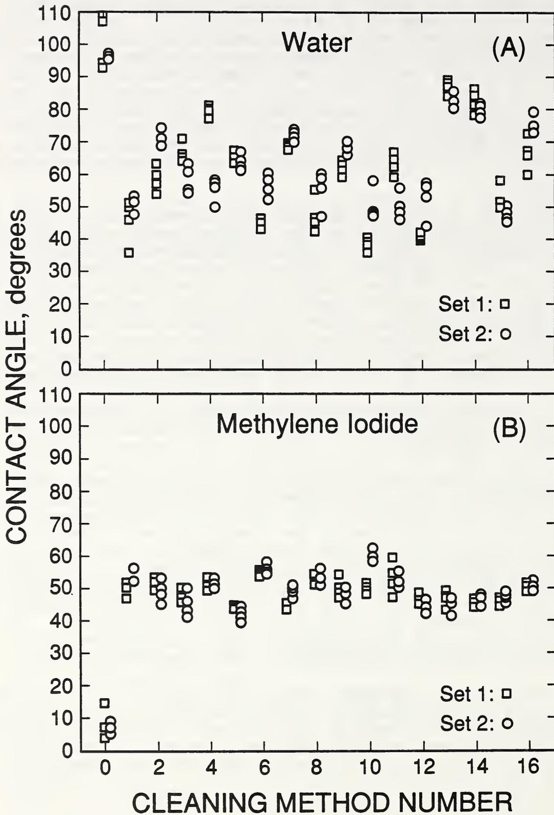
Figure 9. Contact angle as related to the cleaning method: (a) measured with water and (b) measured with methylene iodide
