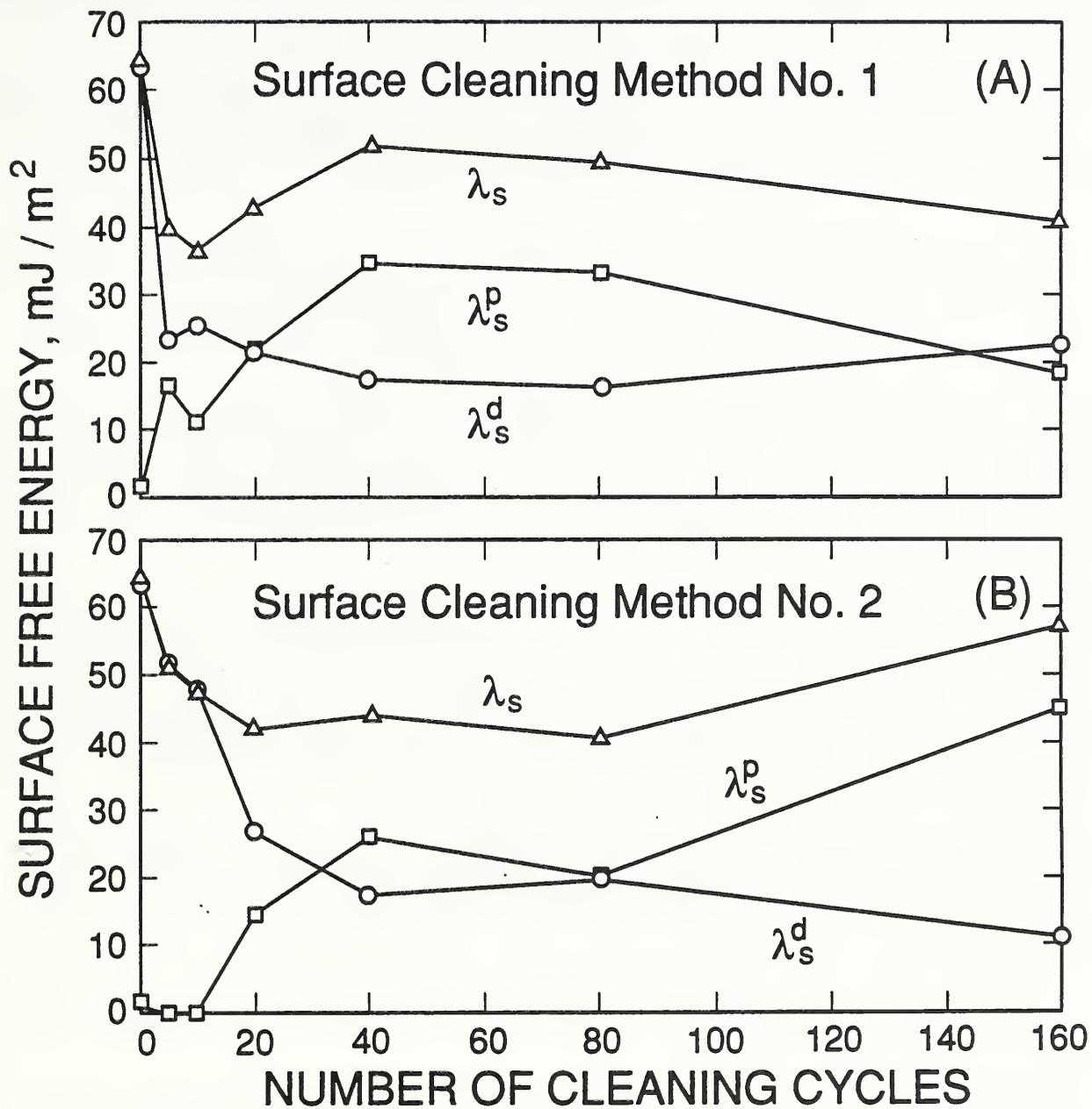
Figure 8. Surface free energies of aged EPDM as a function of the number of cleaning cycles: (a) surface cleaned with Method No. 1 and (b) surface cleaned with Method No. 2
