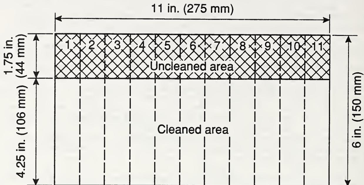
Figure 2. Sampling pattern used to select sections of the cleaned EPDM specimen for use in the peel tests, and the wettability, FTIR, and SEM analyses
