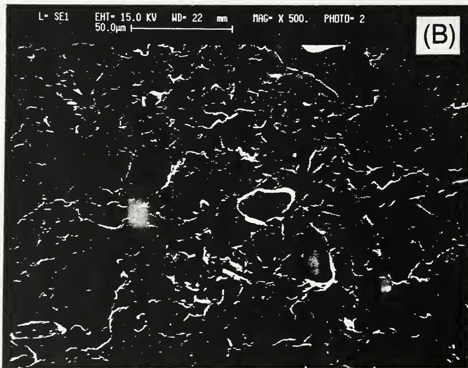
Figure 12. SEM photomicrographs: (a) typical cleaned rubber surface with platelet particles, and (b) a cleaned (Method No. 11) surface which was essentially free of platelet particles
