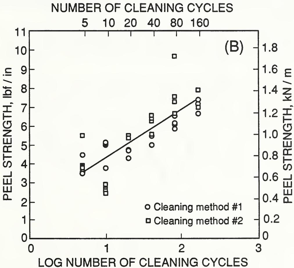
Figure 4. Peel strength of joints prepared from the aged EPDM versus: (a) the number of cleaning cycles, and (b) log of the number of cleaning cycles
