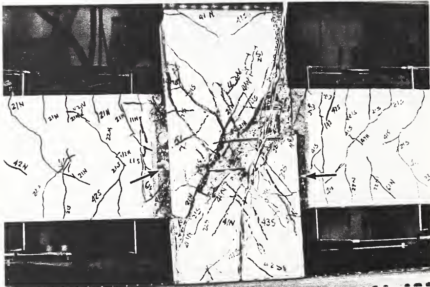
Fig. 4.5 Joint region of A-M-Z2 at 6 \Delta_y - east face.
