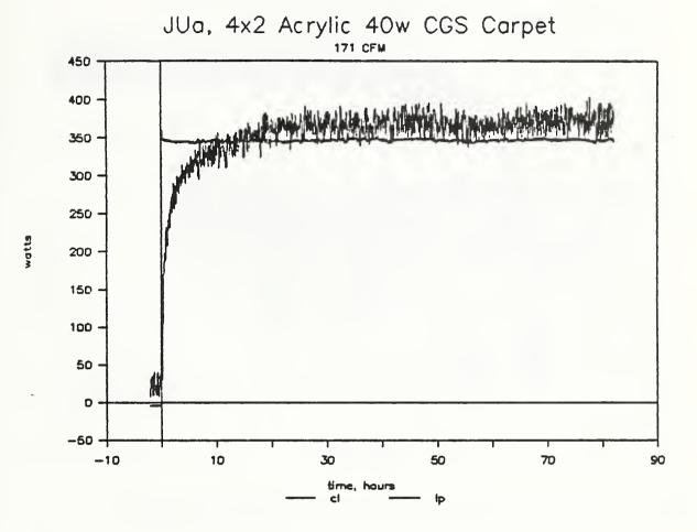
Figure 17. Measured lighting power and cooling load for transient test showing zero and full scale offsets
