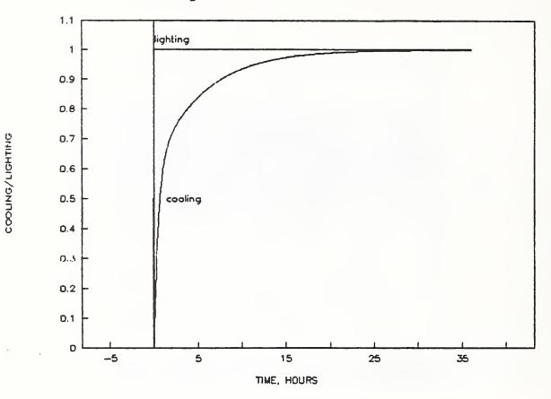
Figure 14. Cooling load profile with no excess heat gains or heat sources
