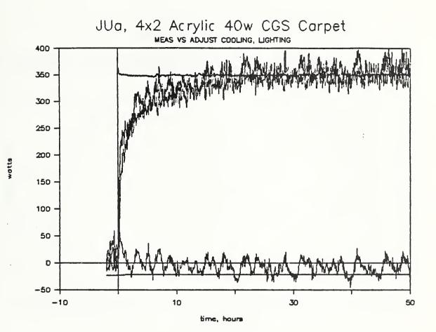
Figure 23. Measured cooling load adjusted using heat flow sensors vs. equilibrium calibration
