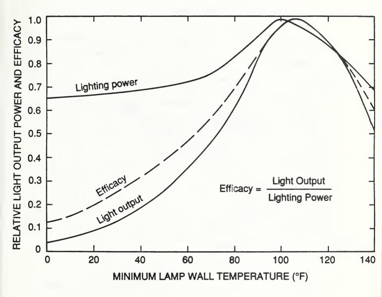
Figure 3. Temperature dependence of a typical fluorescent lamp
