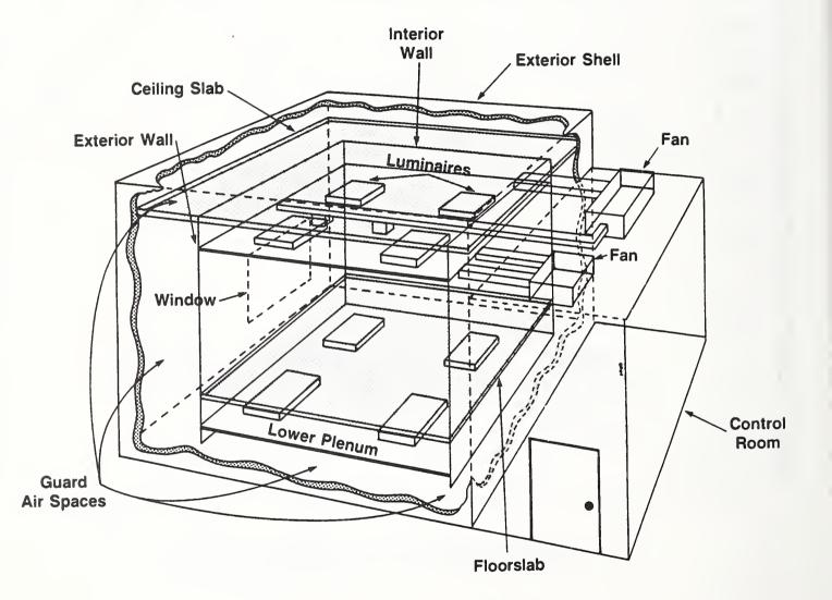
Figure 4. Cut-away schematic of the NIST Lighting/HVAC Interaction Test Facility
