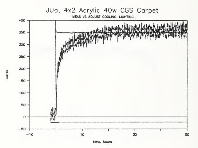
Figure 18. Measured cooling load adjusted for excess heat gains
