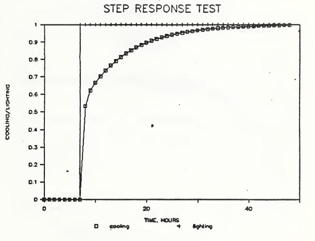
Figure 5. Transient test showing cooling load response due to switching of the lighting system
