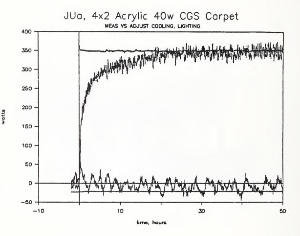
Figure 22. Excess heat gains based on heat flow sensor readings
