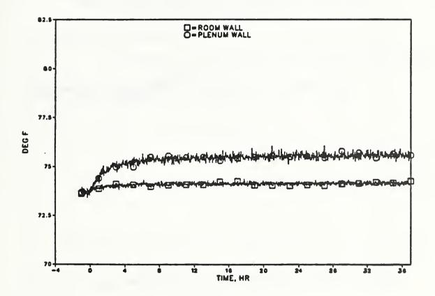
Figure 9. Measured room and plenum wall temperatures for a transient lights-on test
