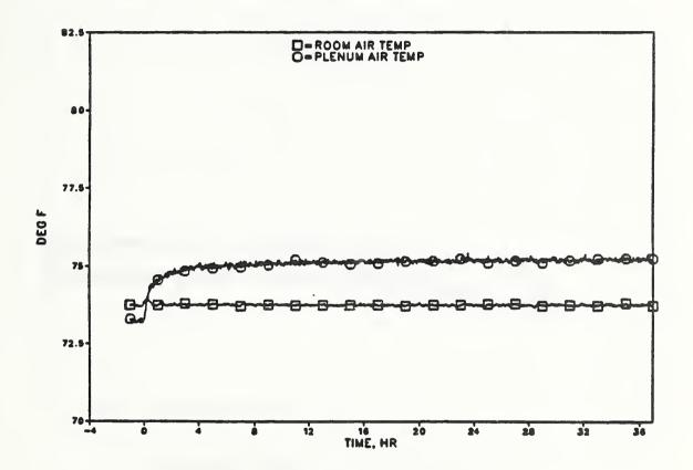
Figure 7. Measured room and plenum air temperatures for a transient lights-on test
