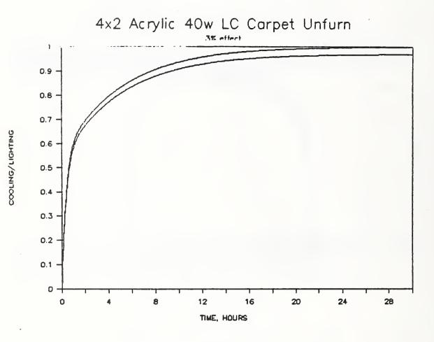
Figure 24. Cooling load profile with 3 percent offset
