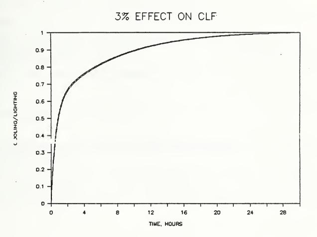
Figure 25. Normalized cooling load profile with 3 percent offset
