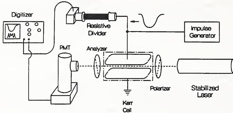
Figure 1. The experimental configuration for Kerr-cell vs. resistive divider comparison.
