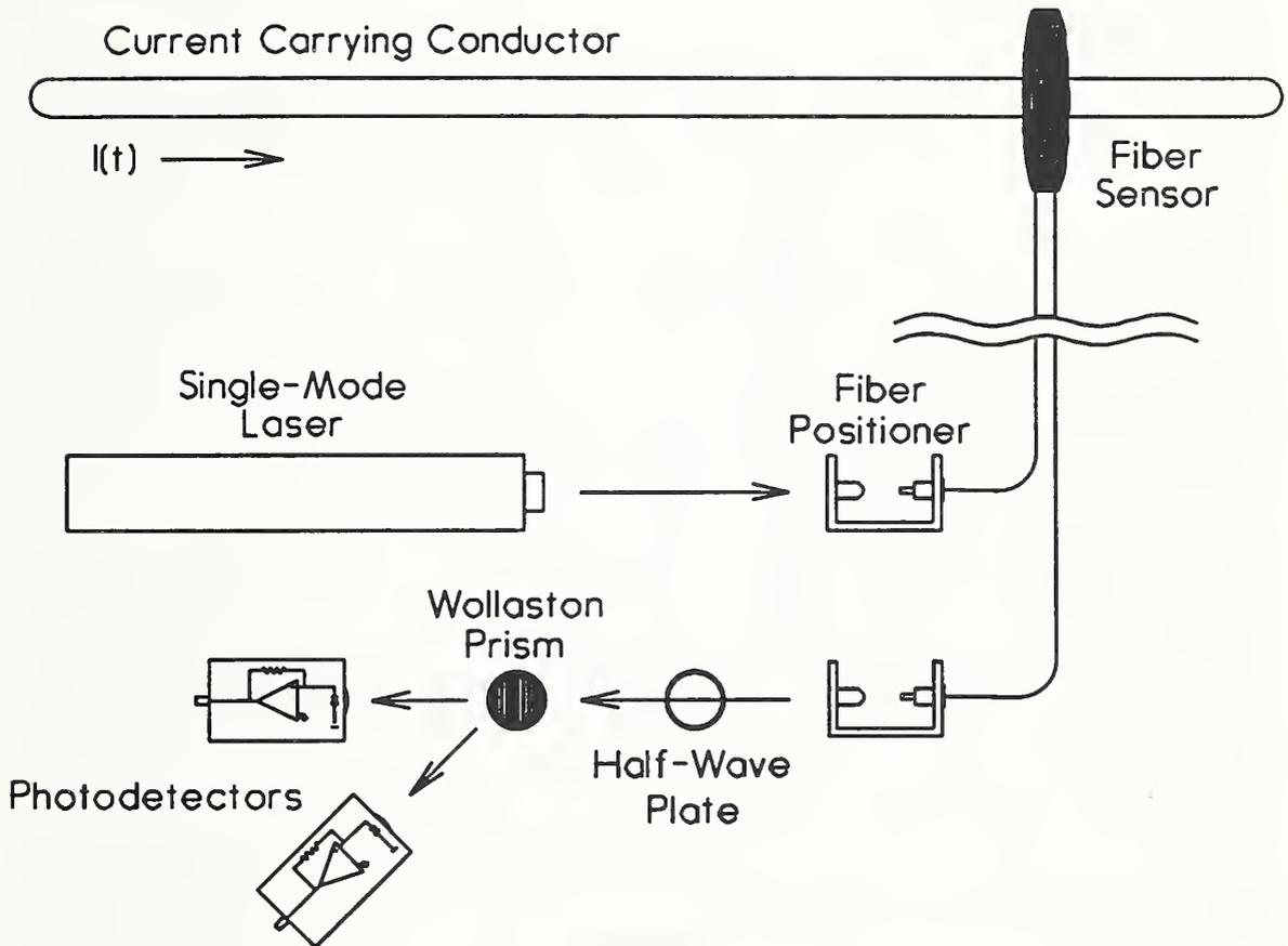
**Figure 8.** Magneto-optic current sensor system. The basic measurement system consists of a light source, fiber optics, optical sensing element, polarimetric optics, and photodetectors.
