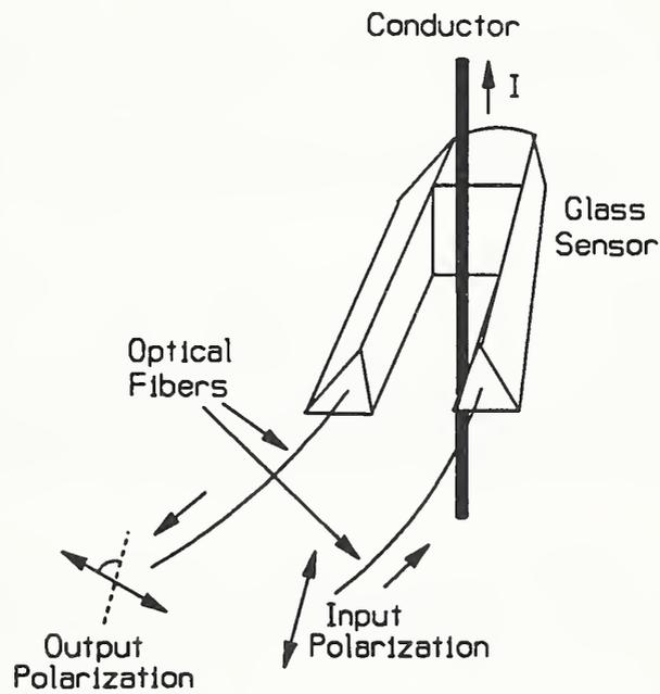
**Figure 9.** Bulk glass sensing element. The loop is open on one end to permit insertion of the conductor.
