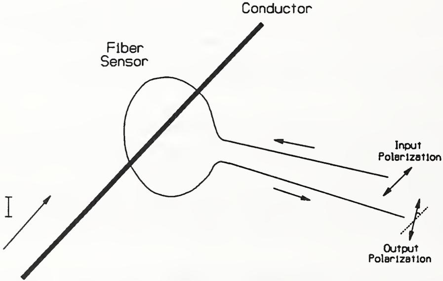
Figure 6. Optical current sensing element.
