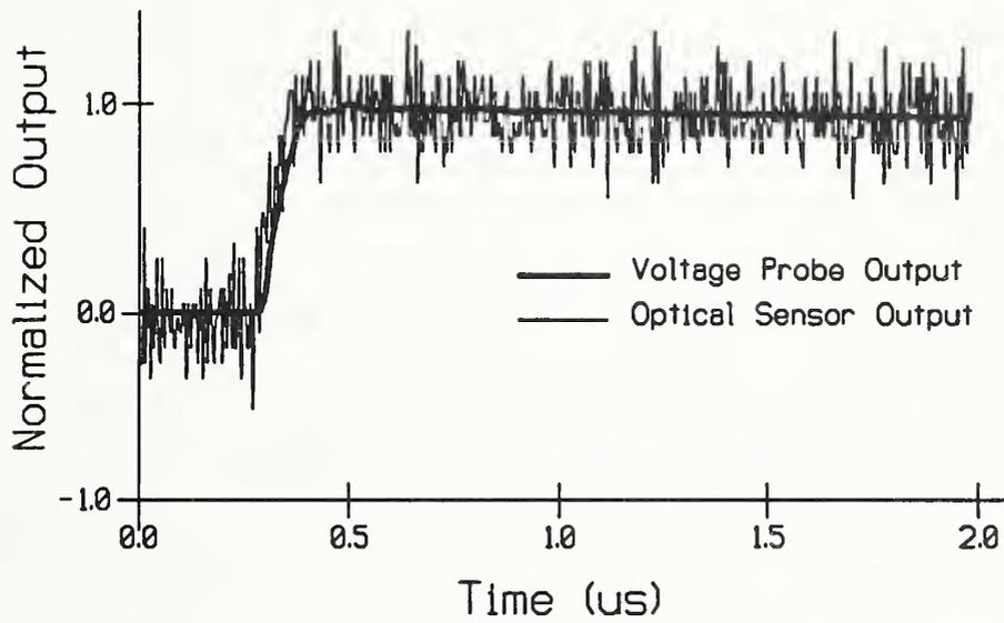
Figure 11. Normalized outputs of optical current sensor and voltage sensor
