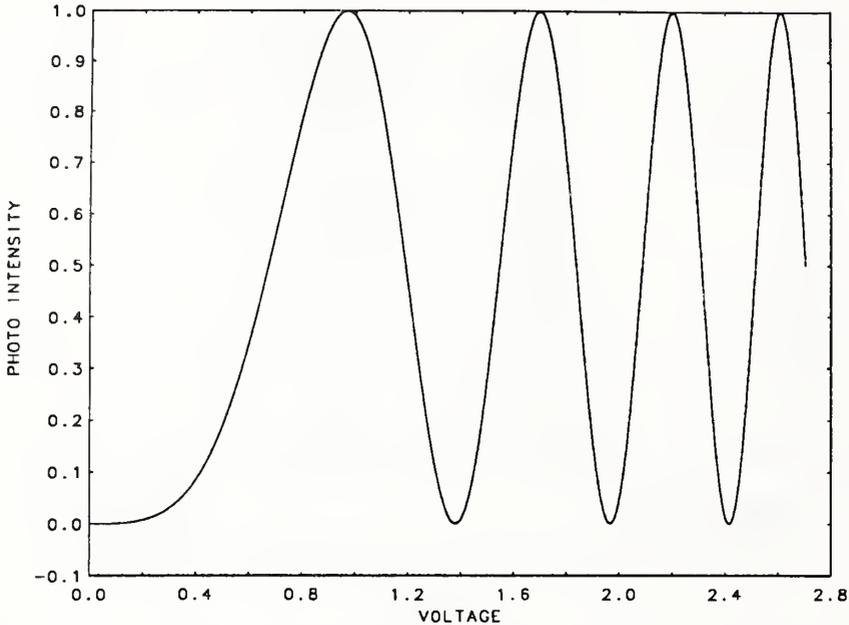
Figure 3. The ideal Kerr-law voltage-intensity ( $U$  vs.  $L$ ) relationship with a voltage peak chosen to generate 7.5 fringes. Time is absent from this plot and from the fitting procedure. The fitting minimizes the total residual between the measured voltage-intensity data and the  $U$  vs.  $L$  ‘curve’.
