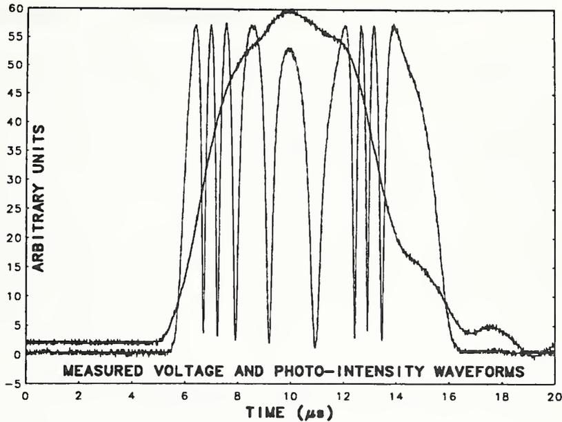
**Figure 2.** The traces of the voltage and Kerr optical waveforms are displayed simultaneously for an overdriven detector. The general fringe pattern is entirely characteristic of Kerr-cell measurements. The applied voltage waveform has a single maximum.
