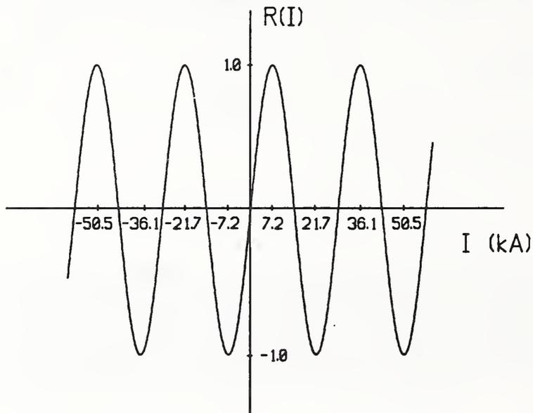
Figure 7. Response function for the dual photodetector configuration.
