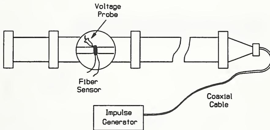
**Figure 10.** Test circuit configuration. The Marx-type impulse generator launches the fast-risetime pulses into the  $50\ \Omega$  coaxial line. The current and voltage sensors measure the pulse at the same point in the line.
