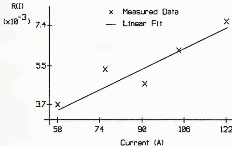
**Figure 13.** Measured dependence of the response function,  $R(I)$ , on peak current. The solid line is a linear fit to the measured peak values.
