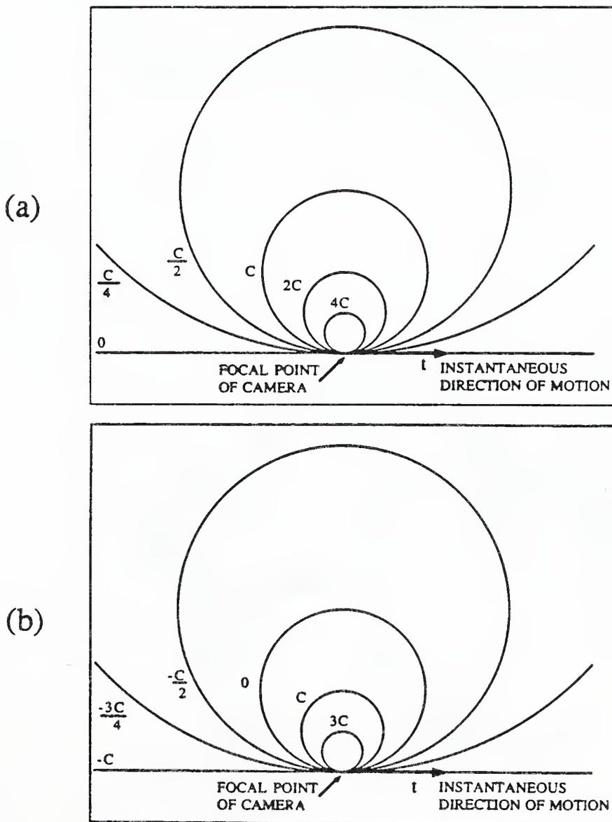
Figure 5: Optical flow values due to camera motion
