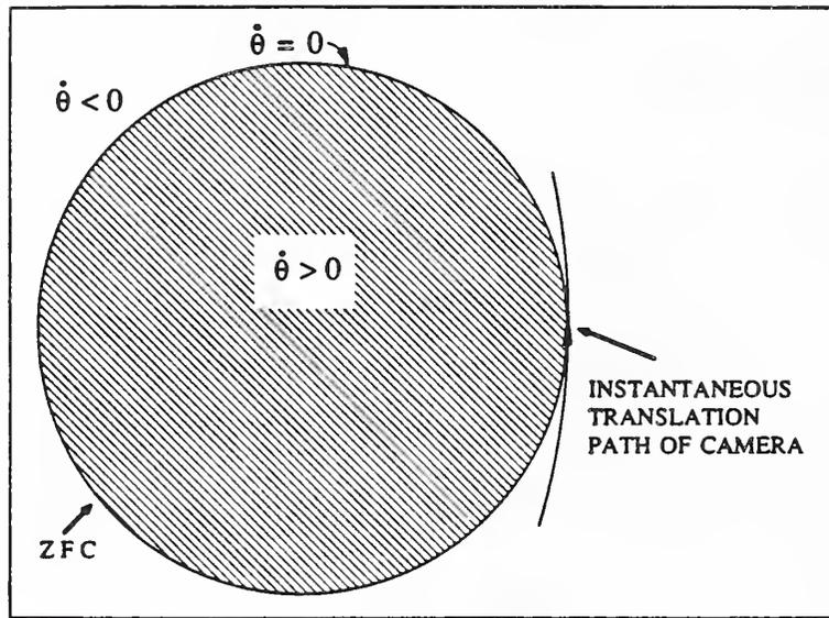
Figure 6: Optical flow signs inside and outside the ZFC
