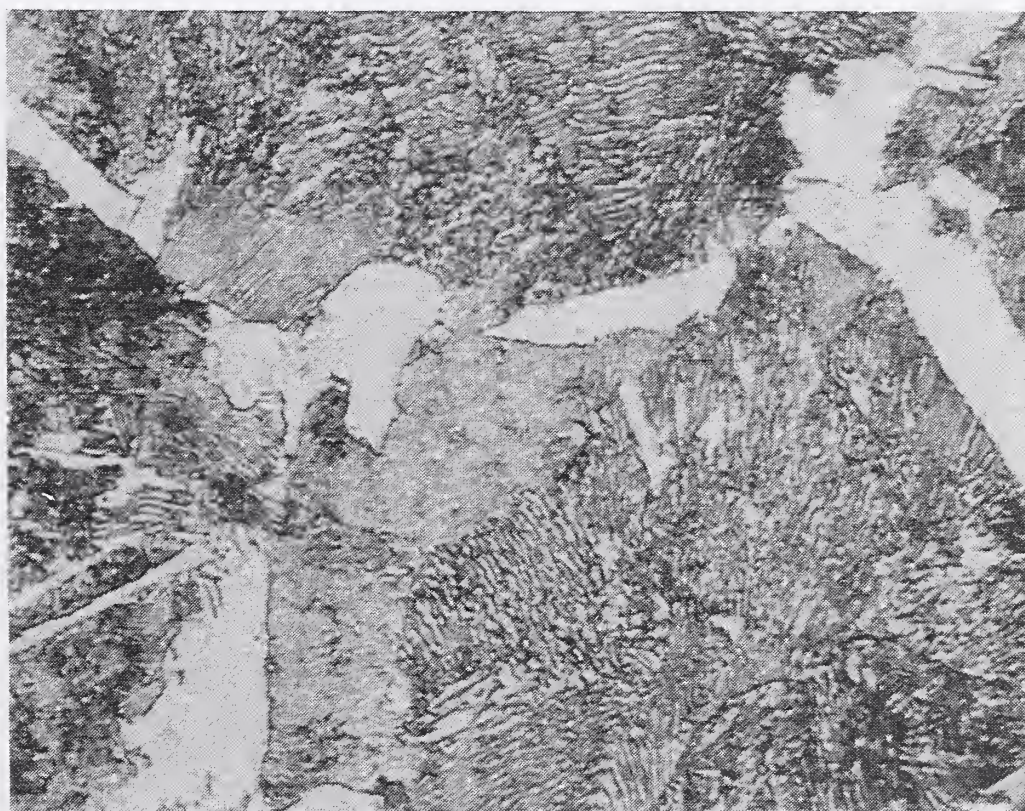
Fig. 29. Microstructure of SAE 1141-Nb steel after deformation at 1100°C and air-cooling (a) low magnification, (b) low magnification.
