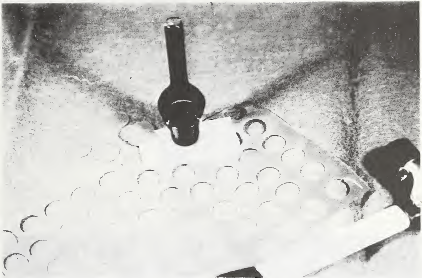
Figure 2. A single layer of PPMI film was sandwiched between paper and cut with a circular gasket cutter. Use of a backing sheet of PTFE prolonged the life of the cutting edge.
