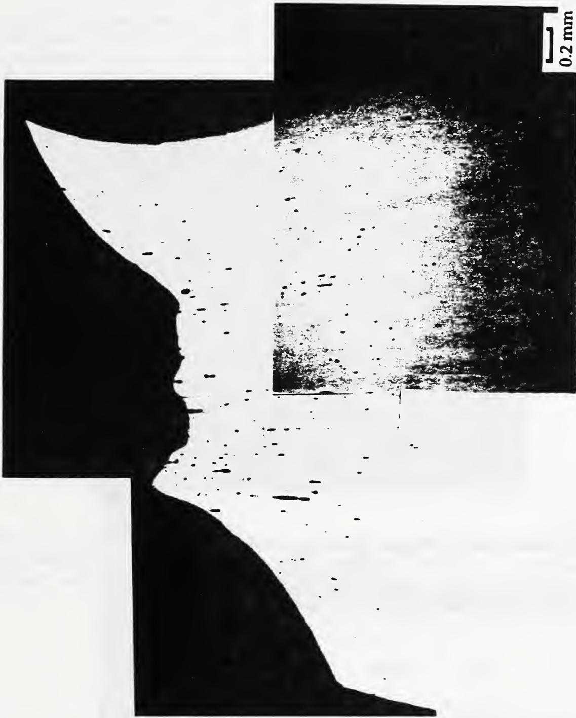
Figure 28. Cross section, unetched, through transverse uniaxial tension specimen broken at 295 K.
