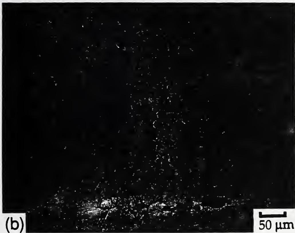
Figure 42. The cross section through compact specimen AA-2 tested at 295 K. Crack growth direction is left to right.
