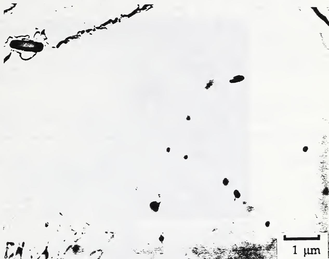
Figure 14. Representative TEM micrograph shows the distribution of submicrometer particles in the processed plate after annealing history.
