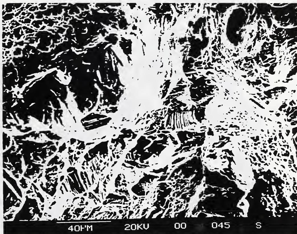
Figure 9. SEM fractographs of Charpy specimens: Fe-18Cr-3Ni-13Mn steel tested at 4 K (upper, 500X) and at 77 K (lower, 500X).
