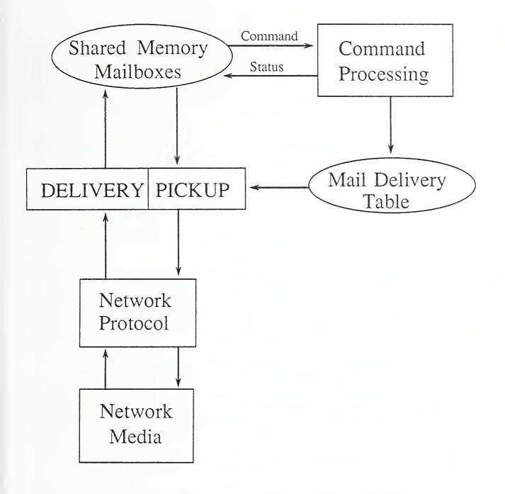
Figure 11-7. The Anatomy of the Network Interface Process (NIP)
