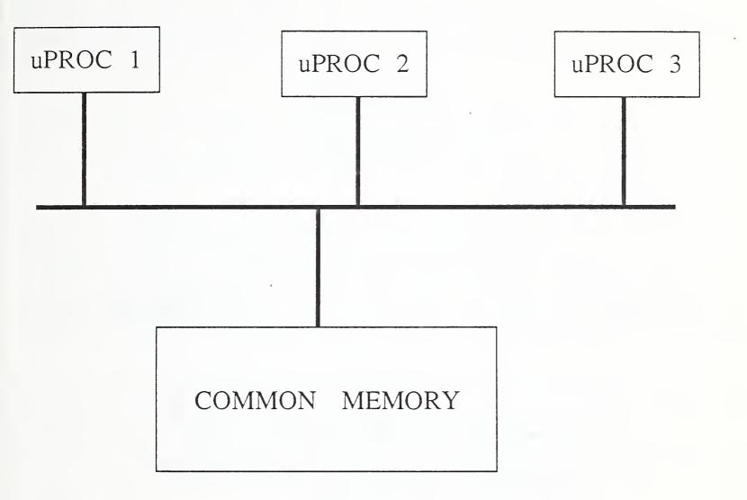
Figure 11-1. Multiple-Processor Structure with a Physical Common Memory.
