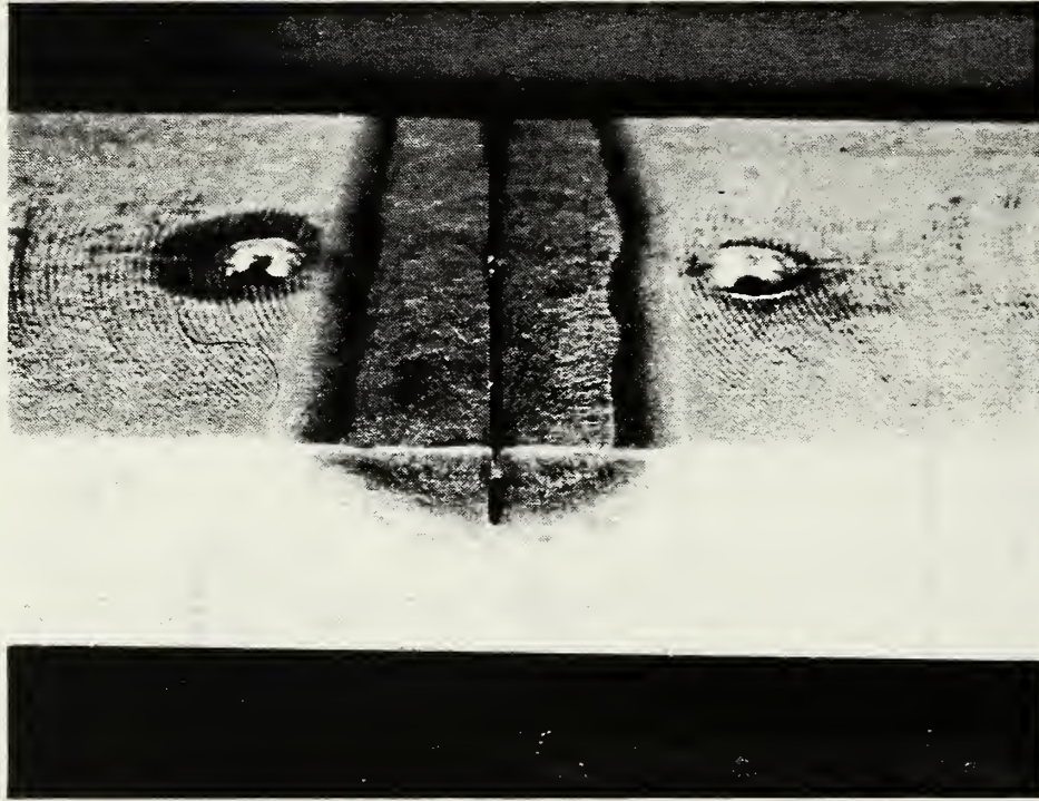
Figure 7.12a - Embrittlement Zone at Notch Tip in Single-Edge Notch Bend Test
