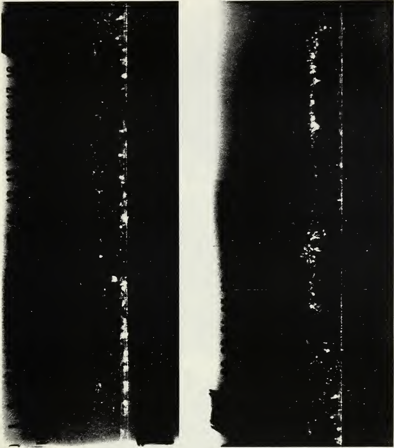
Figure 7.15 - X-ray Radiograph of Horizontal Weld after Surface Grinding
