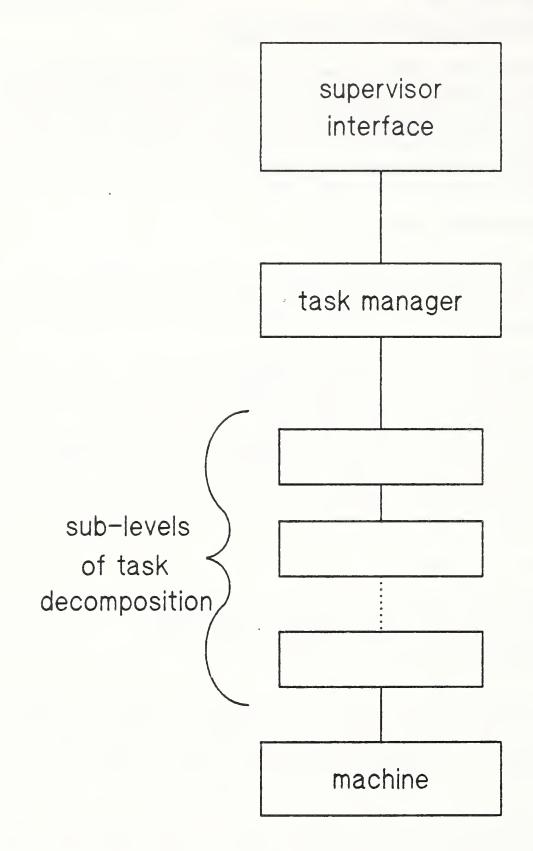
Figure 1. Control levels for the IWS Generic Controller
