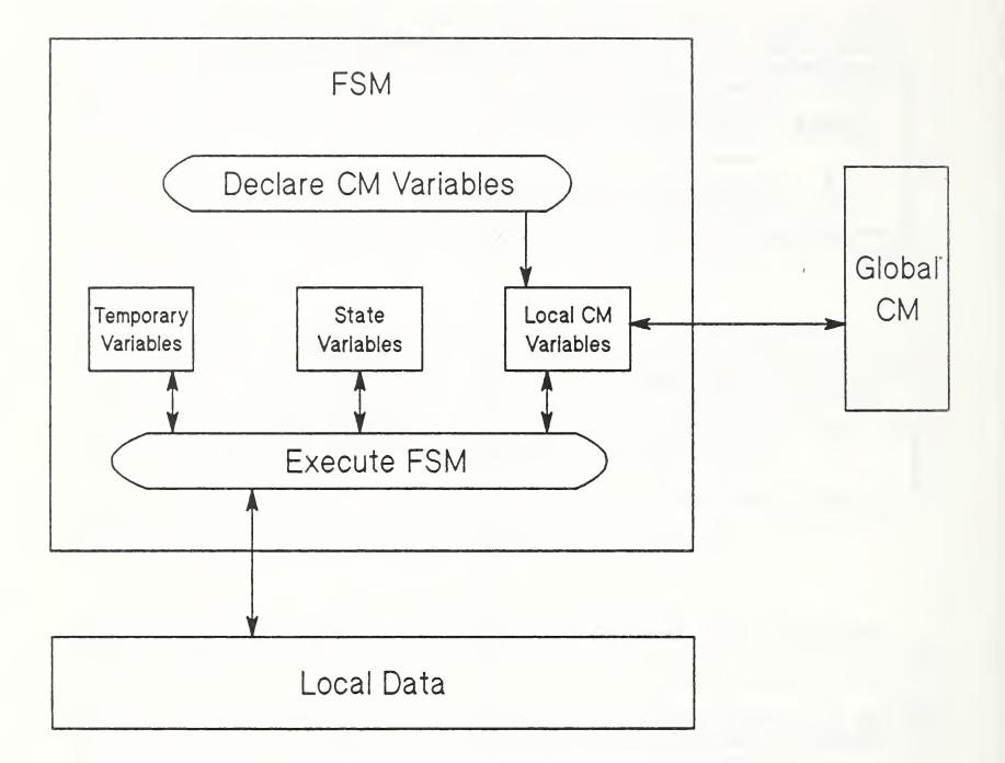
Figure 4. Software Components of FSM
