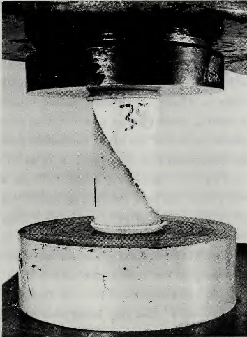
Figure 3. Slant shear specimen being compressed. One half of the specimen is base portland cement concrete and the other half is repair material.
