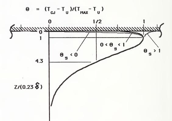
Figure 4. Plots of dimensionless ceiling jet temperature distribution,  $\theta$ , as a function of  $z/(0.23\delta)$  per Eq. (52) for cases when  $\theta_s$ is < 0, between 0 and 1, and > 0
