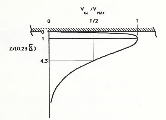
Figure 3. A plot of dimensionless ceiling jet velocity distribution,  $V_{CJ}/V_{MAX}$ , as a function of  $z/(0.23\delta)$  per Eq. (49)
