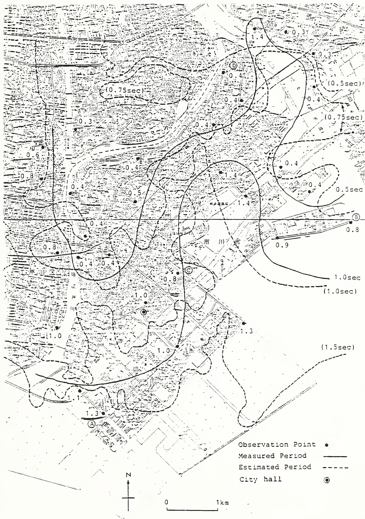
Fig.5 Predominant period of surface layer and observation points of microtremors (eastern neighbor of Tokyo)
