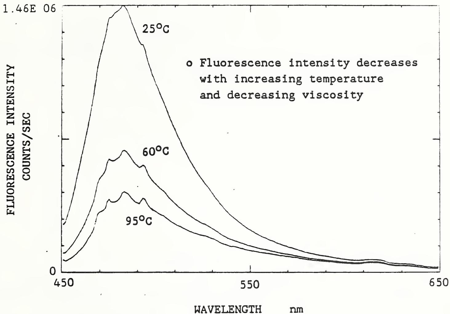
Figure 8. The fluorescence spectra of a doped polymer binder, BAMO/NMMO, are shown for 25, 60, and 95°C. The chromophore was p-dimethylaminobenzylidene malononitrile.
