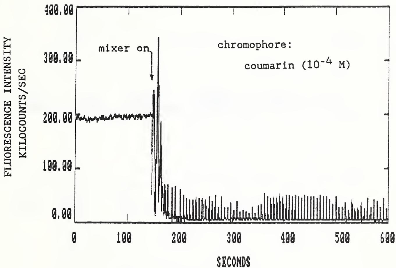
Figure 4. Fluorescence intensity versus time is plotted for mixing of coumarin 30 doped PBAN with 58% aluminum oxide by weight. Grain size of the aluminum oxide was 14 μm.
