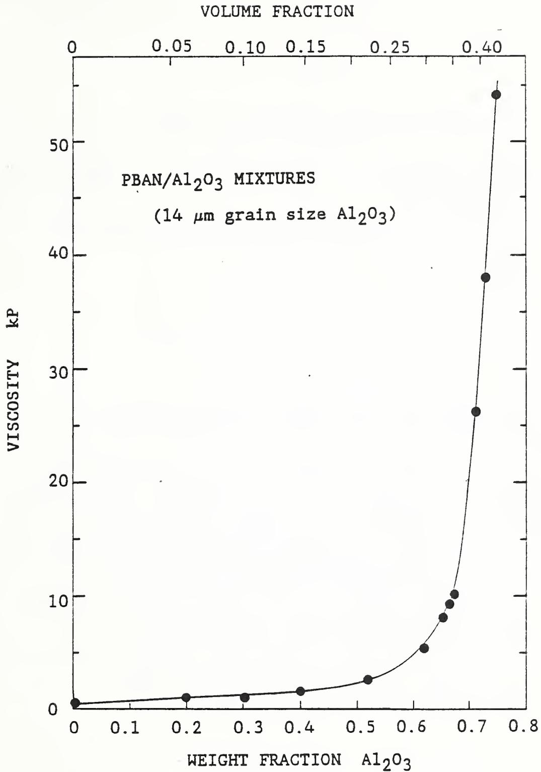
Figure 10. Viscosity vs concentration for aluminum oxide filled PBAN is shown. The measurements are reported for a shear rate of  $0.55 \text{ s}^{-1}$ .
