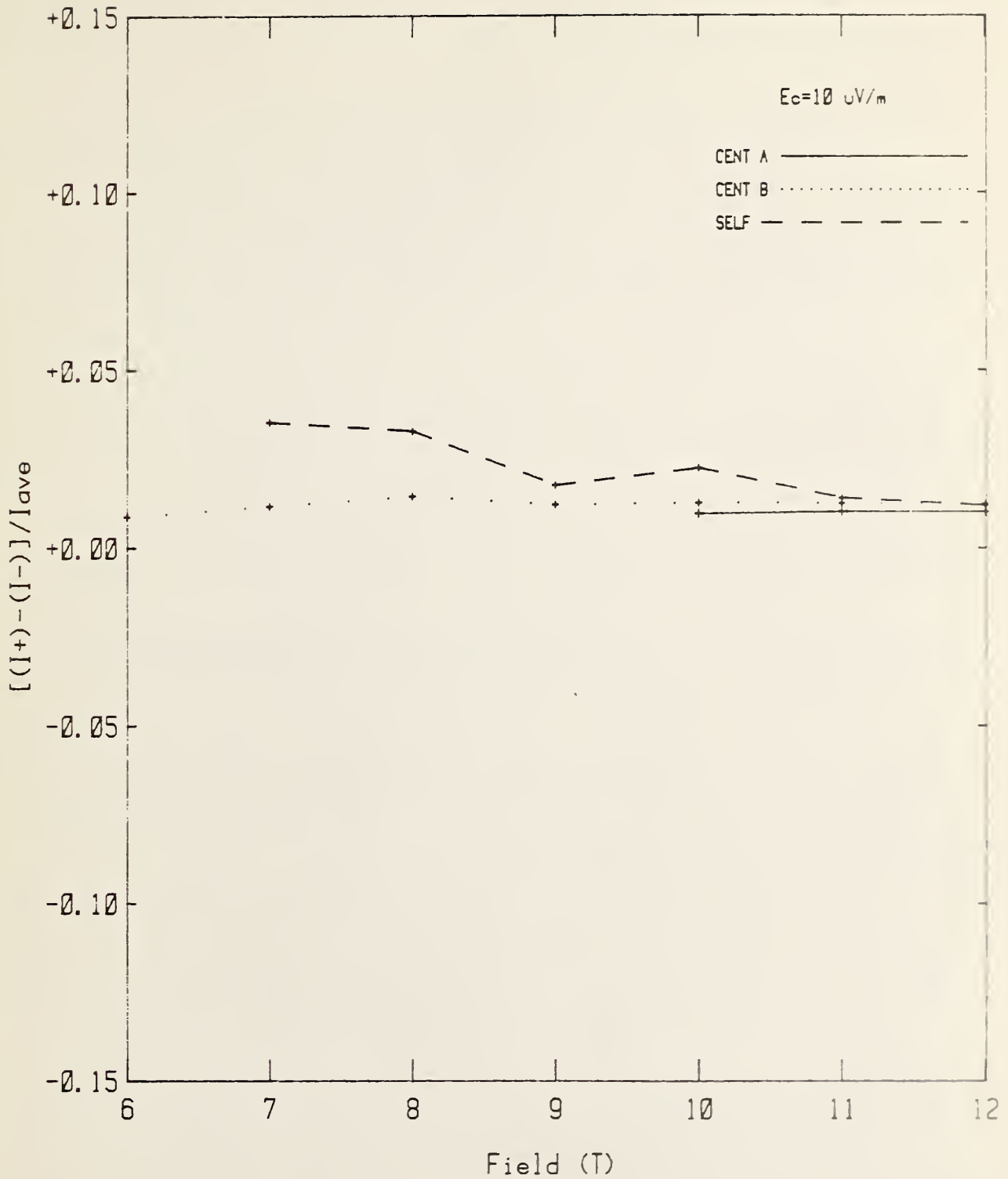
Fig. 12. Percentage difference between I_c measured with reverse and forward current directions versus magnetic field for specimens of sample Z.
