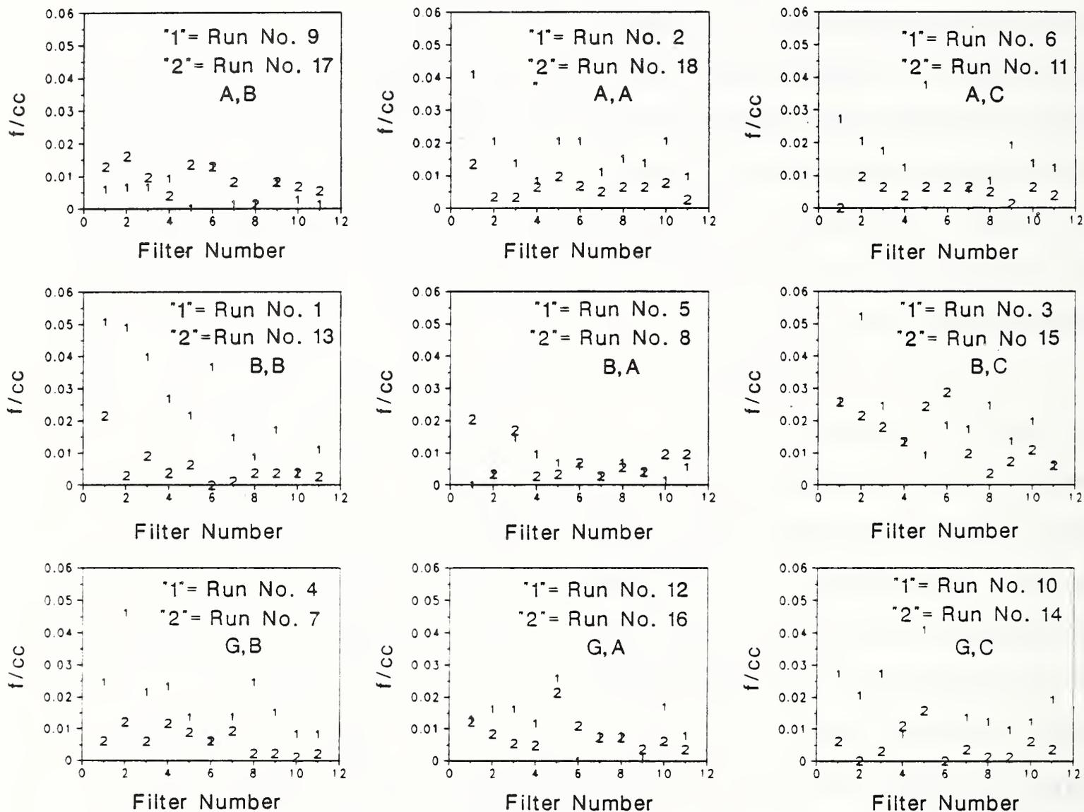
Figure 7. The first and second replicates, denoted by "1" and "2" respectively, are plotted for each of the 11 filter numbers. Each of the nine plots corresponds to a different mechanical anchoring device-encapsulant combination. For each plot, the type of mechanical anchoring device is designated by the first letter and the encapsulant type is designated by the second letter (see table 8).
