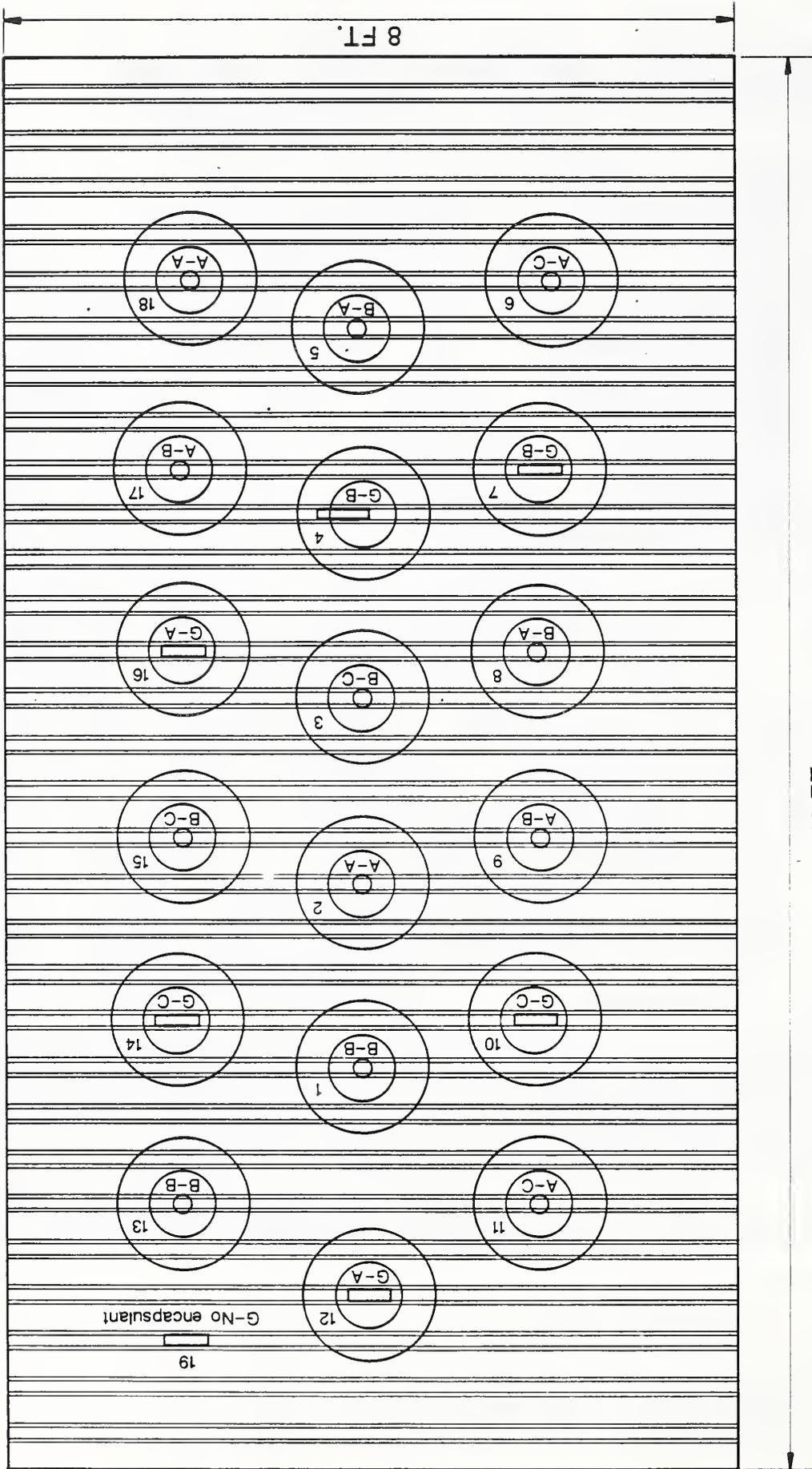
Figure 3. Sketch of the position and order of testing for each test run. Areas of encapsulation and coring are shown with respect to the position of the flutes. At each test location, the test run number is shown. The type of mechanical anchoring device is designated by the first letter, and the encapsulant type is designated by the cond letter (table 8).
