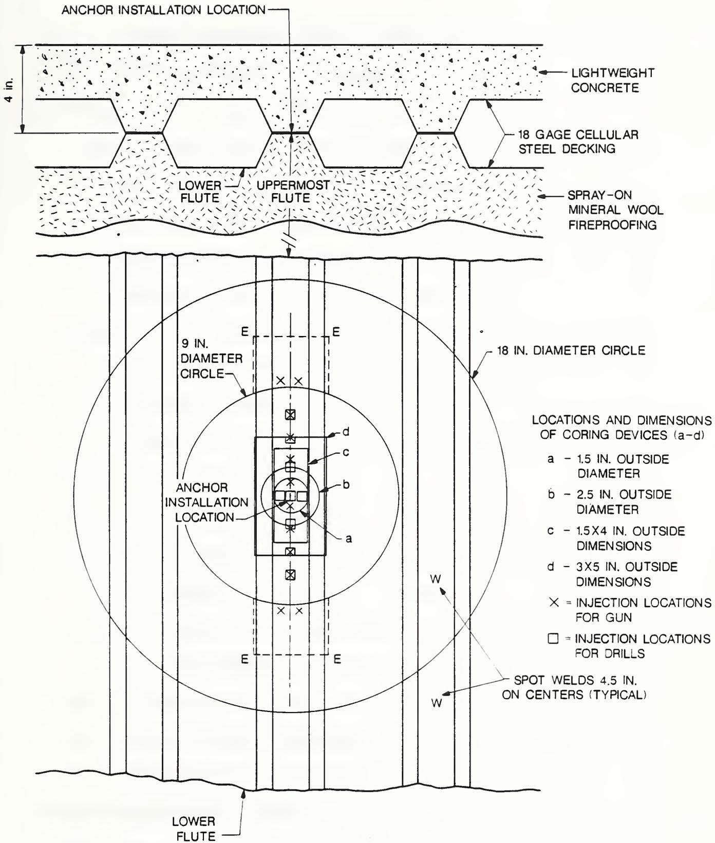
Figure 1. Sketch of typical test area of cellular steel deck/concrete floor slab and spray-on mineral wool. Locations of anchor installation, encapsulation, injection, and coring are shown. The "E" lines represent extended areas of encapsulation (Section 3.5).
