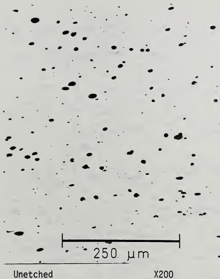
Figure 3. Photomicrograph of AISI 12L14 Steel Base Metal
