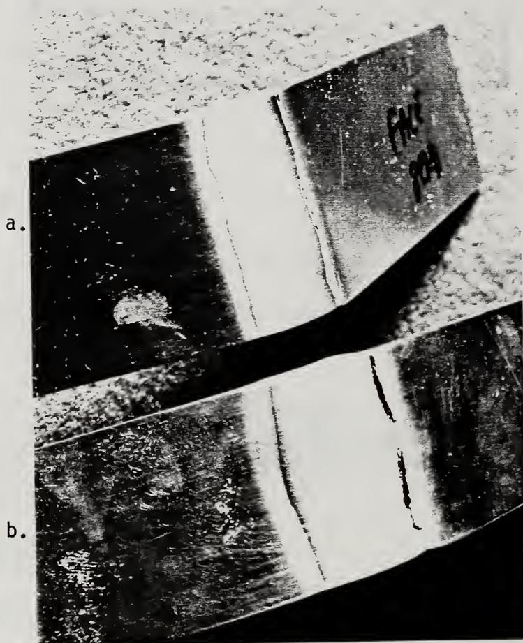
Figure 2. Guided Bend Roller Test Specimens
