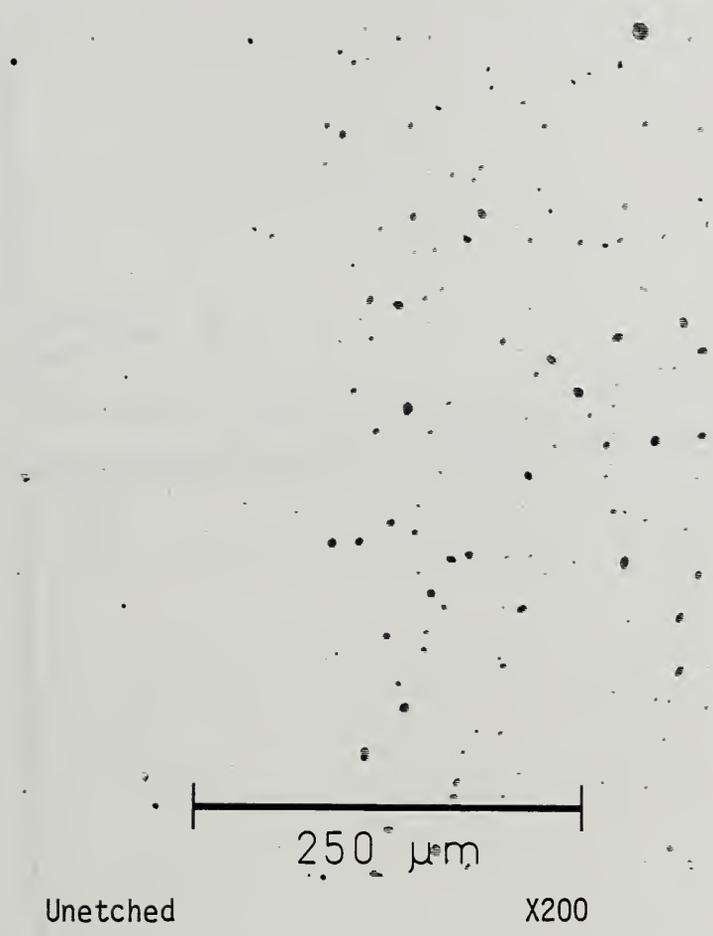
Figure 5. Photomicrograph of AISI 12L14 Steel Weld Metal/HAZ Interface
