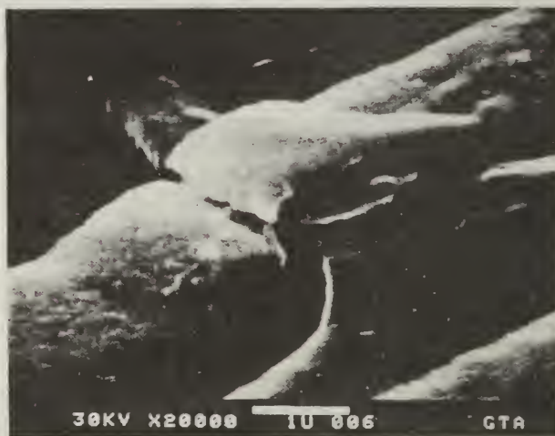
Figure 1. Vendor A failing word line showing crack in refractory metal silicide line and interlevel oxide. SEM micrograph, 20,000x.
