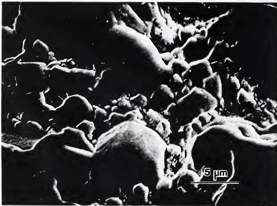
3. Scanning electron micrograph of one of the dark regions shown in figure 2. X-ray energy dispersive spectroscopy indicates these submicron grains to consist largely of \text{MgCr}_2\text{O}_4 . Traces of calcium, aluminum and silicon are also observed in these areas.
