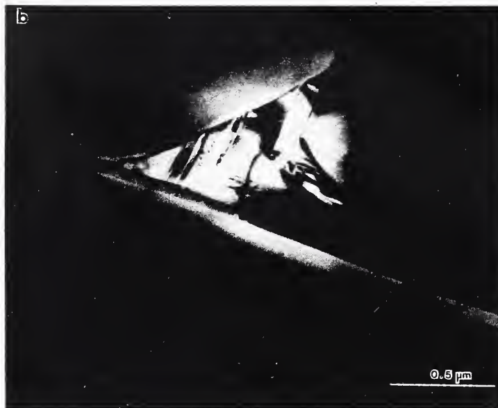
1. Intergranular phase in vitreous bonded aluminum oxide (AD-96): (a) In the as-received material, the bonding phase is amorphous consisting of an aluminosilicate glass which also contains calcium, magnesium and potassium as network modifiers; (b) After heating at 1050°C for 96 hours, the bonding phase crystallizes into a number of silicate minerals (see reference 2 for details of the composition and crystal structure of this material).
