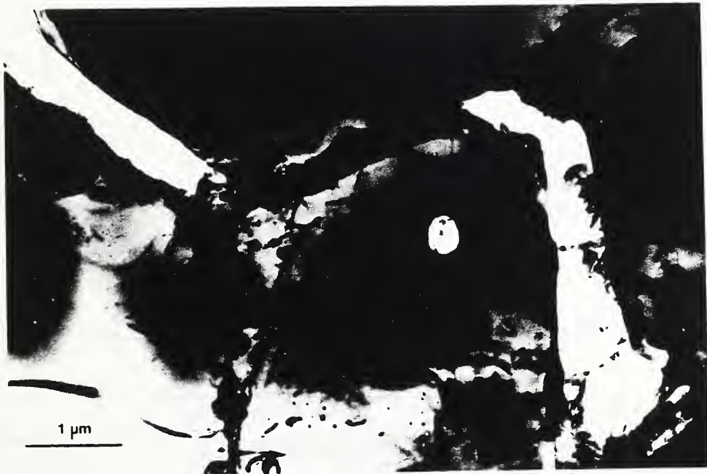
6. Unbroken ligament joining the surfaces of a creep crack. The dislocations in the aluminum oxide grains are a consequence of surface polishing and do not result from the process of creep. Specimens taken from locations that lie further from the surface show no evidence of dislocations within the alumina grains, see figure 2 for example. This transmission electron micrograph shows the ligament separation occurring by shear deformation.
