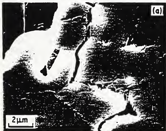
Figure 6 (a) SEM illustrating cavitation at grain boundaries and triple junctions in vicinity of developing creep crack on tensile surface. (b) TEM showing plate-like cavities at inclined grain boundary after creep deformation. Formation and growth of such cavities is considered responsible for intergranular creep crack extension.
