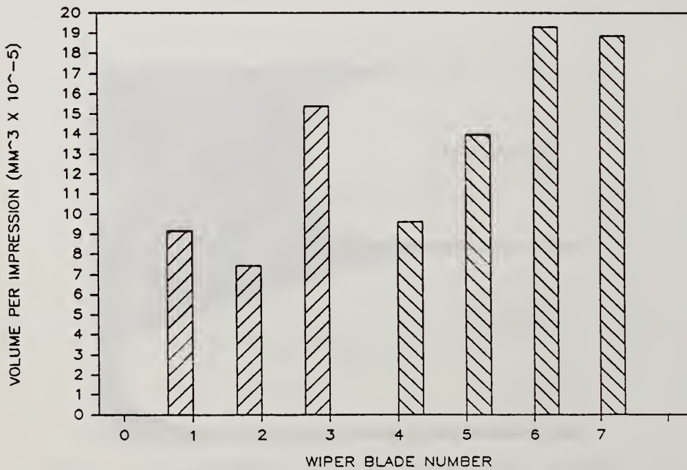
Figure 7. Wear volume as a function of number of impressions for seven different wiper blades.
