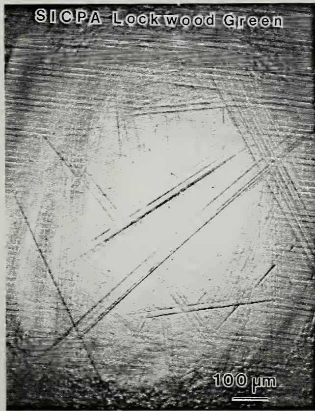
Figure 31. Photographs of wear scars on chromium plated pins after test runs with three intaglio stamp inks. Note differences in scratching produced by each ink.
