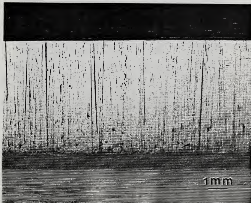
Figure 4. Photograph of the worn surface of a wiper blades showing abrasive wear scratches.
