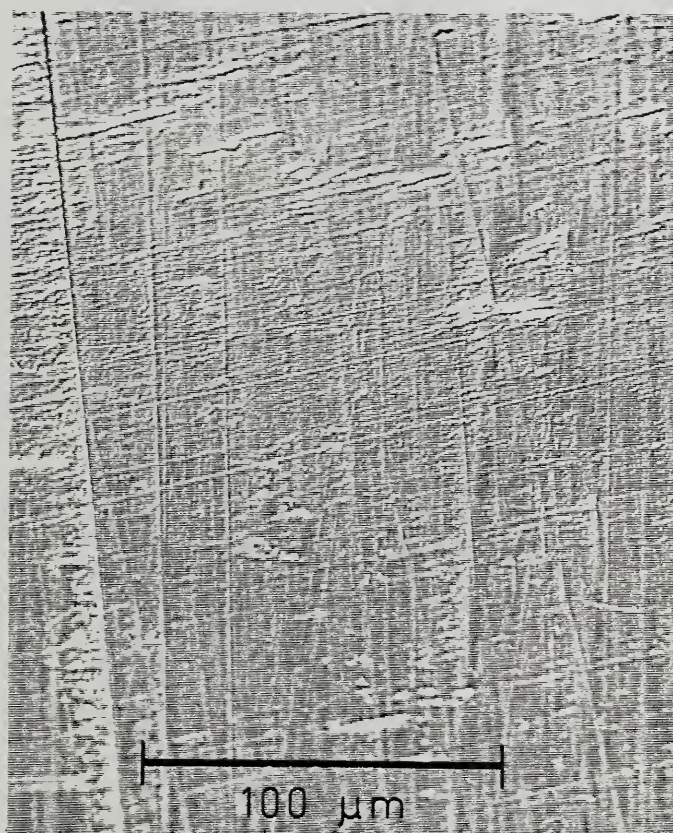
Figure 16. Photograph of chromium plated surface showing transfer of amorphous silica particles.
