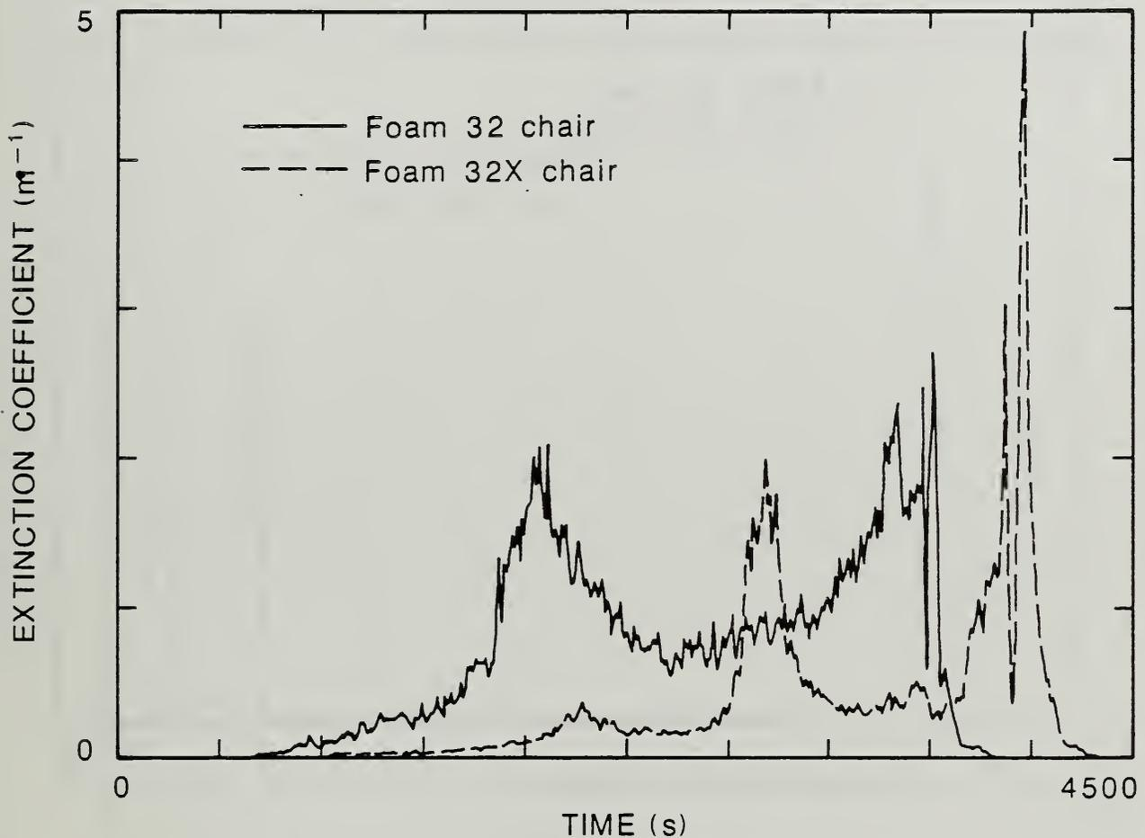
Figure 37. Comparison of the Smoke Extinction Coefficient for the Smoldering-to-Flaming Ignitions of Foams 32 and 32X Upholstery Chair Mock-ups Tested in the Furniture Calorimeter (excluding early smoldering because of erratic response).
