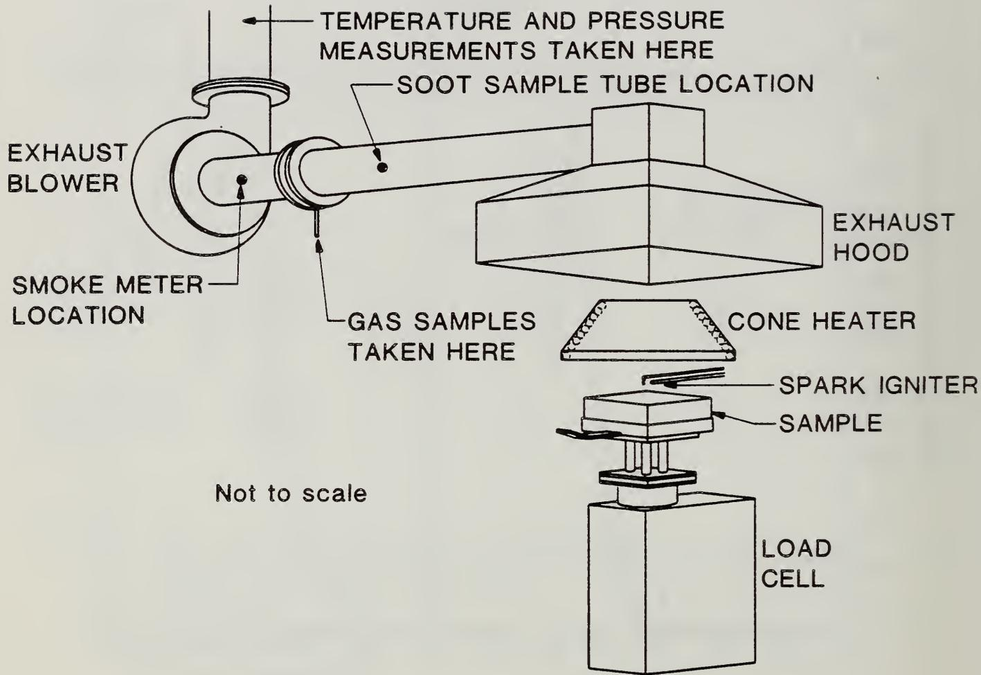
Figure 2. Schematic of the Cone Calorimeter.
