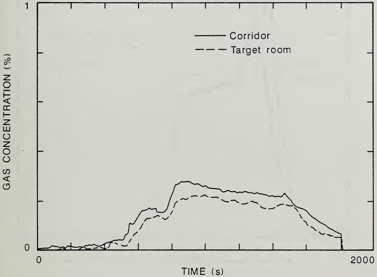
Figure 43. Carbon Monoxide Concentration in Each Compartment of the Large-Scale Facility During Flaming Ignition Test of Foam 32X Mock-up Upholstery Chair Assembly.
