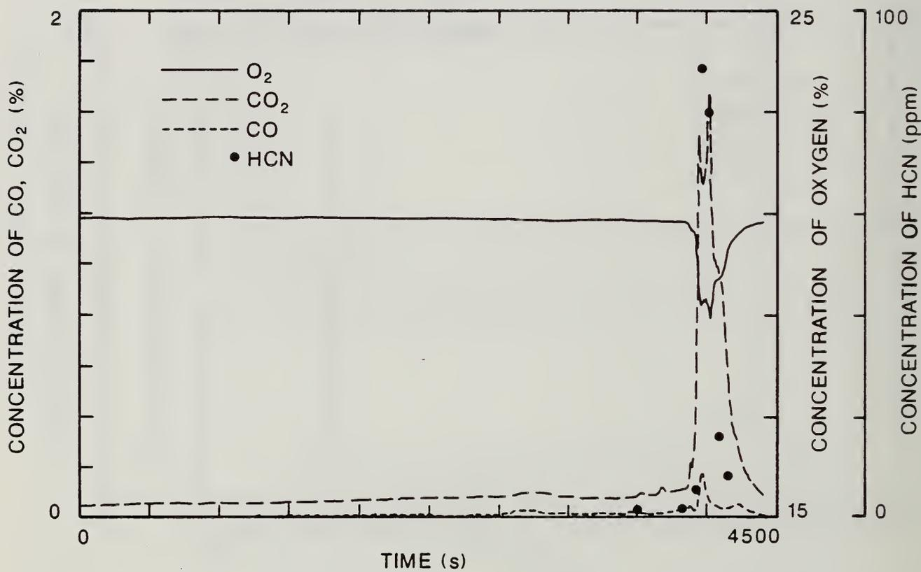
Figure 32. Concentration of CO<sub>2</sub>, CO, HCN, and Oxygen During the Smoldering-to-Flaming Ignition of Foam 32X Mock-up Upholstery Chairs Tested in the Furniture Calorimeter.
