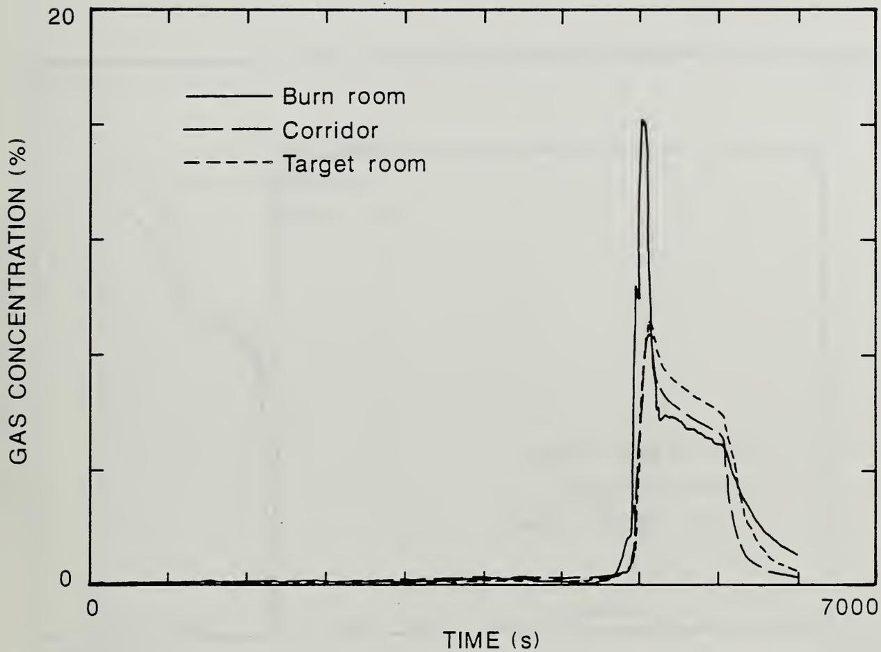
Figure 53. Comparison of Carbon Dioxide Concentrations in Each Compartment of the Large-Scale Test Facility for the One Cigarette Test of Foam 32 Mock-up Upholstery Chair Assembly.
