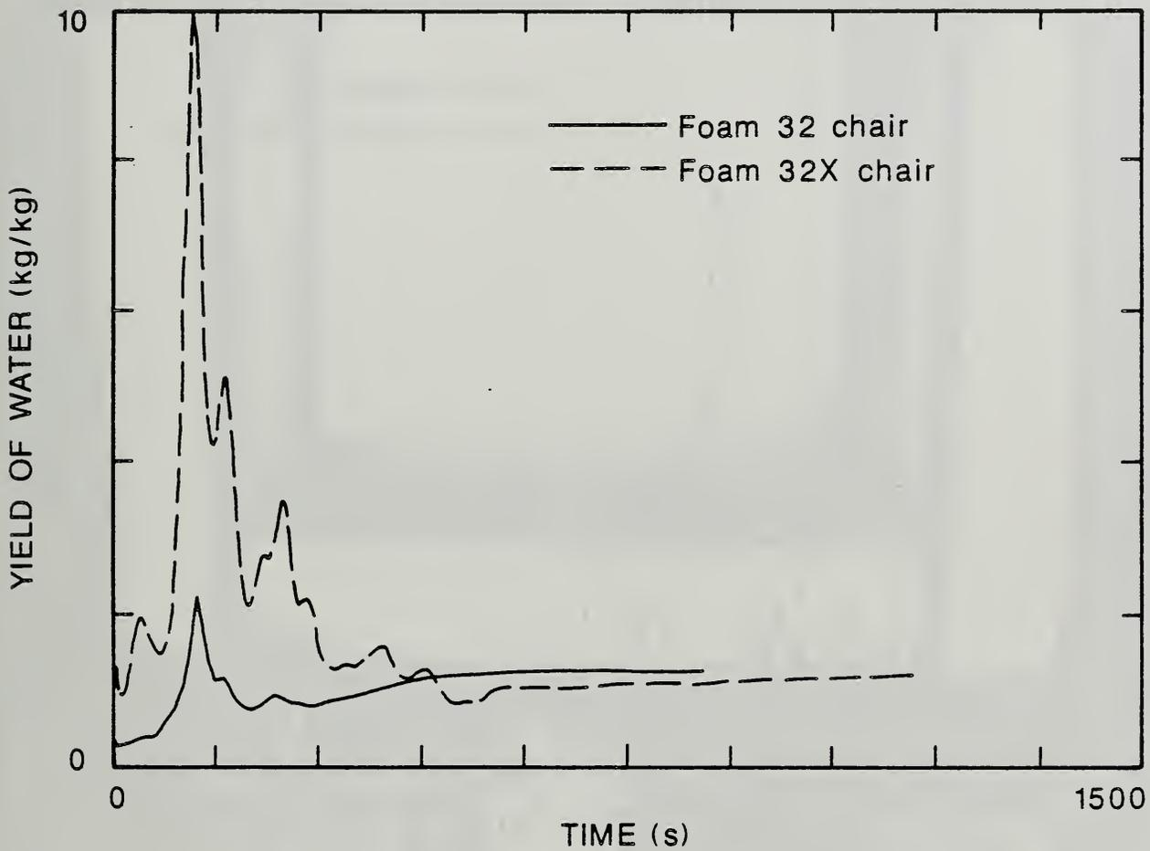
Figure 27. Comparison of the Yield of Water from the Flaming Ignition of Foams 32 and 32X During the Burning of Mock-up Upholstery Chairs in the Furniture Calorimeter.
