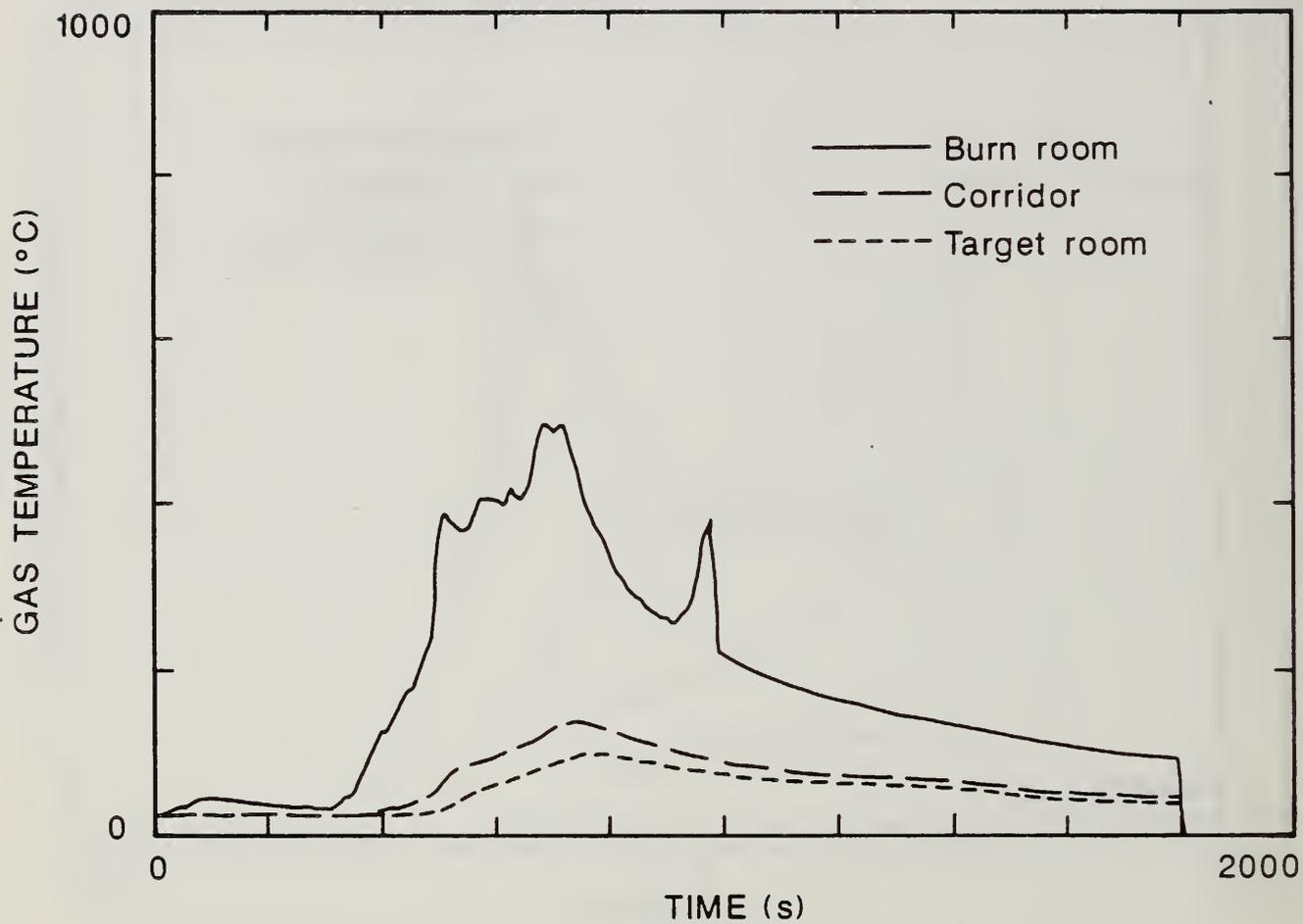
Figure 50. Upper Layer Gas Temperatures in Each Compartment of the Large-Scale Facility During Flaming Ignition Test of Foam 32X Mock-up Upholstery Chair Assembly.
