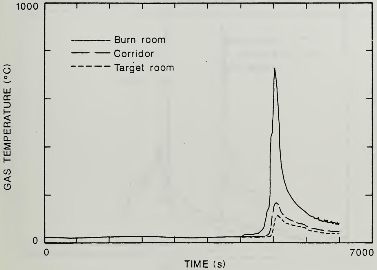
Figure 55. Comparison of Upper Compartment Gas Temperature in Each Compartment of the Large-Scale Test Facility for the One-Cigarette Test of Foam 32 Mock-up Upholstery Chair Assembly.
