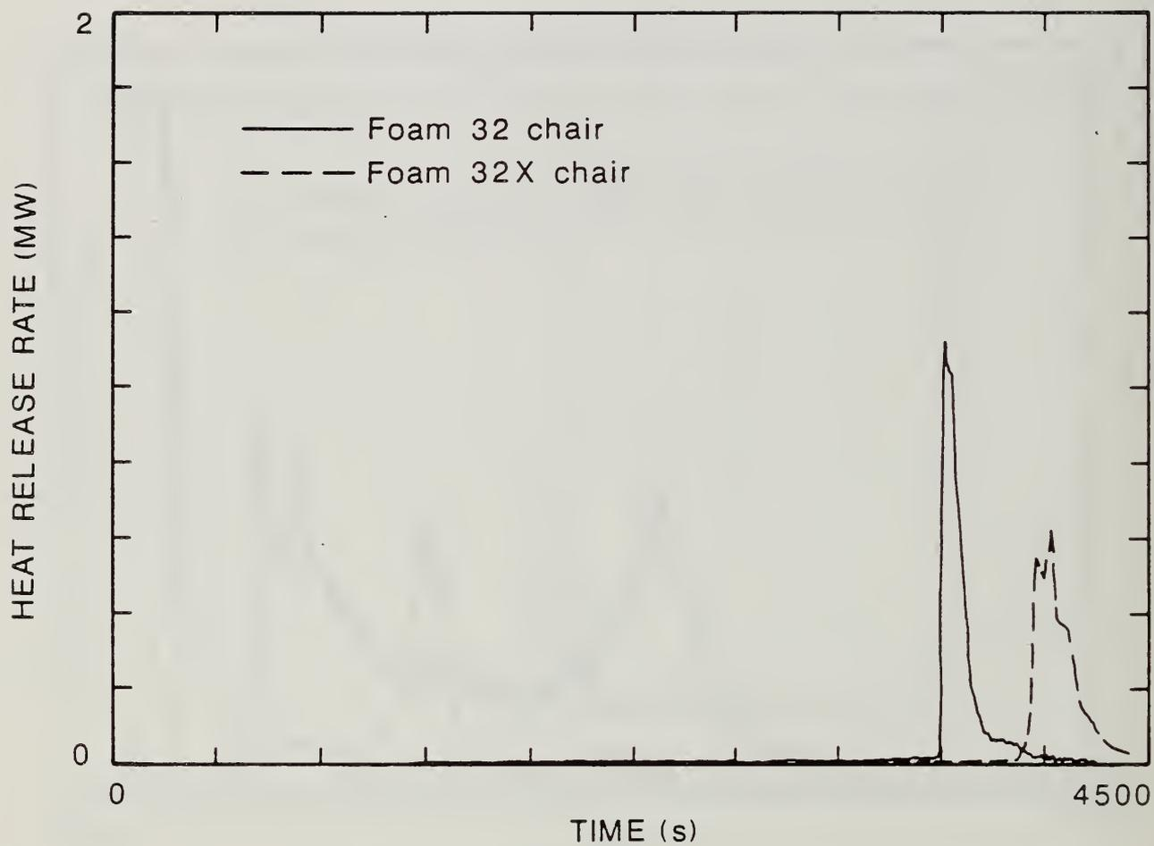
Figure 38. Comparison of the Rate of Heat Release for the Smoldering-to-Flaming Ignitions of Foams 32 and 32X Upholstery Chair Mock-ups Tested in the Furniture Calorimeter (excluding early smoldering because of erratic response).
