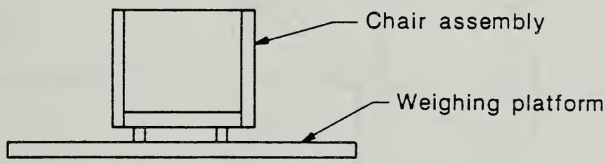
Figure 17. Schematic of Furniture Calorimeter.
