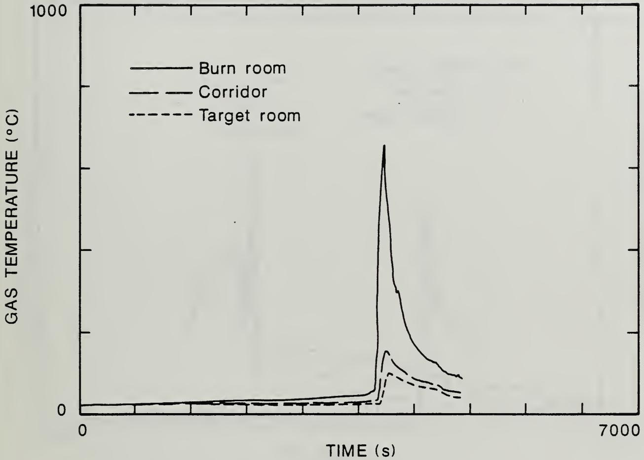
Figure 59. Comparison of Upper Compartment Gas Temperatures in Each Compartment of the Large-Scale Test Facility for the Two-Cigarette Test of Foam 32 Mock-up Upholstery Chair Assembly.
