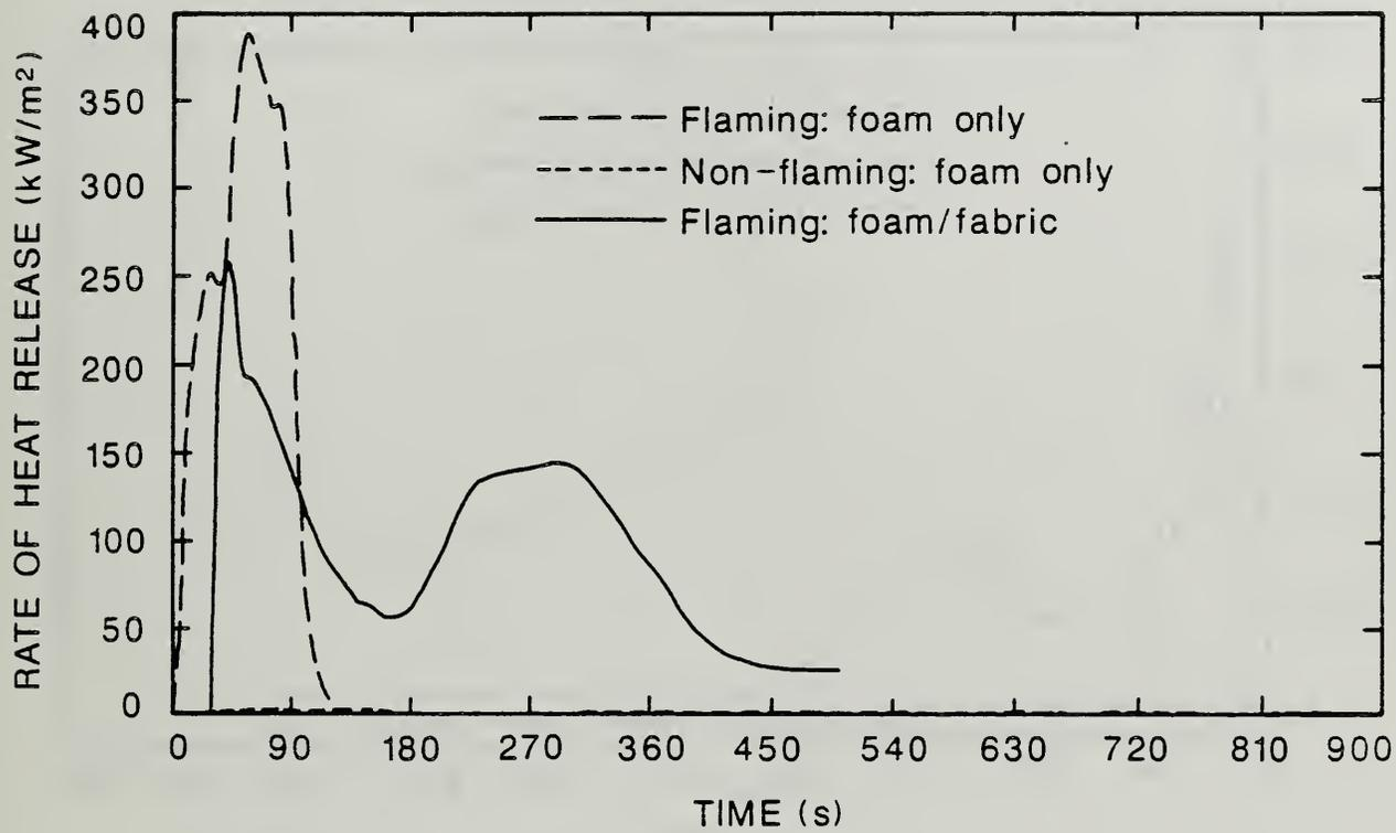
Figure 3. Comparison of Heat Release Rate for Foam 32 Flaming and Non-flaming Exposures Without a Cover Fabric and Flaming Exposure With a Cover Fabric.
