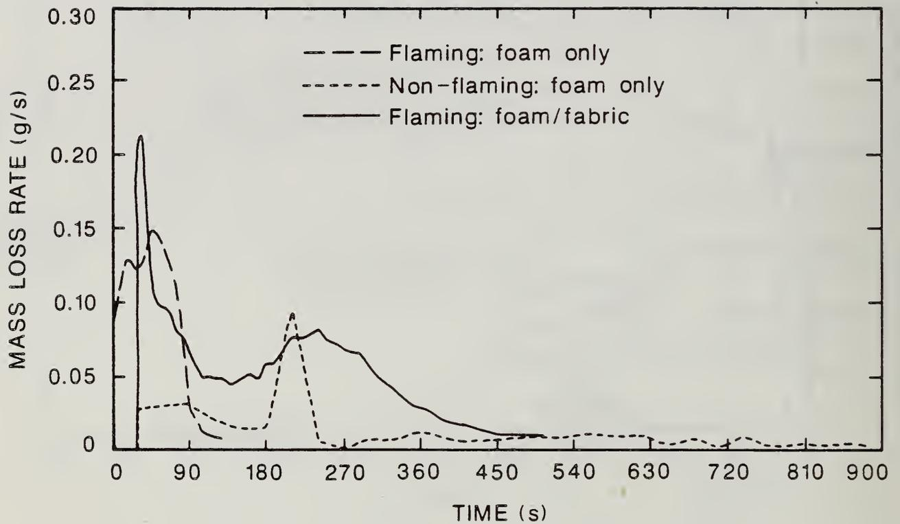
Figure 4. Comparison of Mass Loss Rate for Foam 32 Flaming and Non-flaming exposures Without a Cover Fabric and Flaming Exposures With a Cover Fabric.
