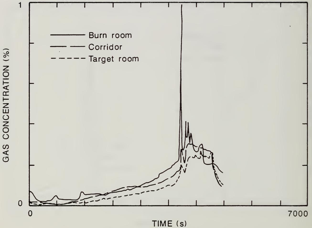
Figure 56. Comparison of Carbon Monoxide Concentrations in Each Compartment of the Large-Scale Test Facility for the Two-Cigarette Test of Foam 32 Mock-up Upholstery Chair Assembly.
