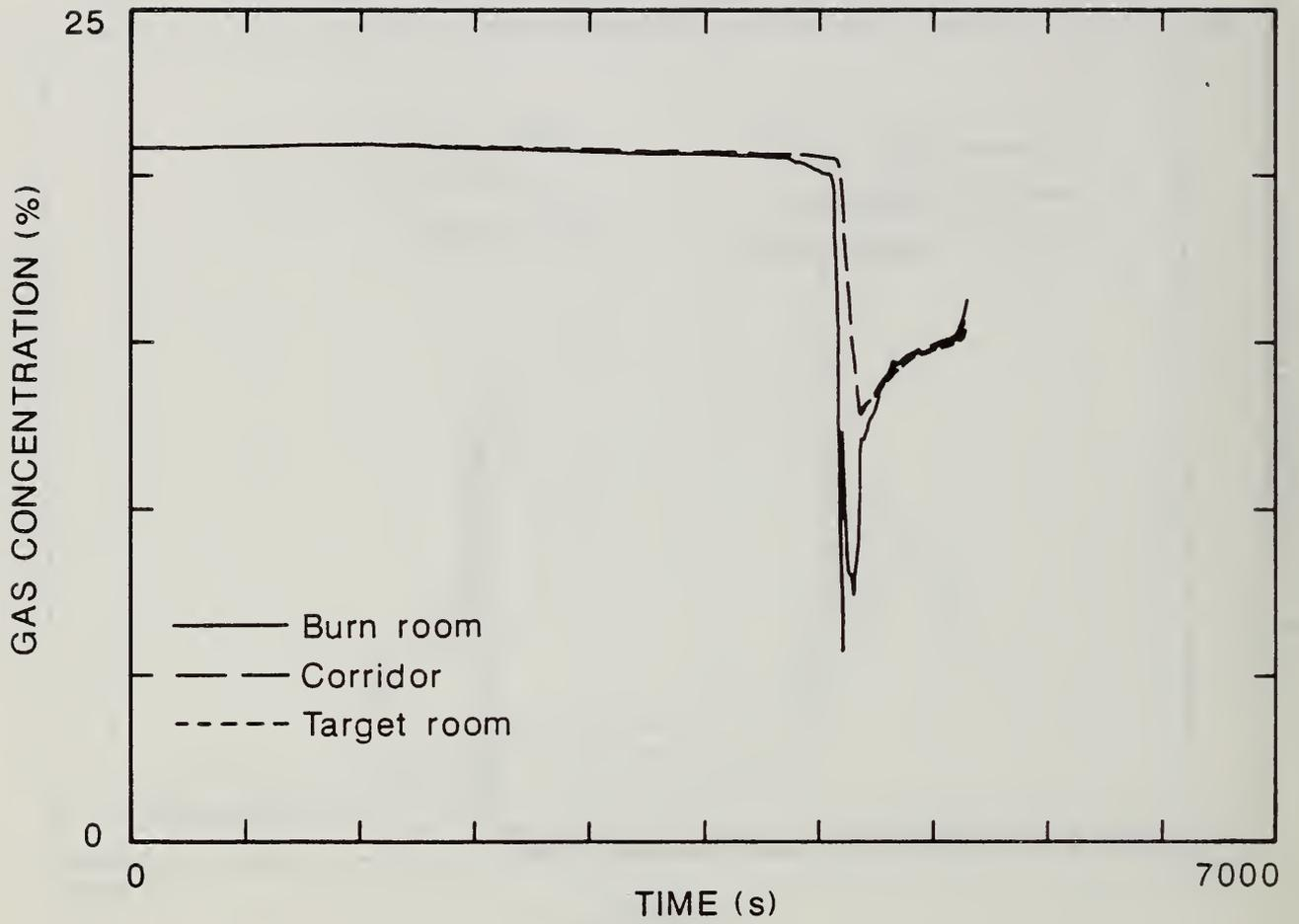
Figure 62. Comparison of Oxygen Concentrations in Each Compartment of the Large-Scale Test Facility for the Two-Cigarette Test of Foam 32X Mock-up Upholstery Chair Assembly.
