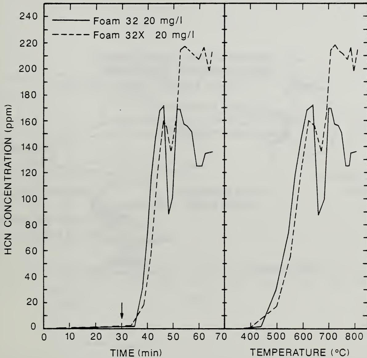
Figure 1. HCN Generation During Ramped Heating (375°C to 800°C) of Foams 32 and 32X After Preheating at 375°C for 30 Minutes in the NBS Toxicity Apparatus.
