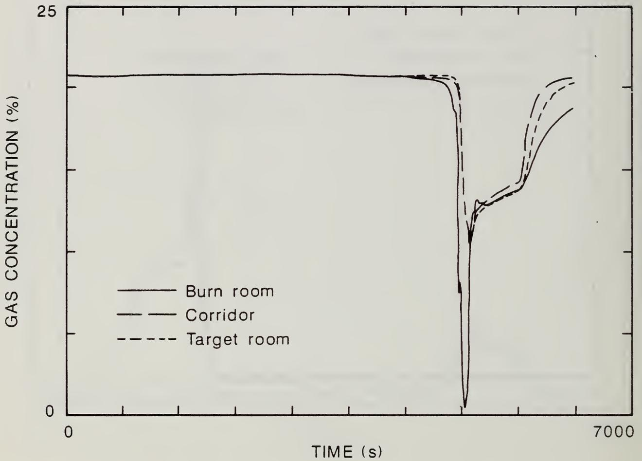
Figure 54. Comparison of Oxygen Concentrations in Each Compartment of the Large-Scale Test Facility for the One-Cigarette Test of Foam 32 Mock-up Upholstery Chair Assembly.
