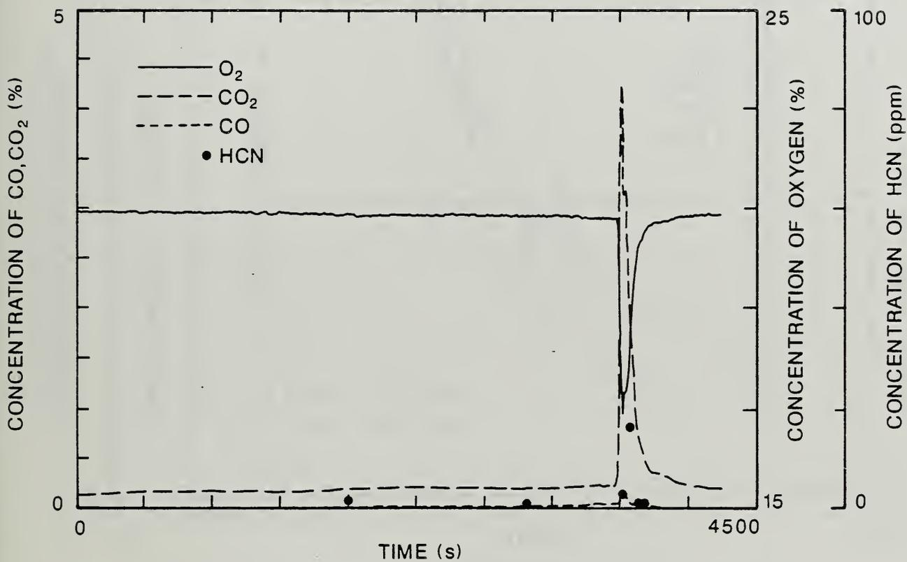
Figure 31. Concentration of CO<sub>2</sub>, CO, HCN, and Oxygen during the Smoldering-to-Flaming Ignition of Foam 32 Mock-up Upholstery Chairs Tested in the Furniture Calorimeter.
