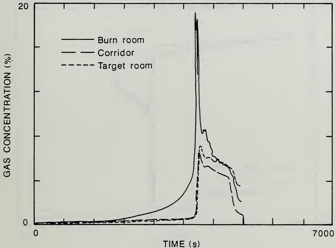
Figure 57. Comparison of Carbon Dioxide Concentration in Each Compartment of the Large-Scale Test Facility for the Two-Cigarette Test of Foam 32 Mock-up Upholstery Chair Assembly.
