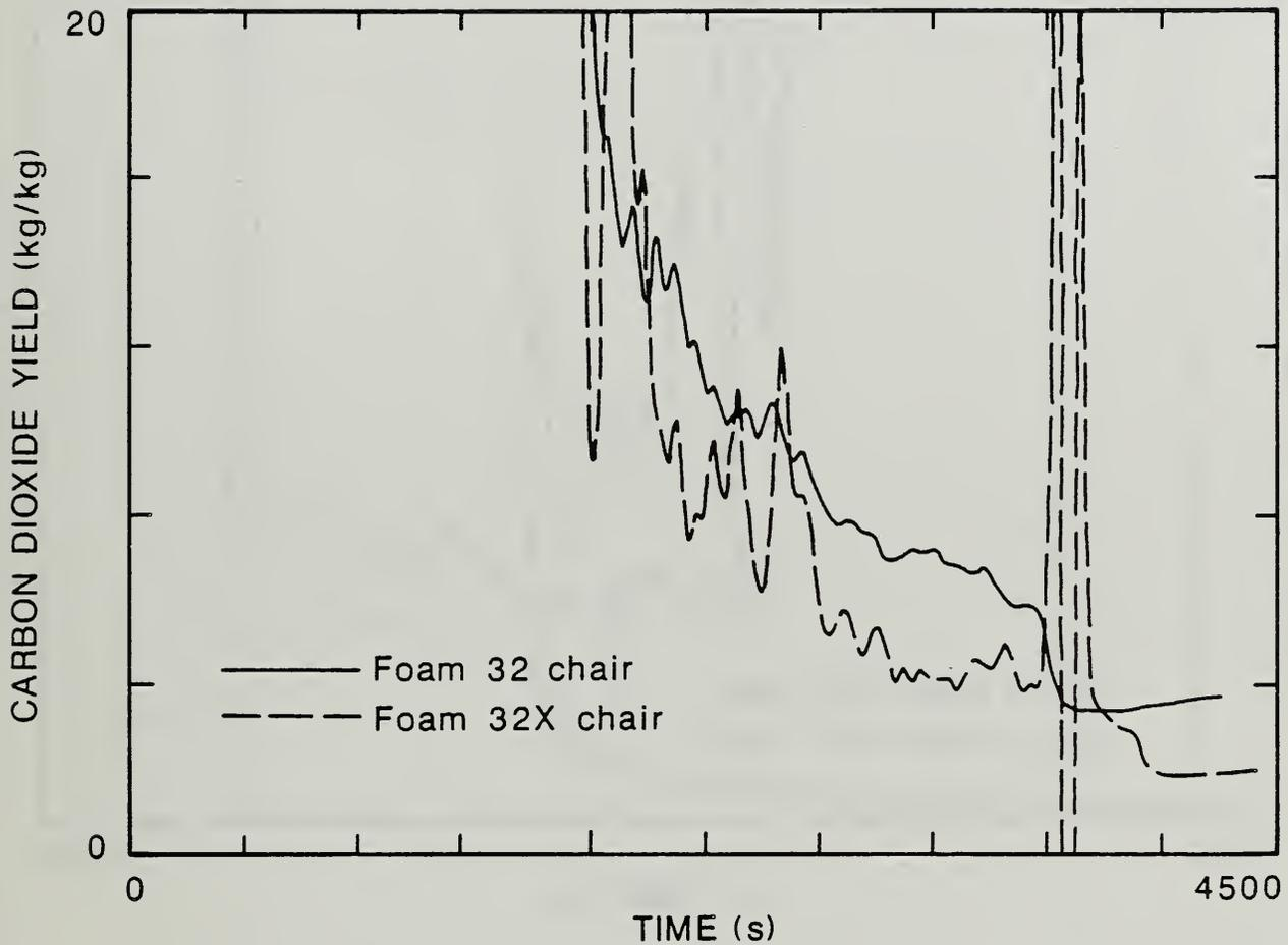
Figure 33. Comparison of Carbon Dioxide Yields for Smoldering-to-Flaming Ignitions of Foams 32 and 32X Mock-up Upholstery Chairs Tested in the Furniture Calorimeter.
