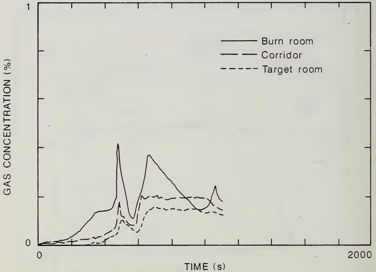
Figure 42. Carbon Monoxide Concentration in Each Compartment of the Large-Scale Facility During Flaming Ignition Test of Foam 32 Mock-up Upholstery Chair Assembly.
