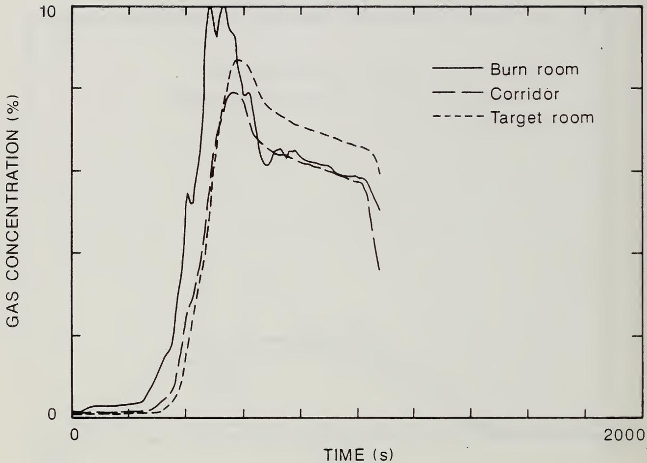
Figure 44. Carbon Dioxide Concentration in Each Compartment of The Large-Scale Facility During Flaming Ignition Test of Foam 32 Mock-up Upholstery Chair Assembly.
