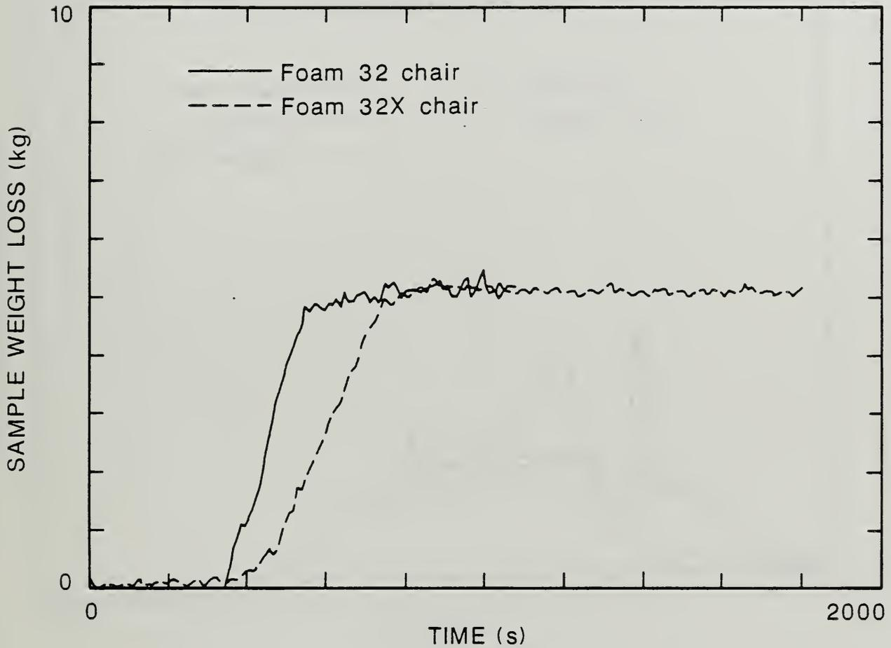
Figure 41. Comparison of Sample Weight loss for Flaming Ignition of Mock-up Upholstery Chairs made from foams 32 and 32X in the Large-Scale Three Compartment Tests.
