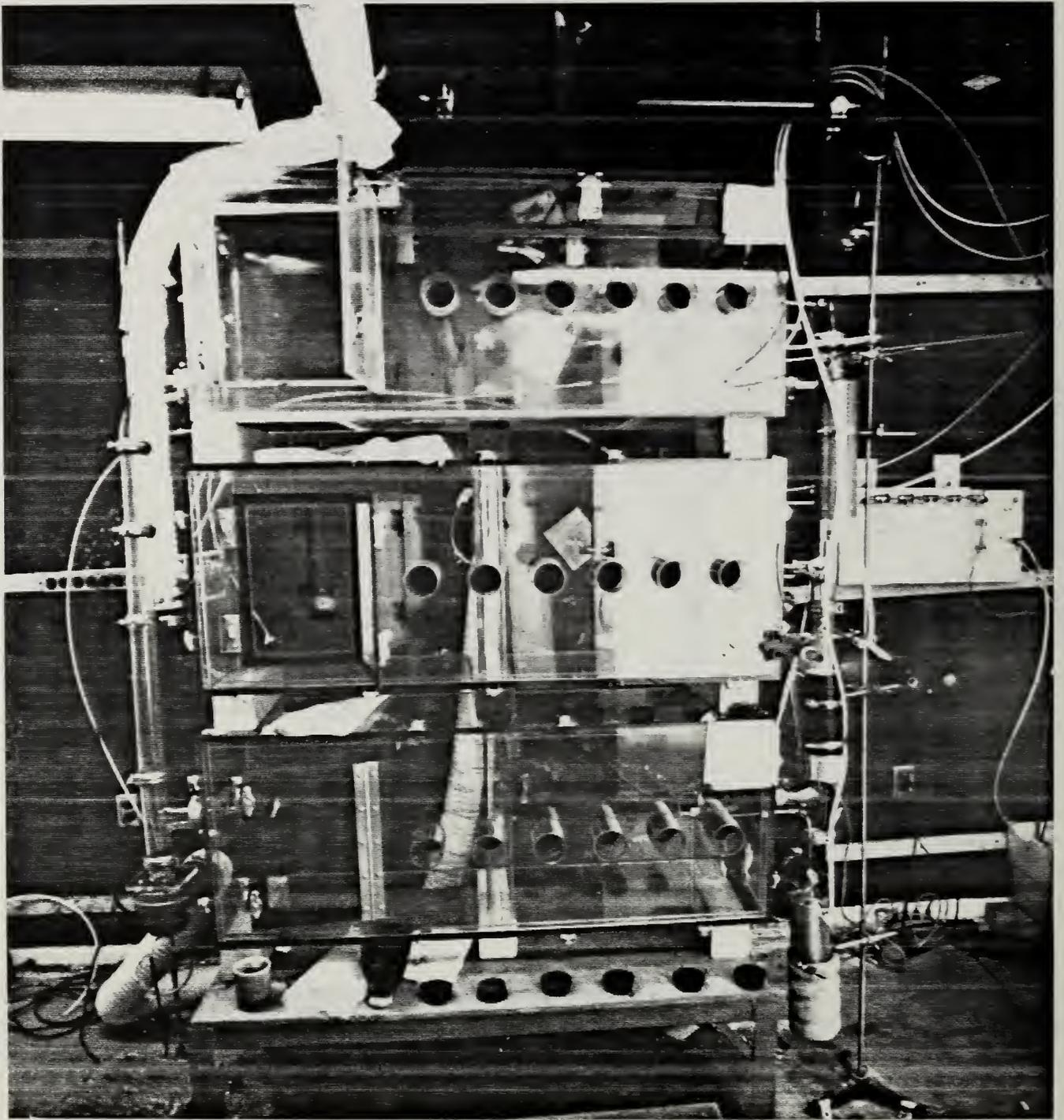
Figure 64. Large-Scale Three Compartment Animal Exposure System - Three Animal Exposure Chambers.
