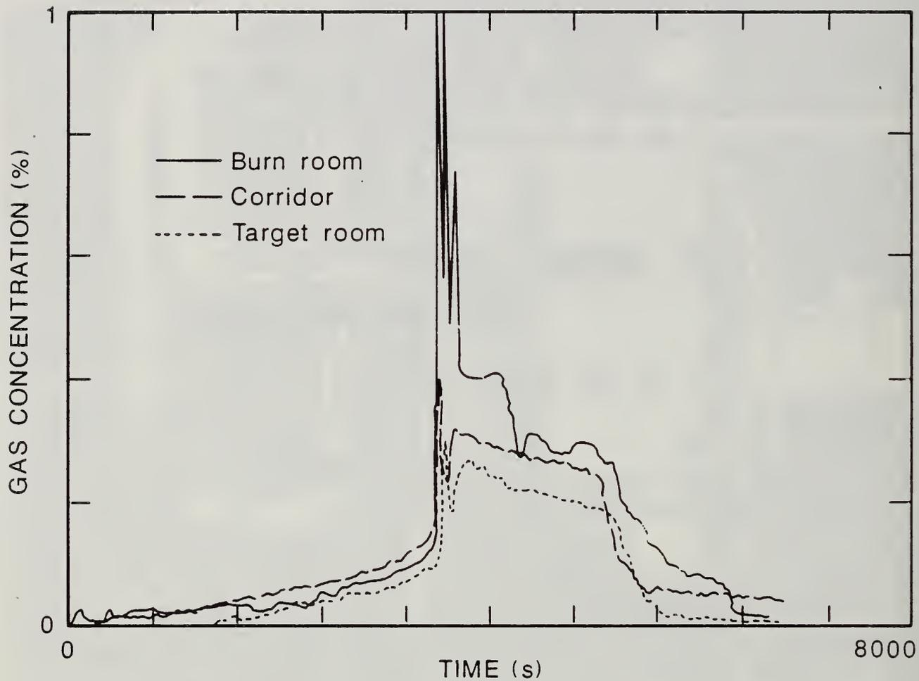
Figure 66. Comparison of Carbon Monoxide Concentrations in Each Compartment of the Large-Scale Test Facility for the Two-Cigarette Test of Foam 32 Mock-up Upholstery Chair Assembly With the Animal Exposure Chambers Connected to the Burn Room.
