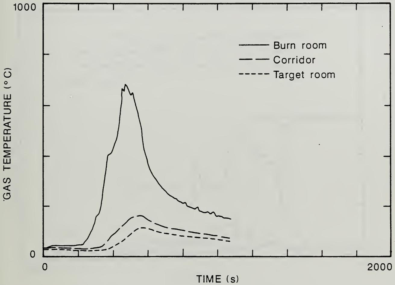
Figure 49. Upper Layer Gas Temperatures in Each Compartment of the Large-Scale Facility During Flaming Ignition Test of Foam 32 Mock-up Upholstery Chair Assembly.
