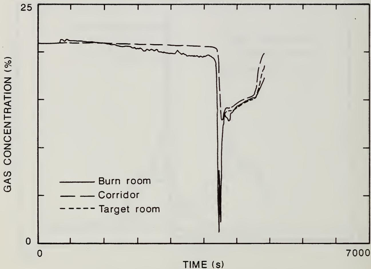
Figure 58. Comparison of Oxygen Concentrations in Each Compartment of the Large-Scale Test Facility for the Two-Cigarette Test of Foam 32 Mock-up Upholstery Chair Assembly.
