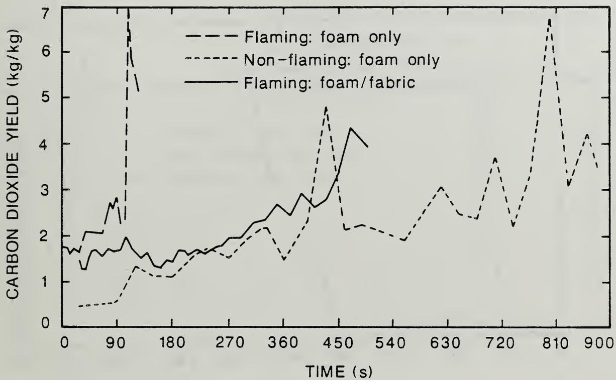
Figure 5. Comparison of Carbon Dioxide Yield for Foam 32 Flaming and Non-flaming Exposures Without a Cover Fabric and Flaming Exposure With a Cover Fabric.
