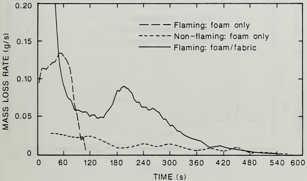
Figure 11. Comparison of Mass Loss Rate for Foam 32X Flaming and Non-flaming Exposures Without a Cover Fabric and Flaming Exposure With a Cover Fabric.
