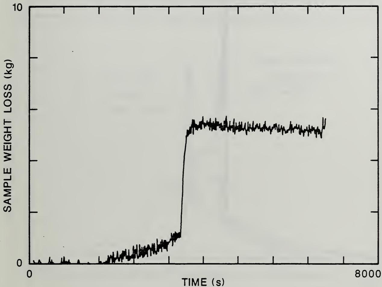
Figure 65. Mass Loss of Upholstery Chair Assembly Made from Foam 32 and Exposed to Two-Cigarettes in the Large-Scale Test Facility With the Animal Exposure Chambers Connected to the Burn Room.
