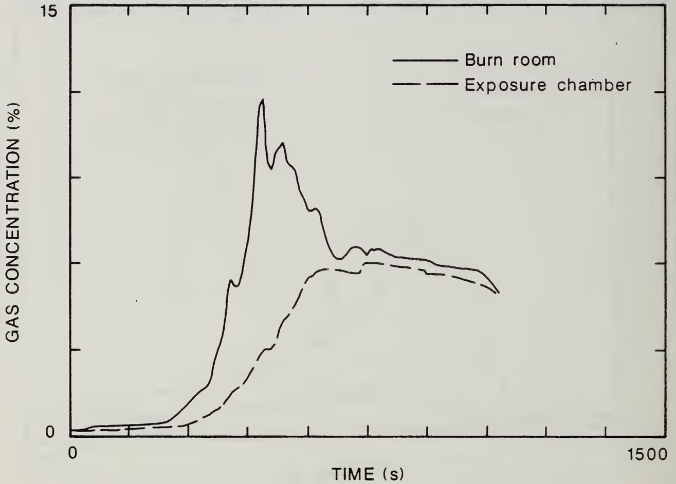
Figure 48. Comparison of Carbon Dioxide Concentration in the Burn Room and the Animal Exposure Chamber for Flaming Ignition of Foam Mock-up Upholstery Chair Assembly.
