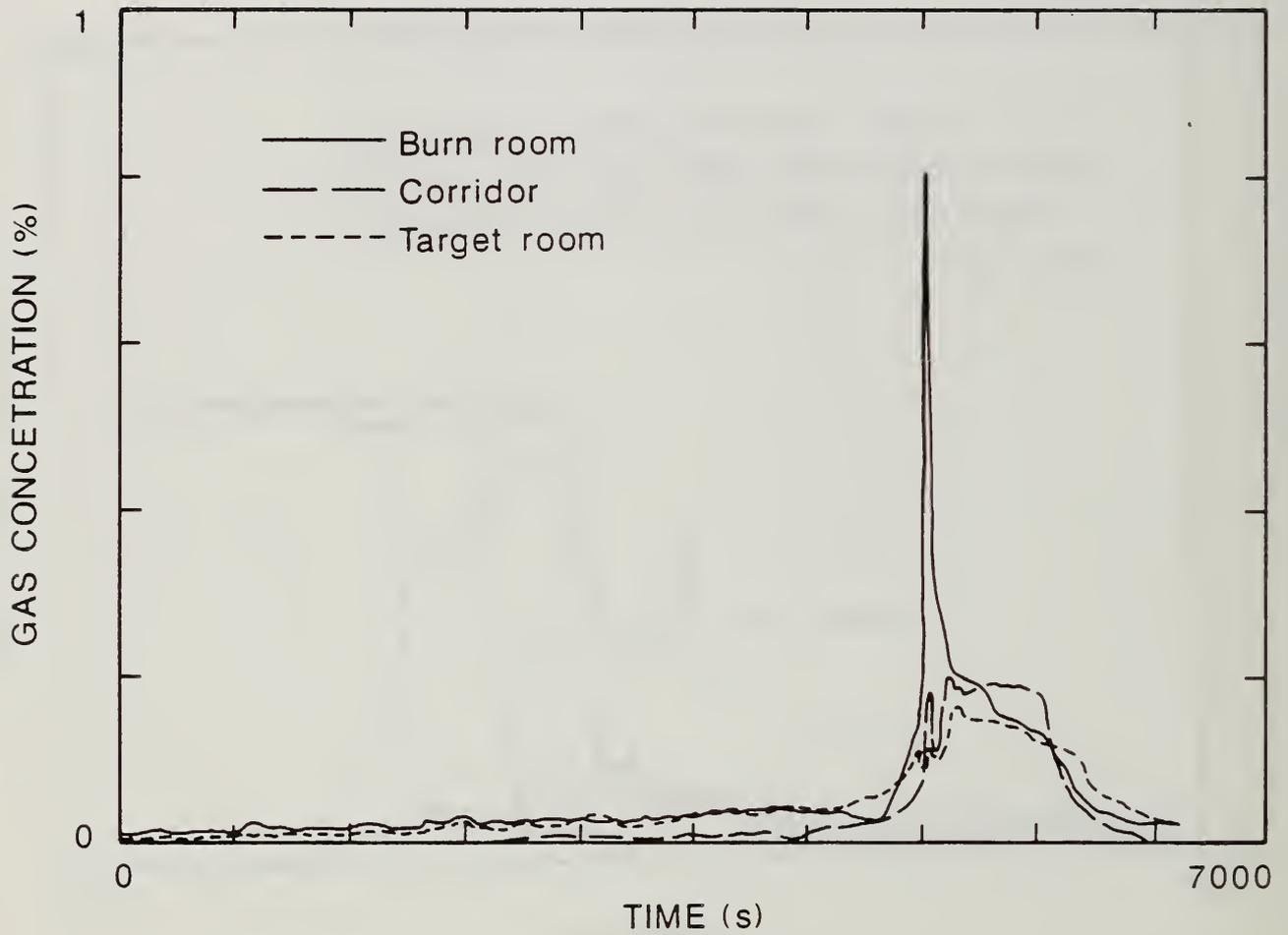
Figure 52. Comparison of Carbon Monoxide Concentrations in Each Compartment of the Large-Scale Test Facility for the One Cigarette Test of Foam 32 Mock-up Upholstery Chair Assembly.
