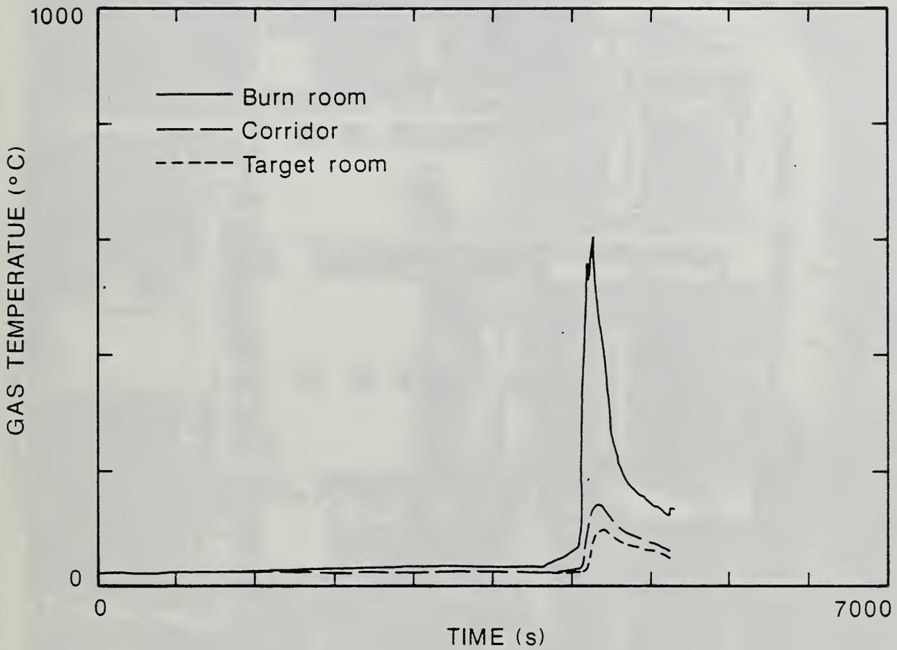
Figure 63. Comparison of the Upper Compartment Gas Temperatures in Each Compartment of the Large-Scale Test Facility for the Two-Cigarette Test of Foam 32X Mock-up Upholstery Chair Assembly.
