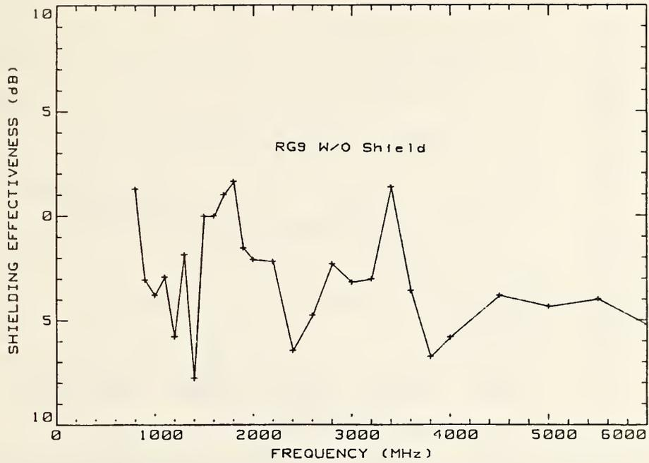
Figure 11. SE of configuration 1 at selected frequencies between 600 and 6000 MHz using the small mode-stirred chamber.
