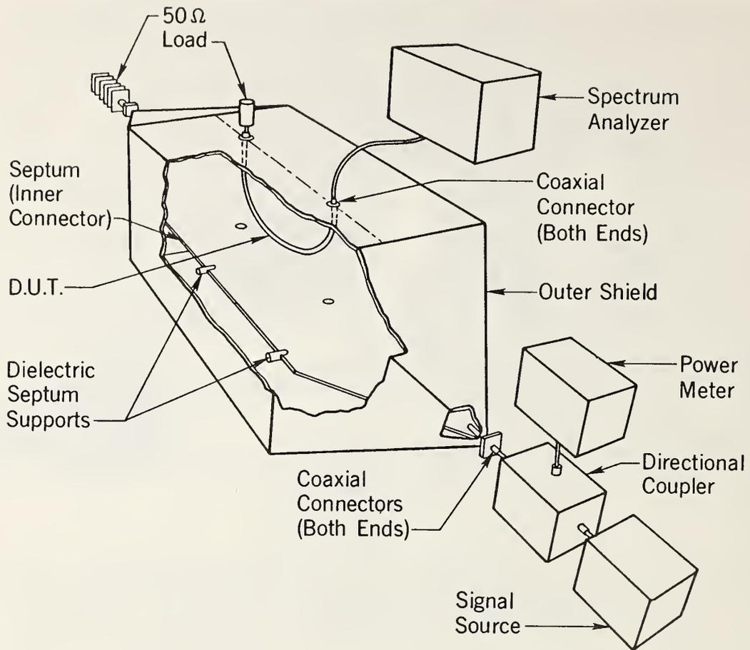
Figure 9. TEM cell and measurement system.
