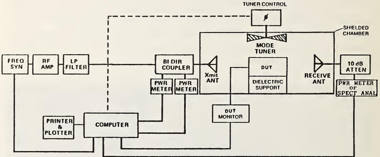
Figure 7. Block diagram of the large mode-stirred chamber and measurement system.
