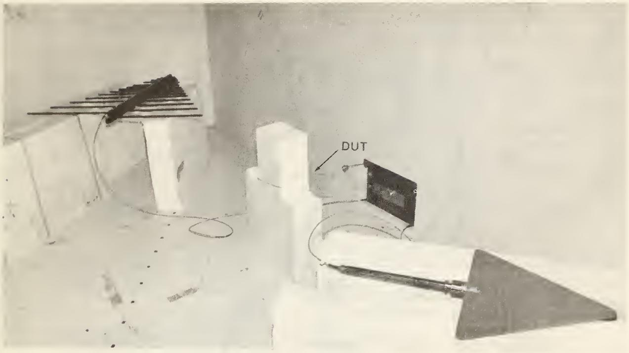
Figure 8. Placement of the DUT and the log periodic antennas inside the large mode-stirred chamber.
