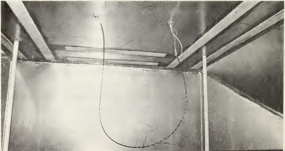
Figure 10. Placement of the DUT inside the TEM cell.
