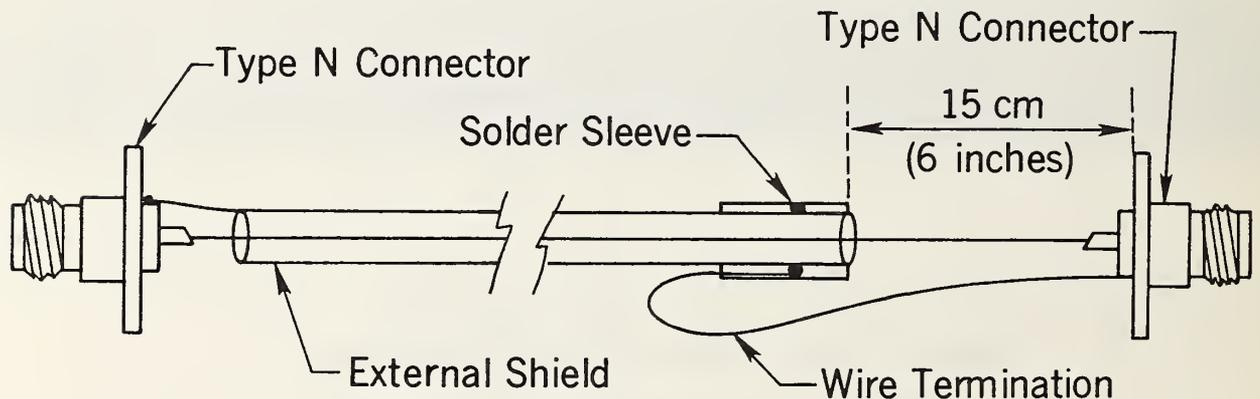
Figure 2. Single shielded wire.
