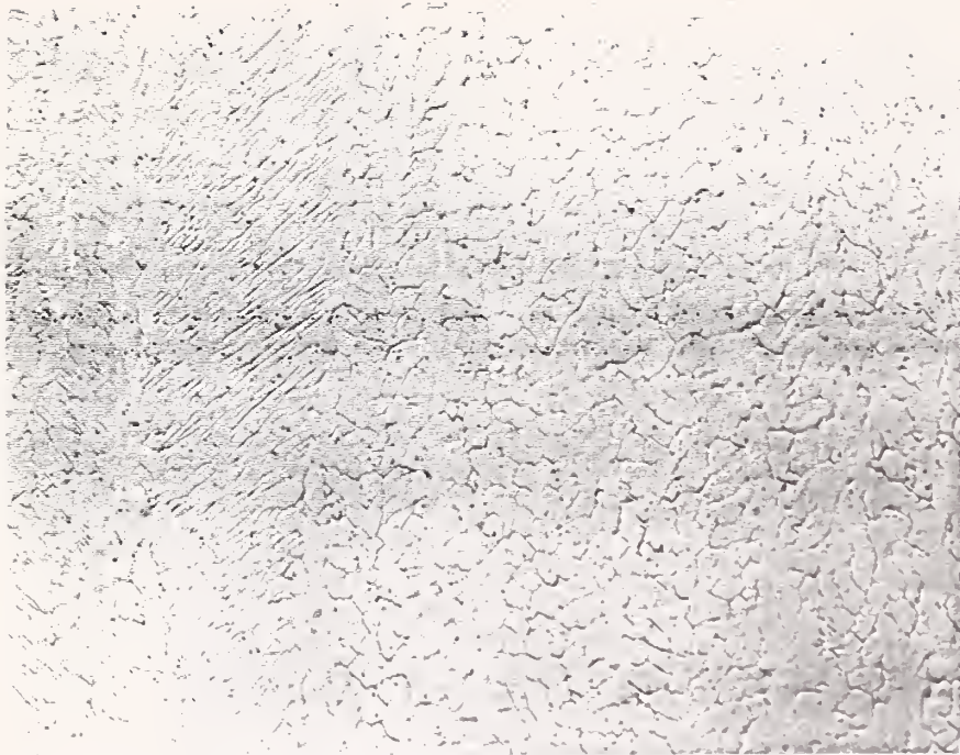
Figure 11. Optical micrograph of the microstructure of weld 6. Vermicular and lacy ferrite morphologies were commonly observed. A hydrochloric-nitric-acetic acid etch was used.
