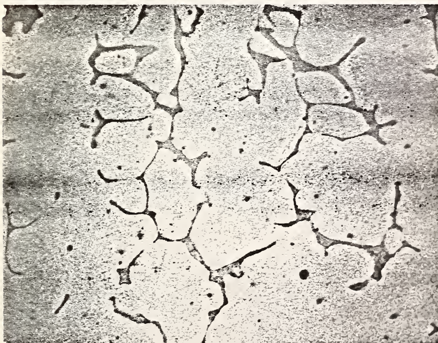
Figure 26. Similarities in the shape and spacing of ferrite morphologies of polished specimens and the tear-ridge networks on the fracture surface for weld 12.
