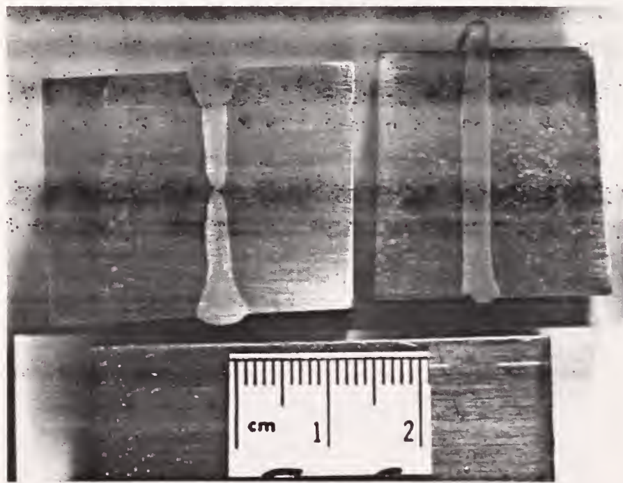
Figure 4. Polished cross sections of laser (left) and EB (right) welds.
