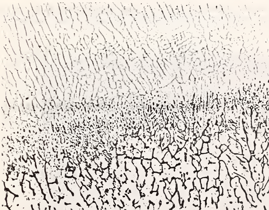
Figure 13. Optical micrograph of the microstructure near an interpass region in weld 22. The weld was etched in a 33 percent nital solution.
