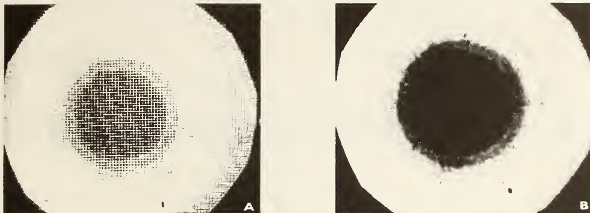
Figure 2. Radial transmittance function displayed on the LCD monitor, A, before low pass filtering, B, after low pass filtering. Contrast ratio of B is 5 times that of A.
