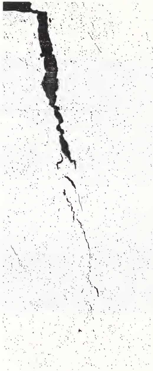
Primary Crack in Cylinder Neck Cyl. No. WK-32699 Mag. 40x
