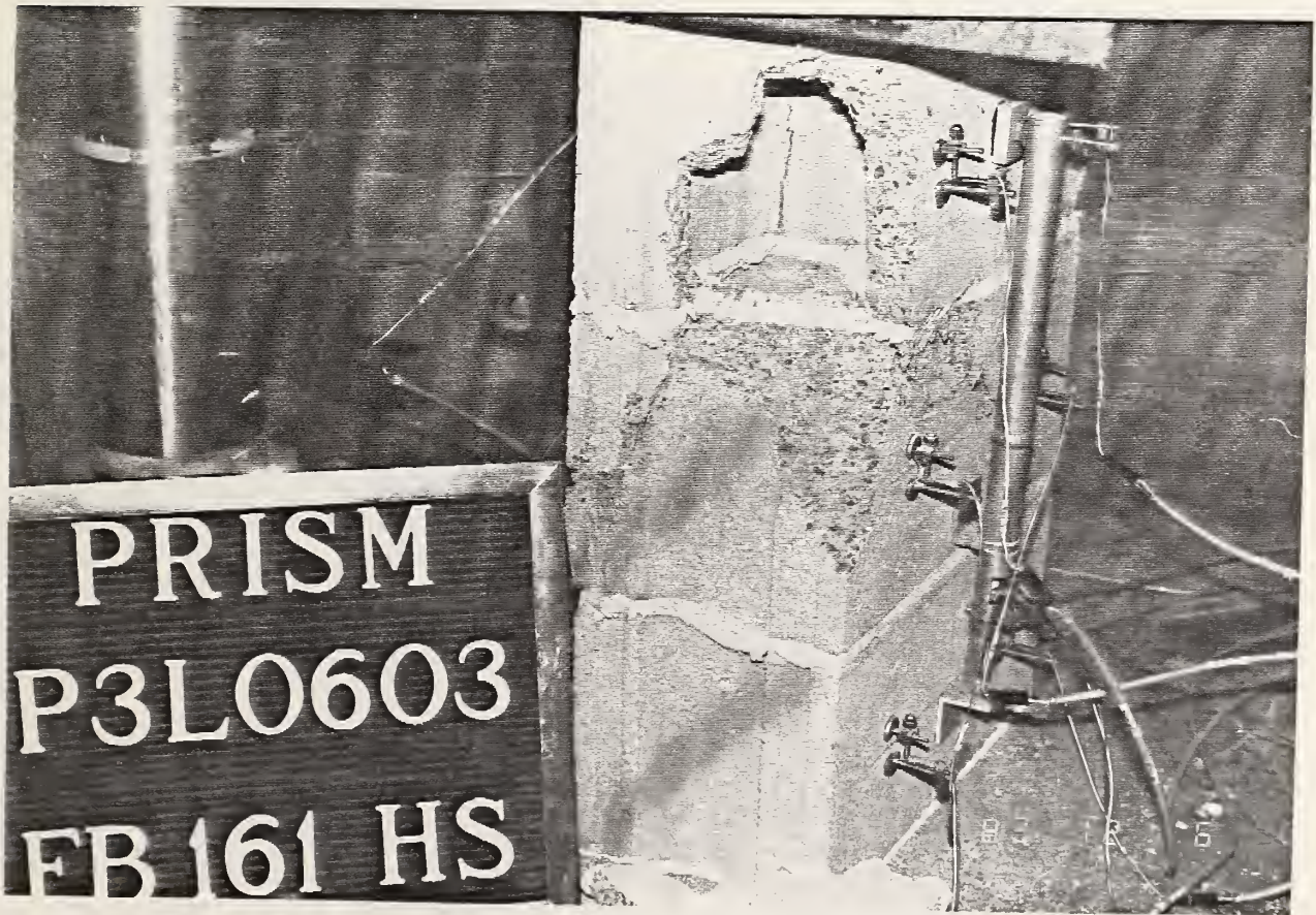
Figure 3.1 Failure of a full-area-bedded prism
