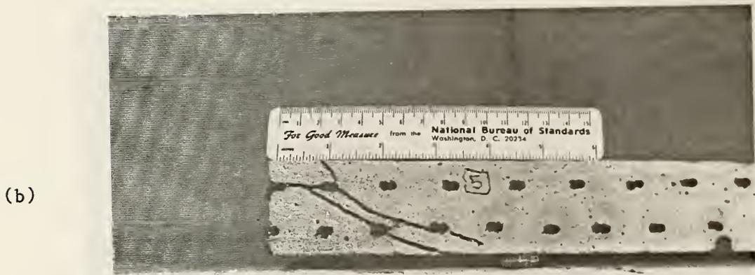
Fig. 4.5 Cracks in specimen no. 5: a) transverse cross-section; and b) span cross-section on half the specimen.
