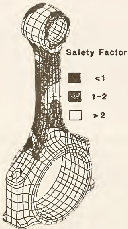
Fig. 7. Finite-element analysis of a connecting rod.
