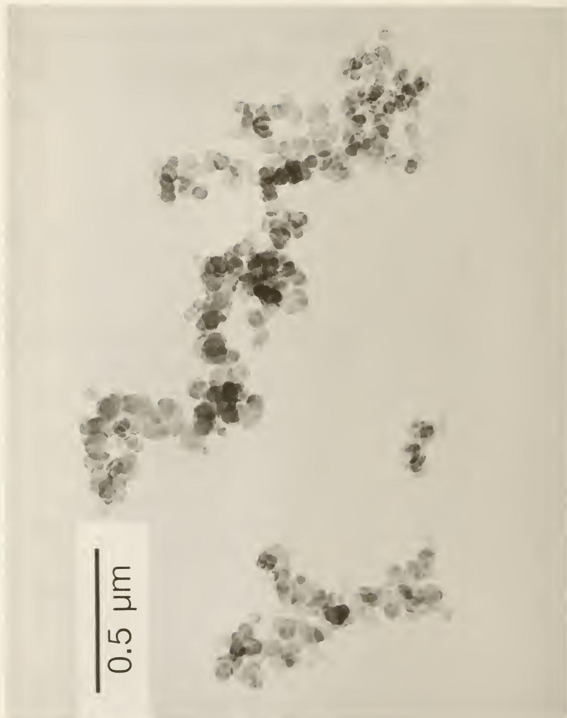
Figure 12. Electron Micrograph of Smoke Particles Produced by 0.6 Meter Diameter Prudhoe Bay Crude Oil Pool Fire, 0.5 Micrometer Scale
