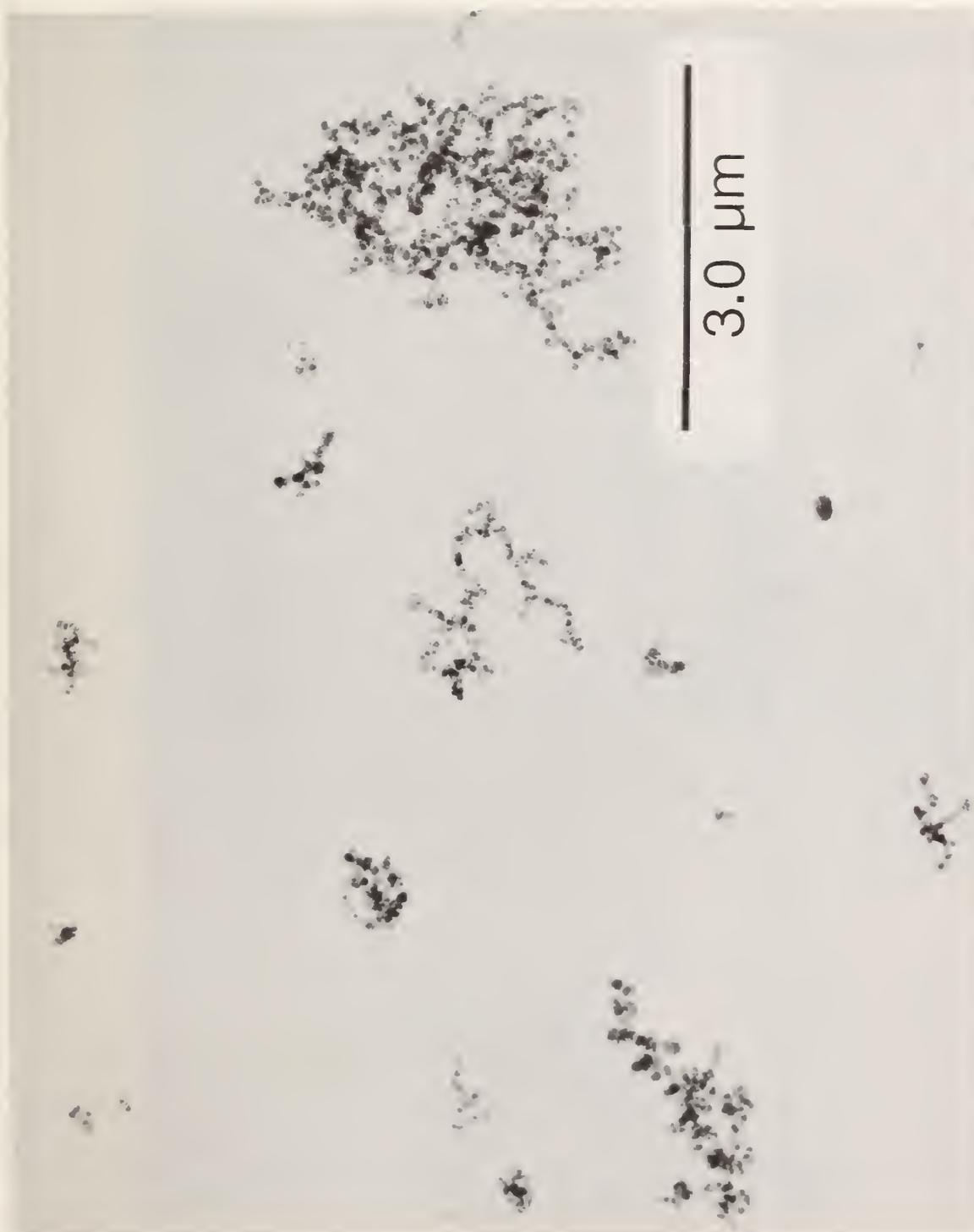
Figure 11. Electron Micrograph of Smoke Particles Produced by 0.6 Meter Diameter Prudhoe Bay Crude Oil Pool Fire, 3 Micrometer Scale
