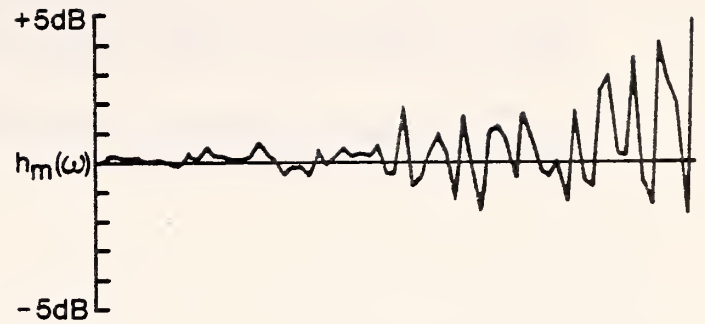
Figure 12. h_m(\omega) was calculated after using corrections obtained by the Marquardt algorithm. The high-frequency roll-off has vanished.
