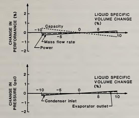
Figure 5. Sensitivity of performance of a heat pump to a change in liquid specific volume.
