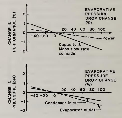
Figure 10. Sensitivity of performance of a heat pump on a change in the evaporative pressure drop.
