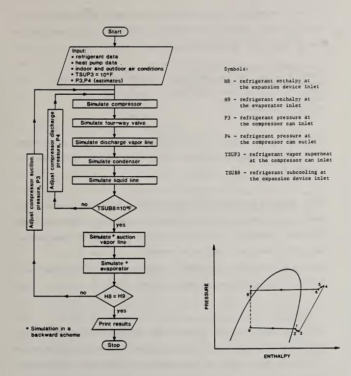
Figure 2. Logic of the heat pump model used in the sensitivity study.
