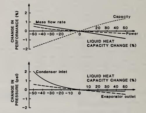
Figure 7. Sensitivity of performance of a heat pump on a change in the heat capacity of liquid.
