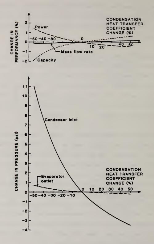
Figure 9. Sensitivity of performance of a heat pump on a change in the condensation heat transfer coefficient.
