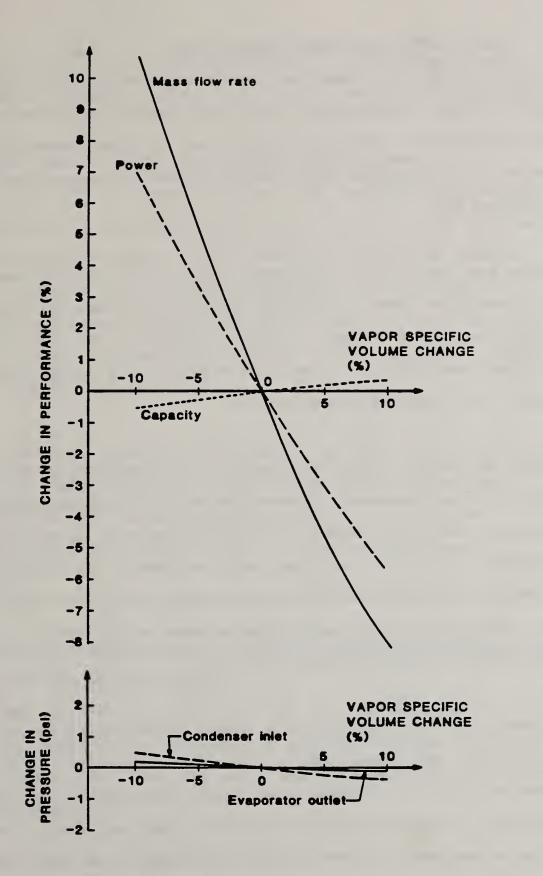
Figure 6. Sensitivity of performance of a heat pump to a change in vapor specific volume.
