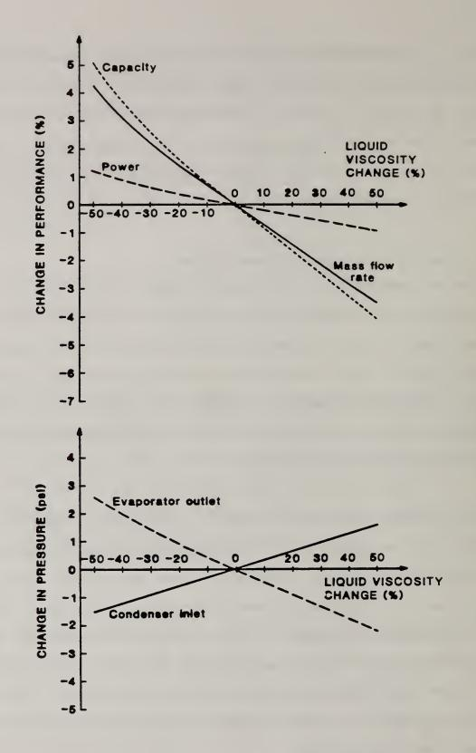
Figure 3. Sensitivity of performance of a heat pump to a change in liquid viscosity.
