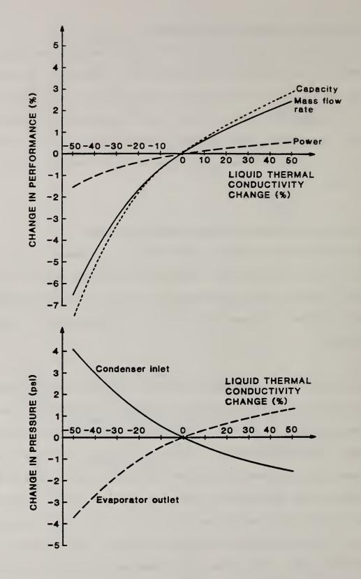
Figure 4. Sensitivity of performance of a heat pump to a change in liquid thermal conductivity.
