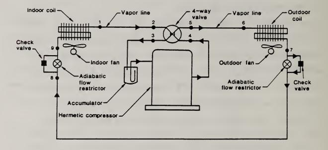
Figure 1. Schematic of a heat pump simulated by the heat pump model, HPSIM.
