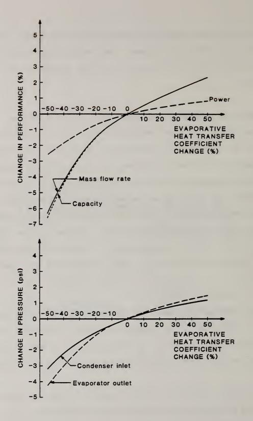
Figure 8. Sensitivity of performance of a heat pump on a change in the evaporative heat transfer coefficient.
