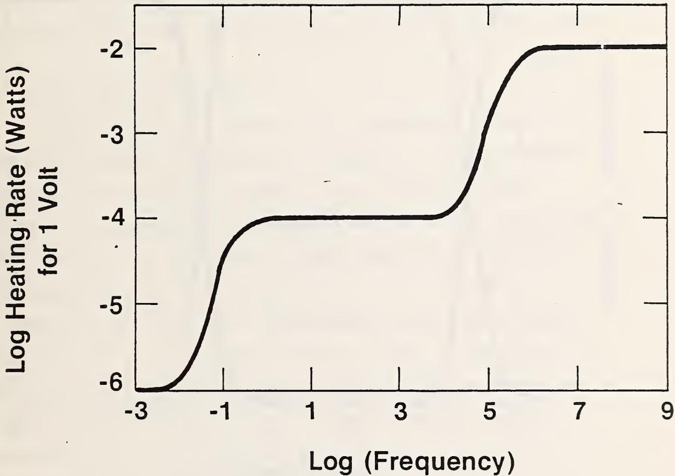
Figure 5. Rate of dielectric heating in watts of the model circuit of figure 4 as a function of frequency for an applied potential of 1 volt.
