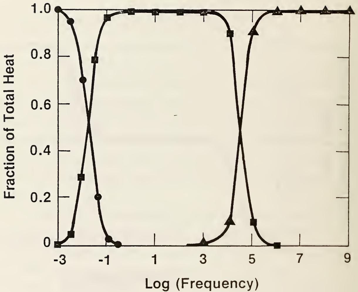
Figure 6. Fraction of total heating in each of the three parts of the circuit in figures 3 and 4. The symbols are for circuit 1, circuit 2, ■; circuit 3, ▲.
