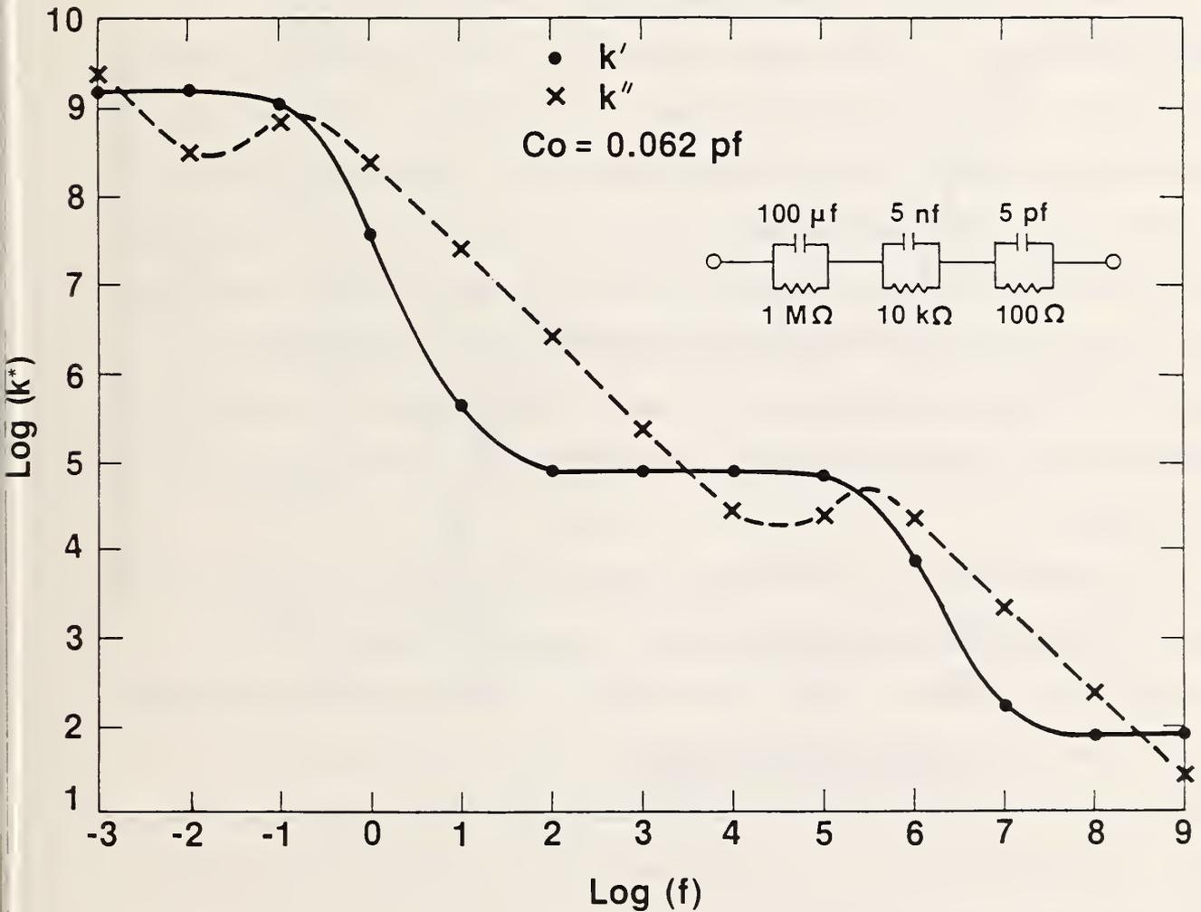
Figure 4. Real and imaginary parts of the complex dielectric constant for the model circuit of figure 3, using the resistance and capacitance values shown in the insert, and assuming an empty holder capacitance of 0.062 pf.
