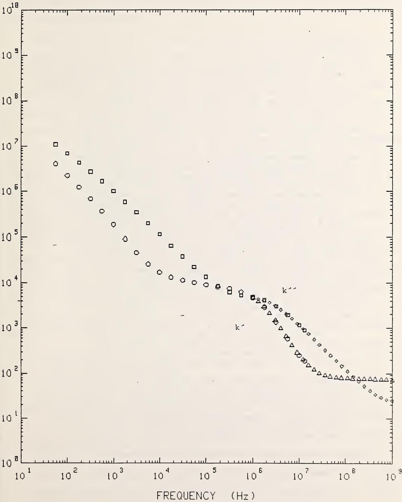
Figure 17. Dielectric properties of the synthetic phantom material with a single film of PET completely covering one electrode.
