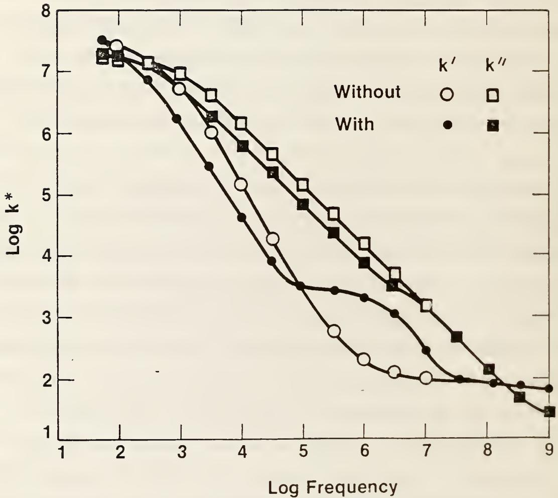
Figure 14. Dielectric properties of a 50/50 mixture of ethylene carbonate and propylene carbonate with 0.28 molar tetraethylammonium tetrafluoroborate. A single film of 1.5  $\mu\text{m}$  thick PET the same diameter as the specimen holder is used for the "with" data.
