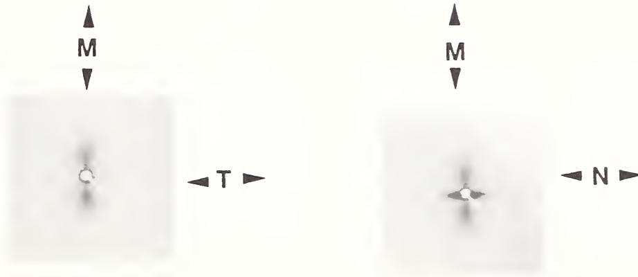
Fig. 22. Small angle x-ray diffraction patterns from film F1. Incident beam in (a) parallel to N direction, (b) parallel to T direction.
