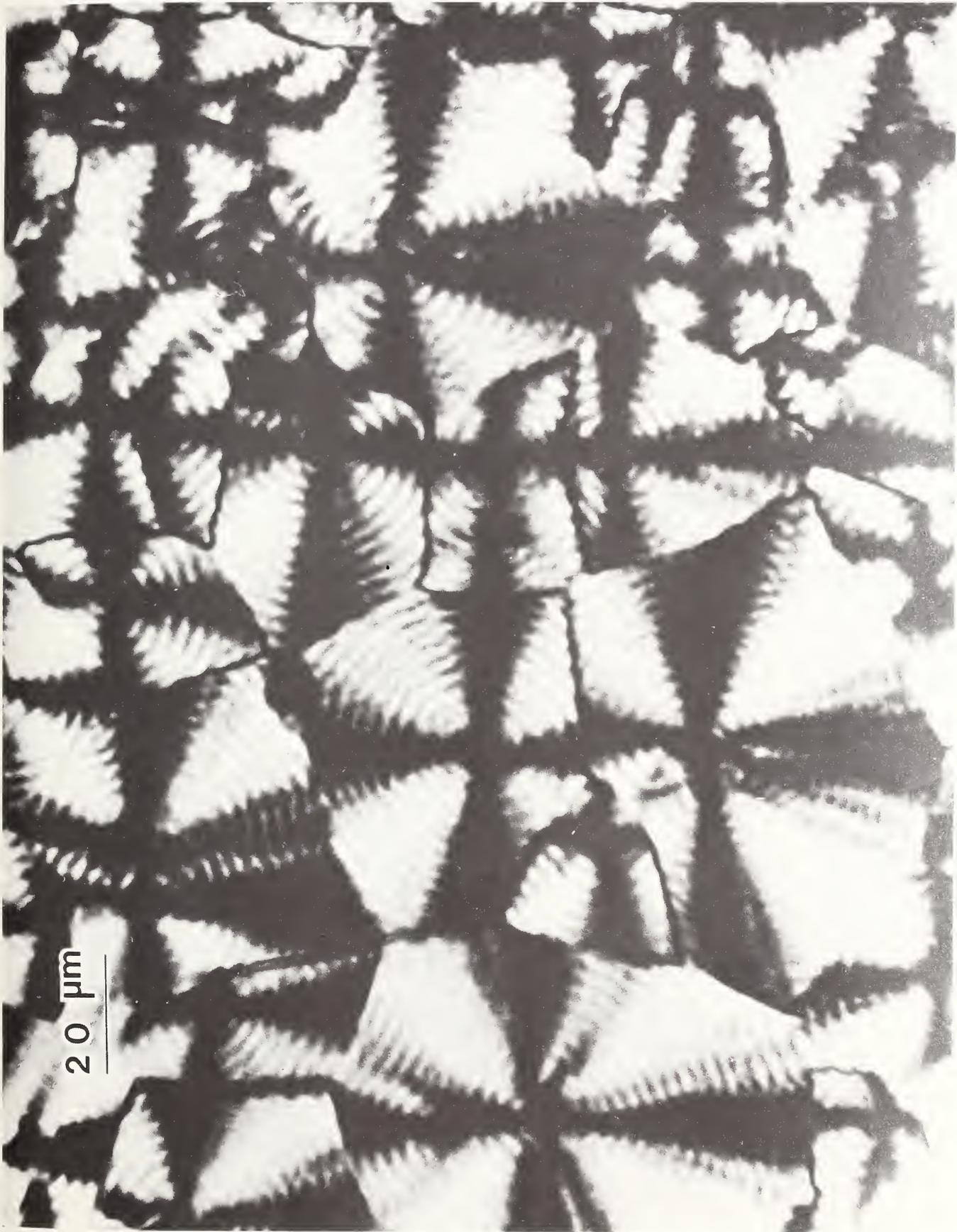
Fig. 25a. Spherulites in a sample of linear polyethylene as seen with a polarizing microscope (crossed polarizer and analyzer).
