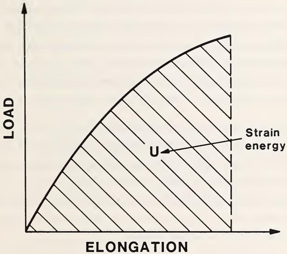
Figure 1. Strain energy: the area under the load-elongation curve
