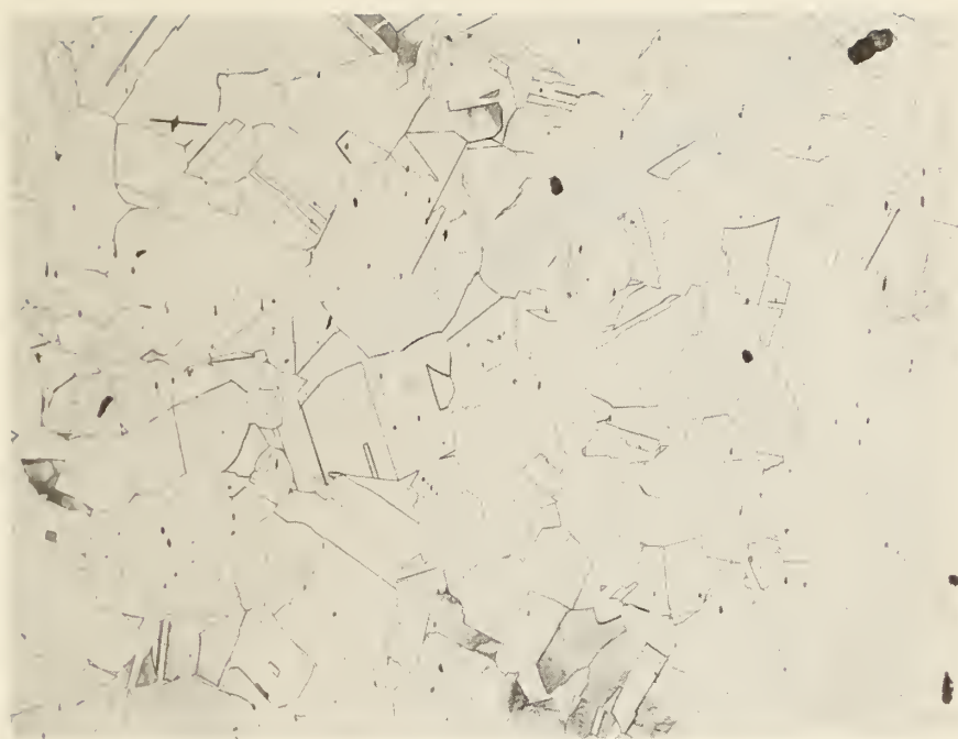
Fig. 1. Photomicrograph of typical studied alloy. Average grain size for nine alloys equals 88 \mu\text{m} .
