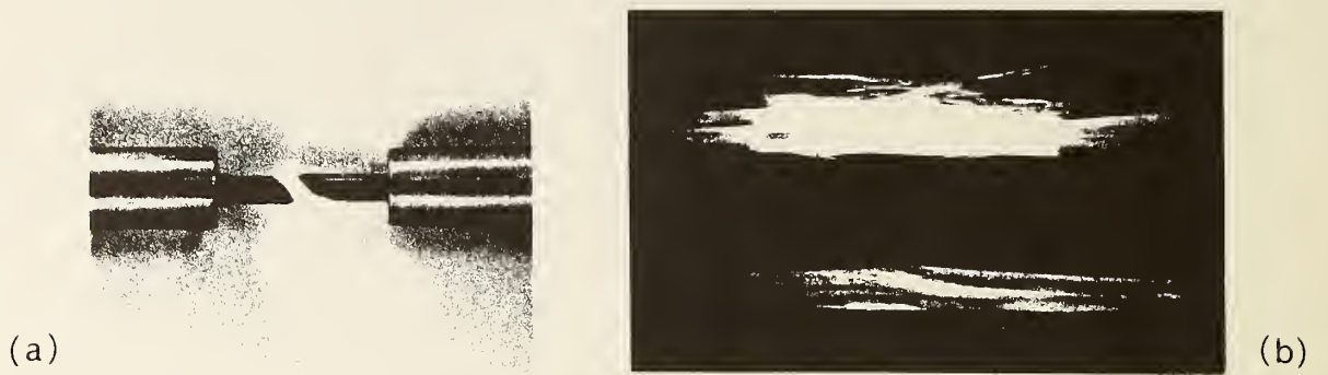
Fig. 4. (a) Typical 76-K torsional failure in an unreinforced resin specimen illustrating the method of holding in aluminum end caps. (b) Typical 76-K torsional failures in glass-reinforced Rutherford resin system (material 3, Table 1).
