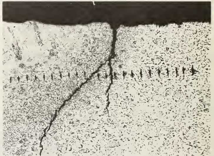
c. Crack in HAZ 3 and microhardness indentations at location B in Figure 32a
