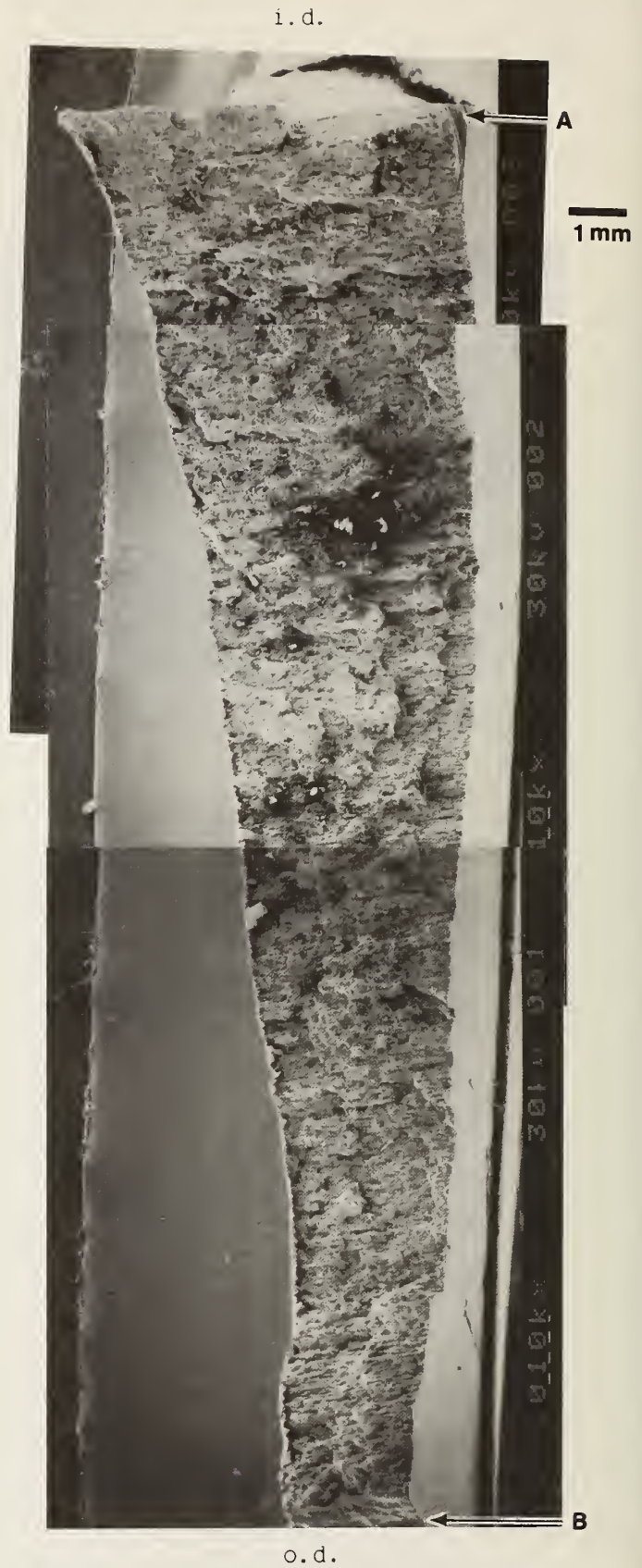
b. SEM fractograph of the fracture surface at the location shown in Figure 36a
