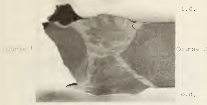
a. Macrostructure of Weld 1/2 at CC 1.3 m
