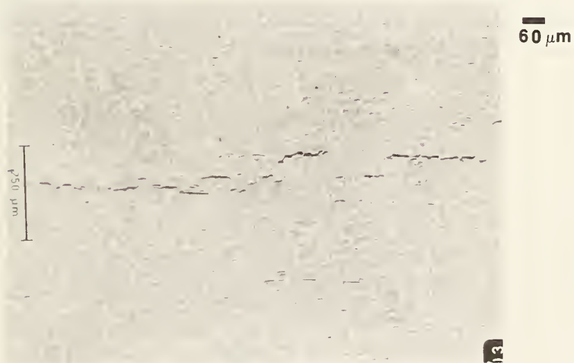
b. Cracks in Course 2 of Specimen I2 of Weld 2/3
