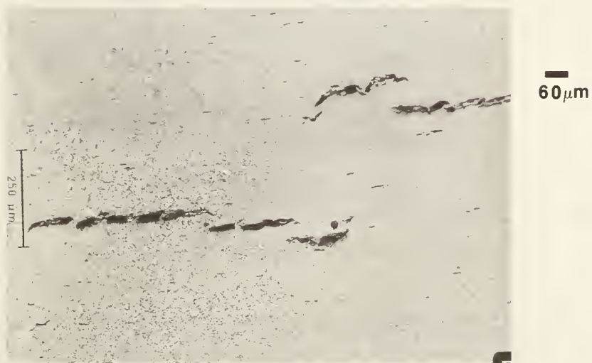
c. Cracks in HAZ 3 of Specimen I2 of Weld 2/3
