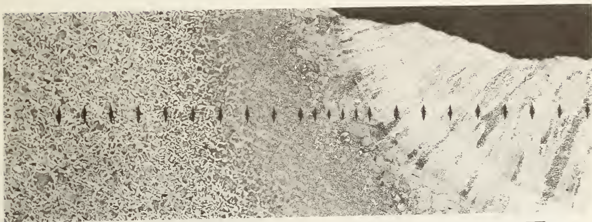
b. Knoop microhardness values of HAZ 3 at location A in Fig. 33a 200 μm
