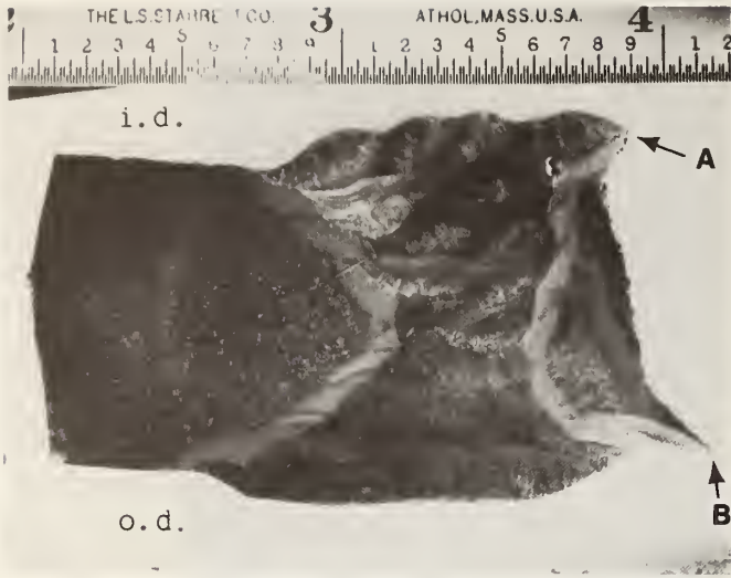
a. Macrostructure of Weld 1/2 at CC 7.3 m
