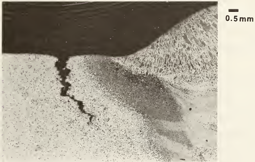
b. Crack at location A in Figure 17a
