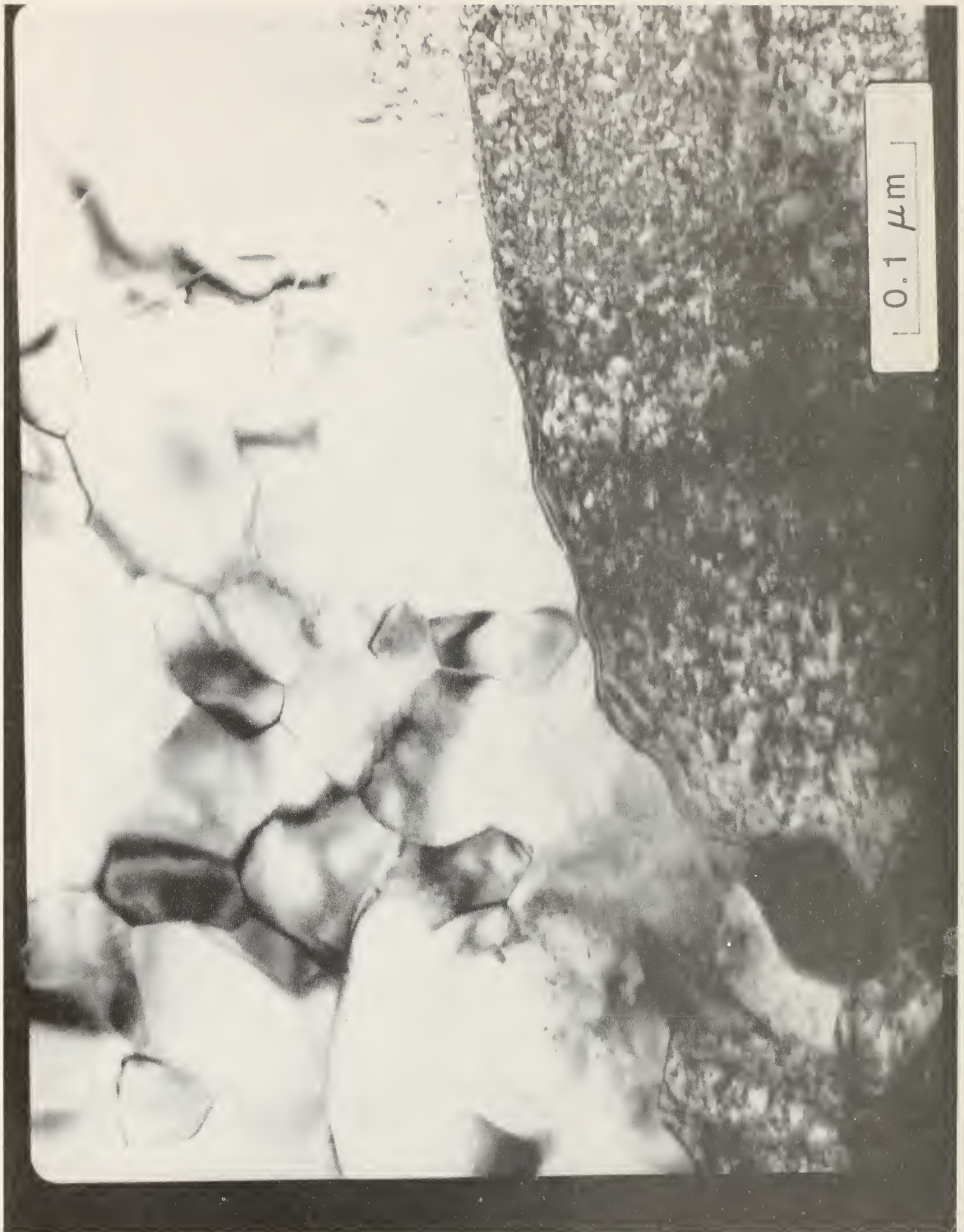
Fig. 2. Typical transmission electron micrograph showing fine equiaxed Al5 grains embedded in the Nb-Ta matrix filled with a high density of dislocations. The mark in the figure is 0.1 μm long.
