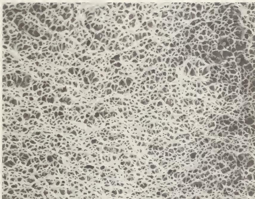
Figure 11. Fracture surface dimple size in the weld.
