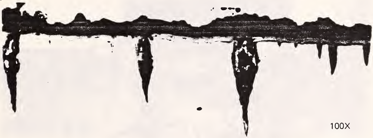
FIGURE 33. INTERNAL SURFACE CORROSION FATIGUE NOTCHES (100X)
