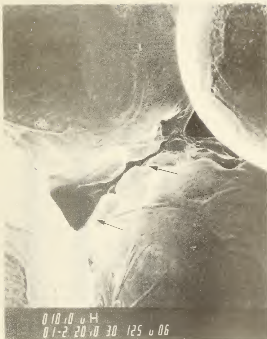
Figure 5. Scanning electron micrograph of neck region connecting sintered Co-Cr-Mo spheres after corrosion testing.
