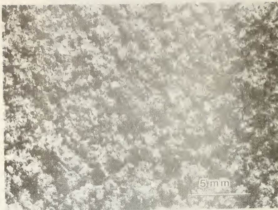
Figure 5. Light micrograph showing surface morphology of an APS Ti-6Al-4V coating on a Ti-6Al-4V substrate.
