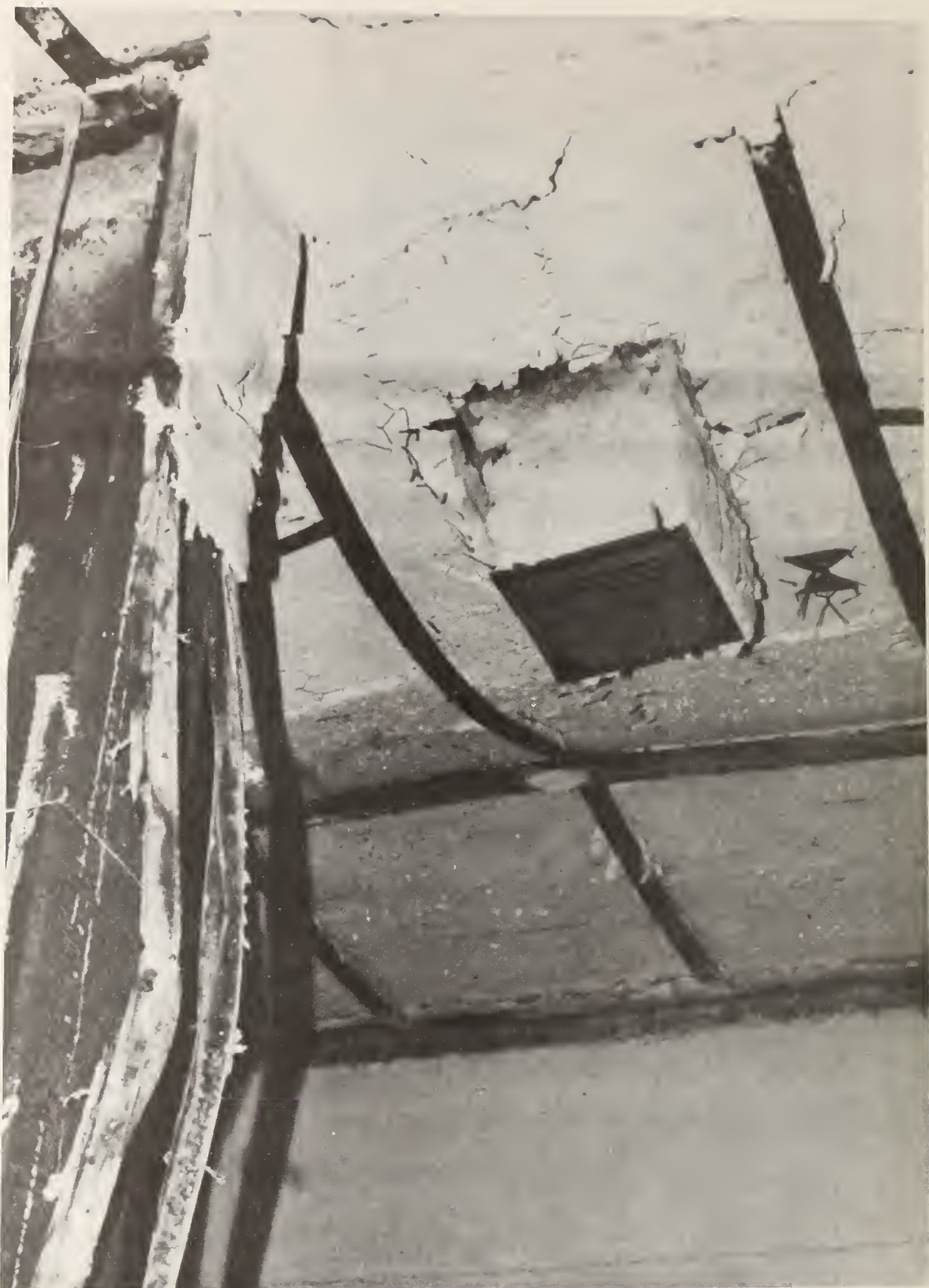
Figure 112. Photograph showing bottom of gypsum walk-on deck after test 3
