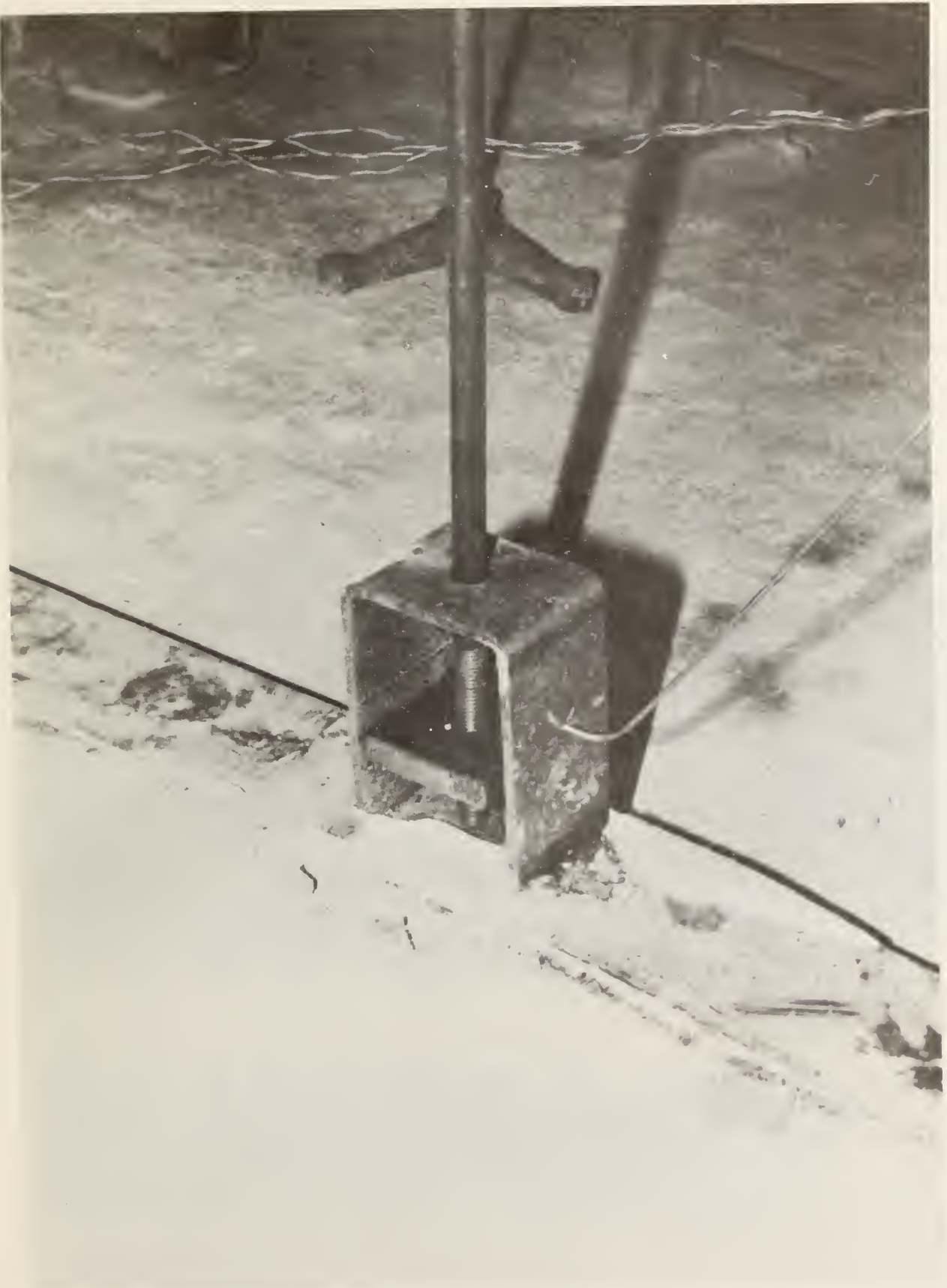
Figure 51. Photograph showing permanent upward set of suspended purlin, test 1
