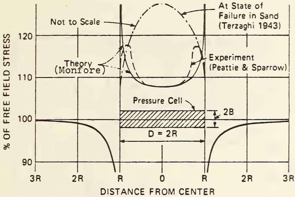
Figure 2 Stress Distribution over Stress Gage (Ref. 11)
