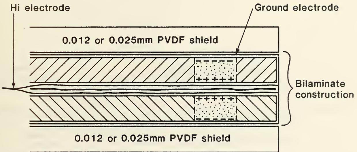
Figure 8 The Polymer Gage - Bilaminate Construction with PVDF Sheets as Protective Covers (Type B Gage)
