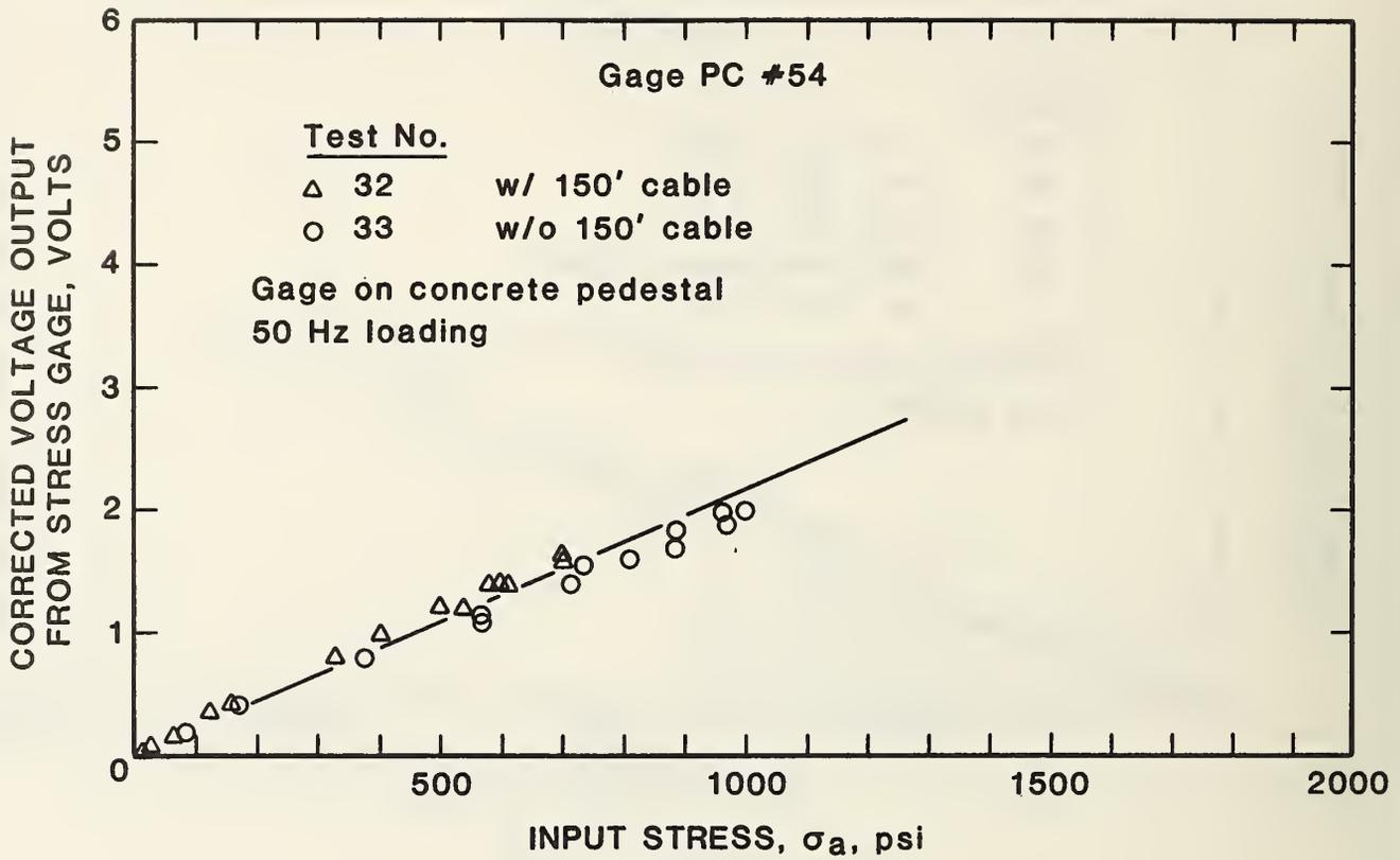
Figure 25      NBS Polymer Gage Test Results - Effect of Cable Length
