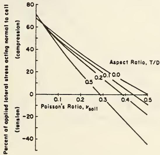
Figure 3 Theoretical Lateral Stress Rotation for Rigid Ellipsoidal Inclusion (Ref. 2)
