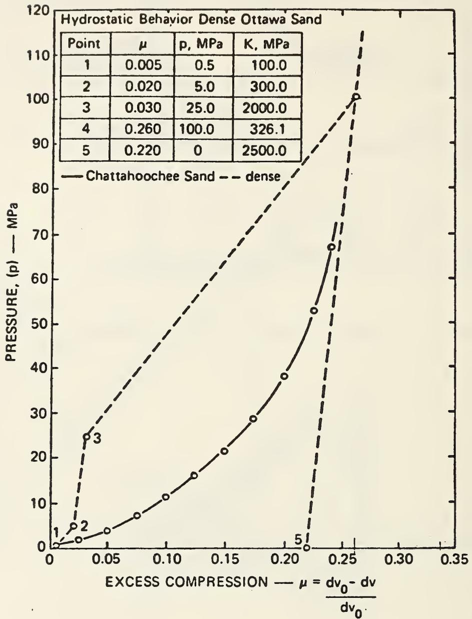
Figure 4 Computational Model of Dense Ottawa Sand - Volumetric Behavior (Ref. 14)
