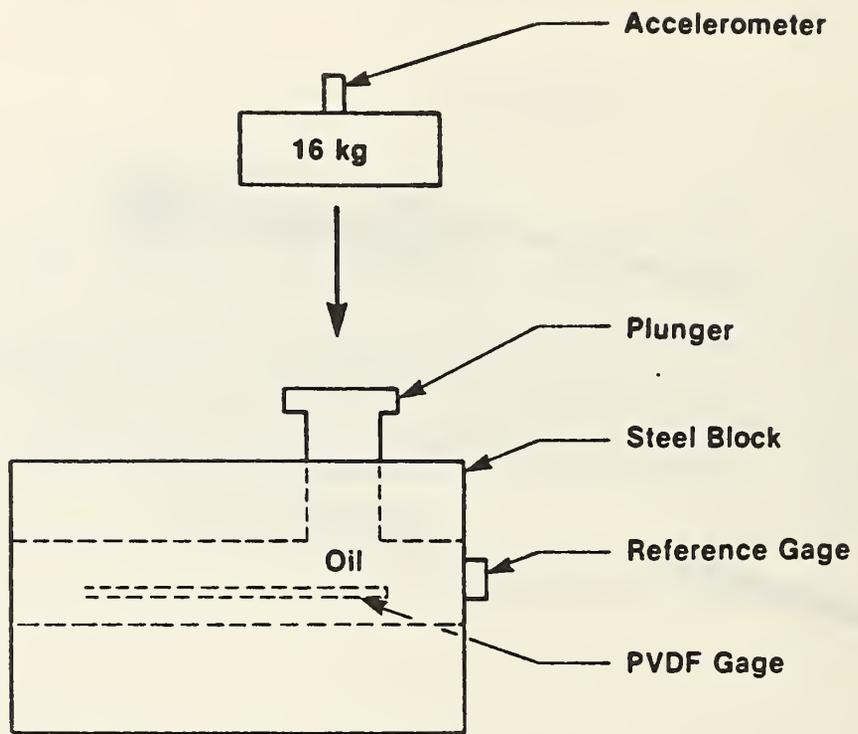
Figure 11 Drop Test Set-up
