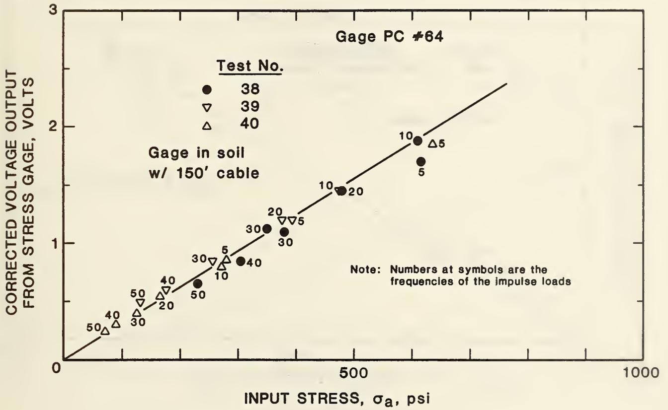
Figure 30 NBS Polymer Gage Test Results - Effect of Frequency, Gage PC #64
