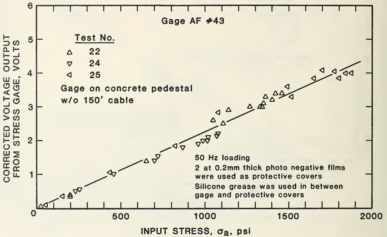
Figure 23 NBS Polymer Gage Test Results - Photo Negative Films Used as Protective Covers
