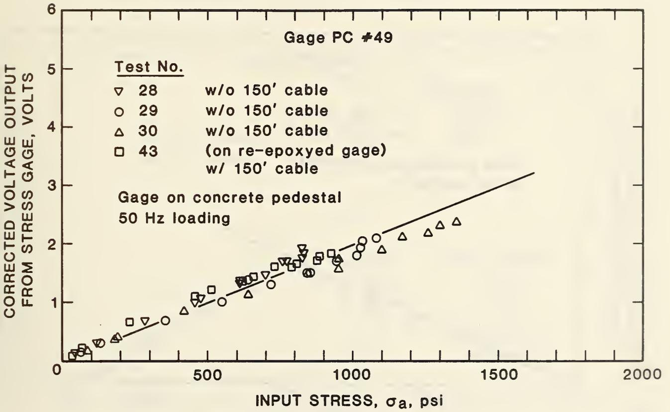
Figure 24 NBS Polymer Gage Test Results - Effect of Cable Length
