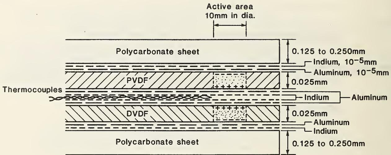
Figure 9 The Polymer Gage - Bilaminate Construction with Polycarbonate Sheets as Protective Covers (Type D and E Gages)
