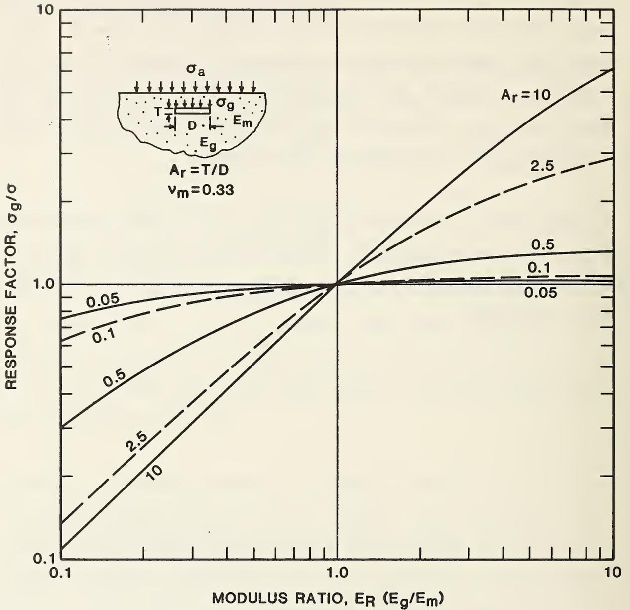
Figure 1 Theoretical Soil Stress Gage Response (Ref. 17)
