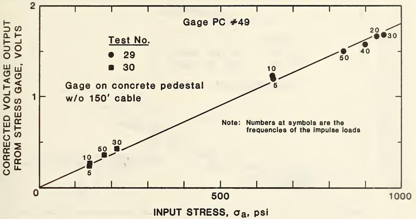
Figure 28 NBS Polymer Gage Test Results - Effect of Frequency, Gage PC #49
