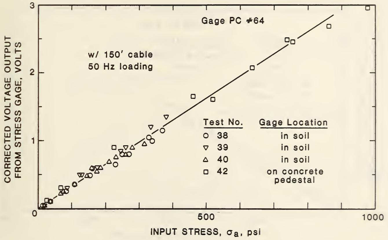
Figure 26 NBS Polymer Gage Test Results - Effect of Gage Location
