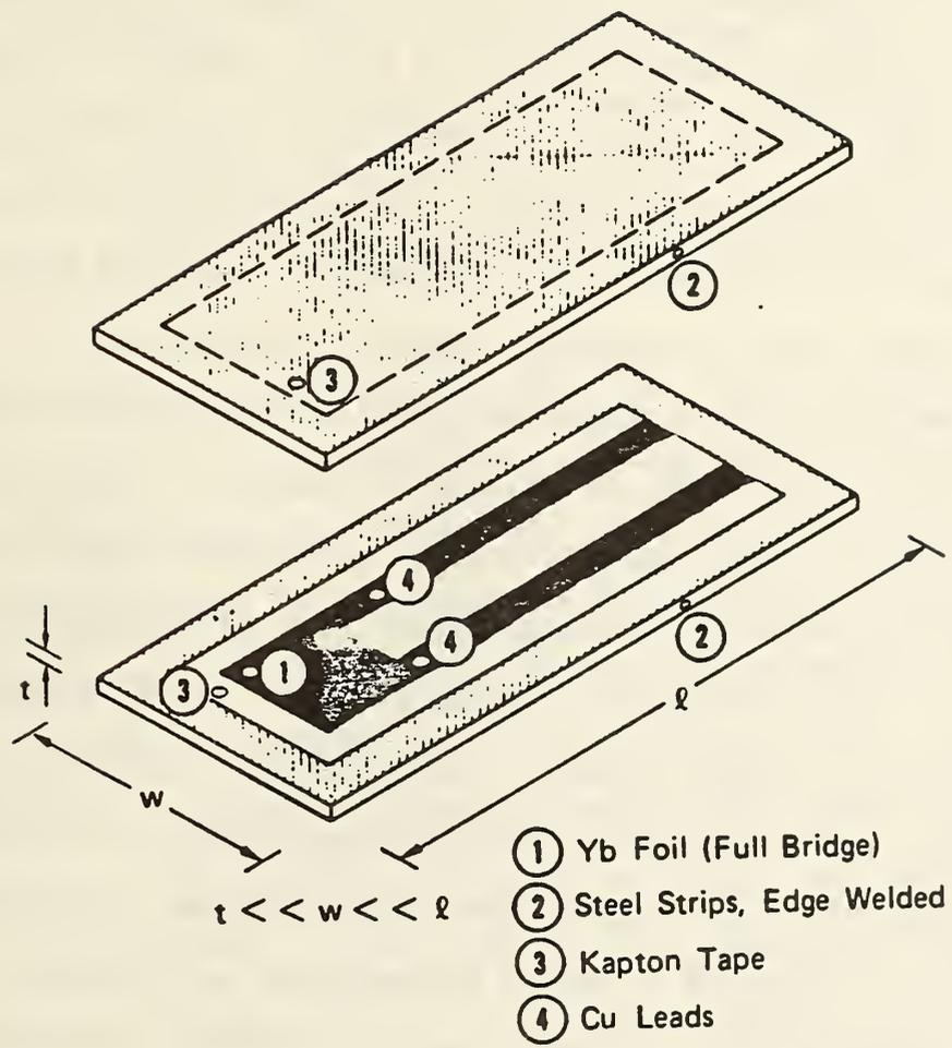
Figure 5 Basic High Modulus Configuration for the SRI Gage (Ref. 13)
