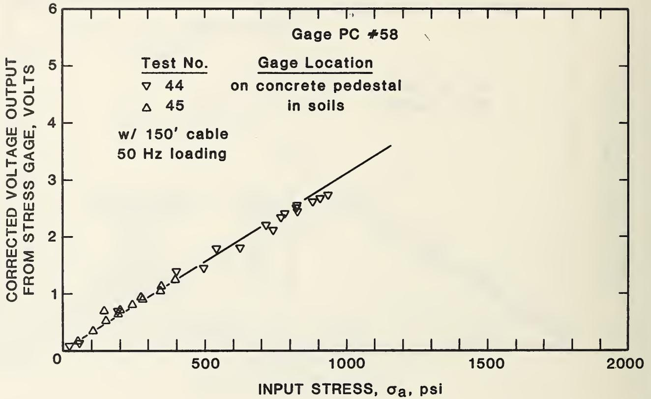
Figure 27      NBS Polymer Gage Test Results - Effect of Gage Location
