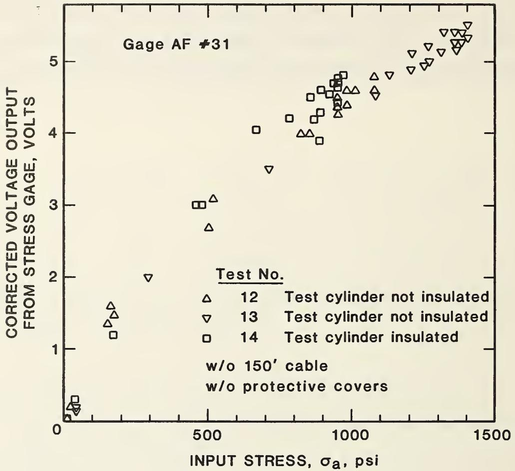
Figure 19 NBS Polymer Gage Test Results - Effect of Test Cylinder Insulation
