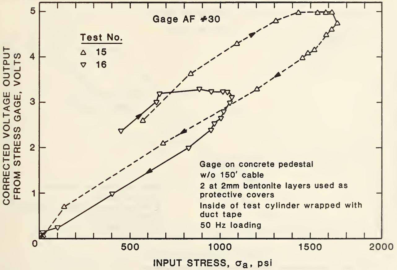
Figure 20 NBS Polymer Gage Test Results -- Bentonite Layers Used as a Protective Covering with The Test Cylinder Insulated
