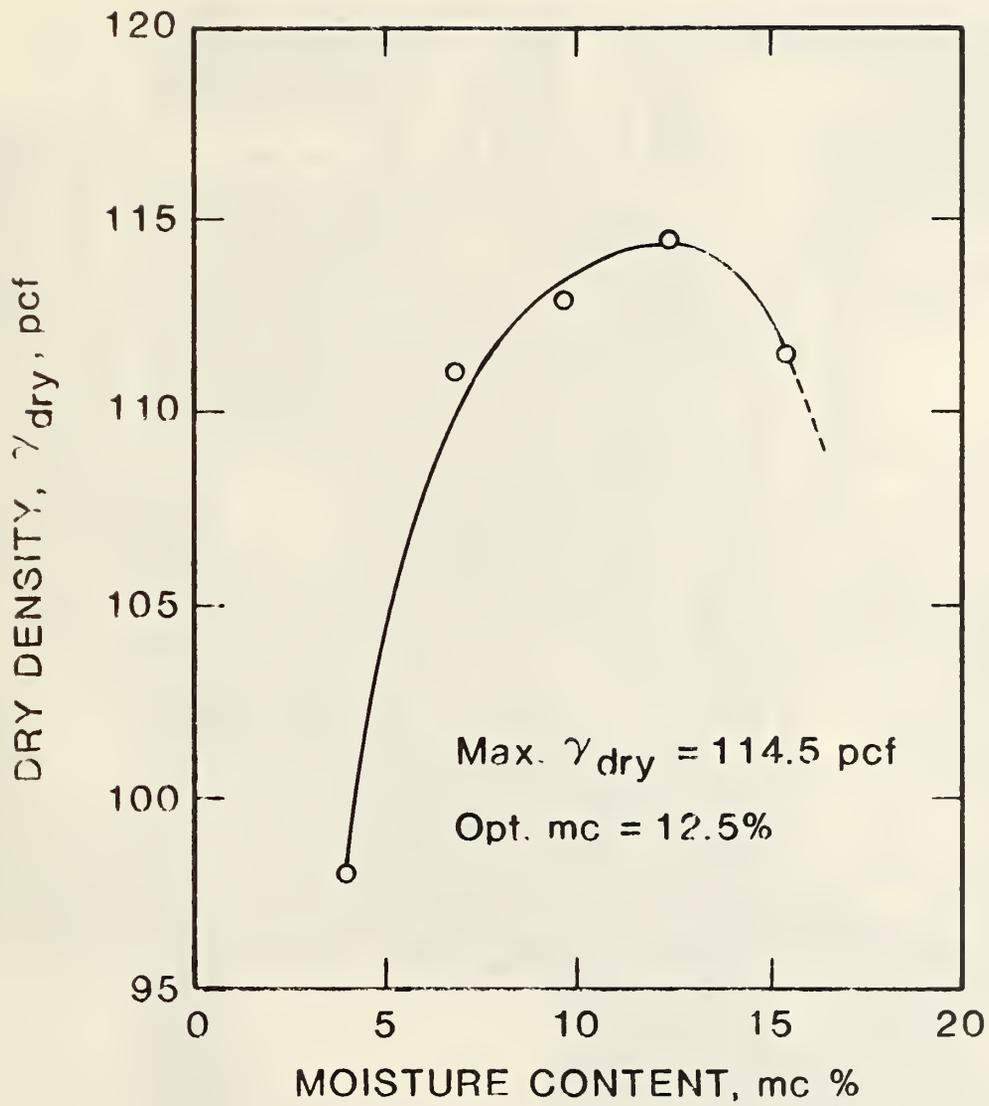
Figure 14 Compaction Curve of Florida Sand
