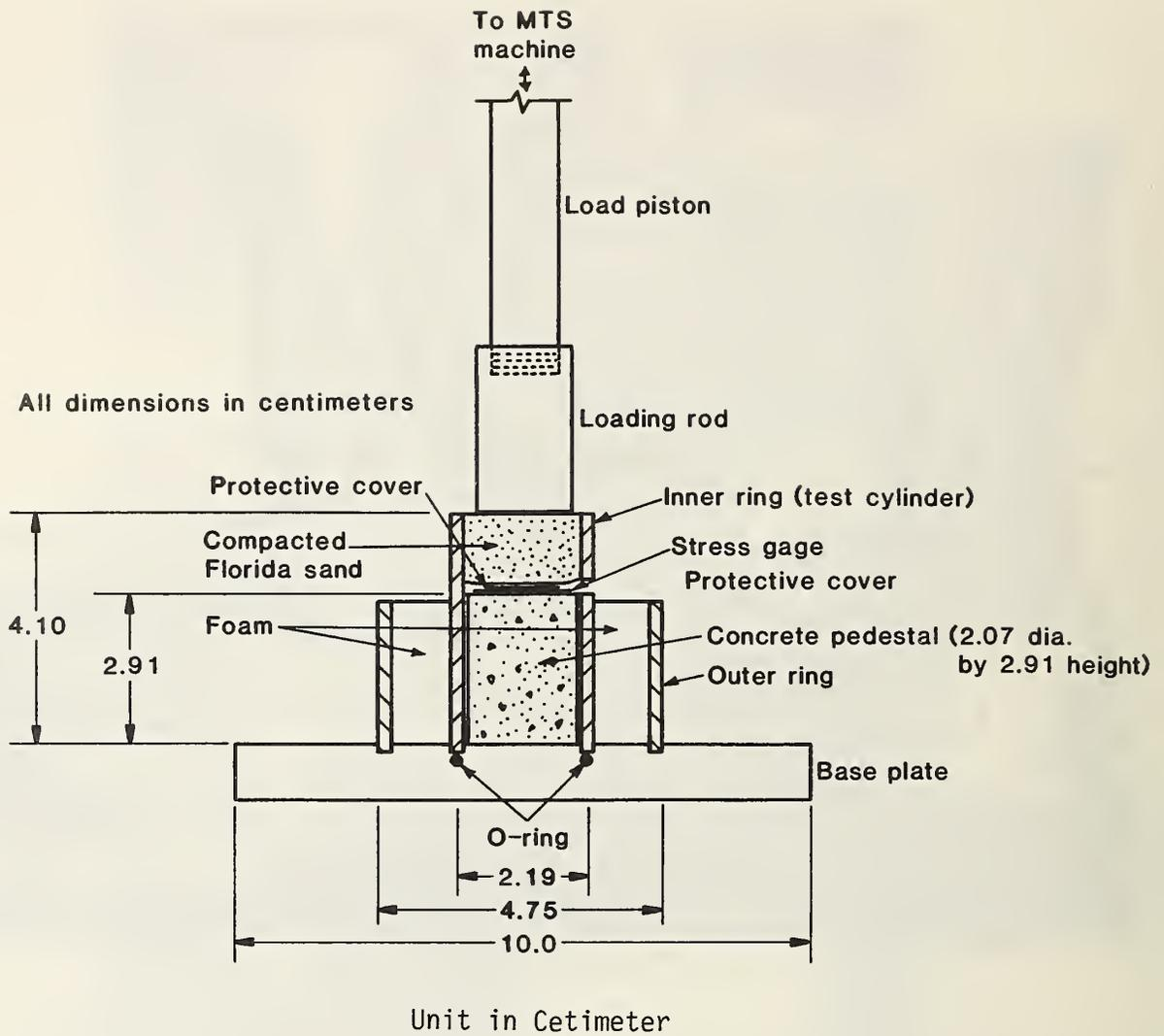
Figure 17 Schematic Drawing of The Test Cylinder and Its Accessories
