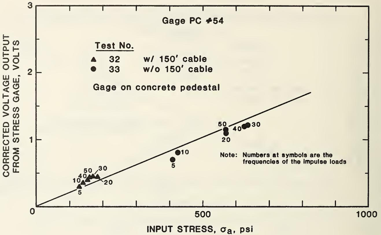
Figure 29 NBS Polymer Gage Test Results - Effect of Frequency, Gage PC #54
