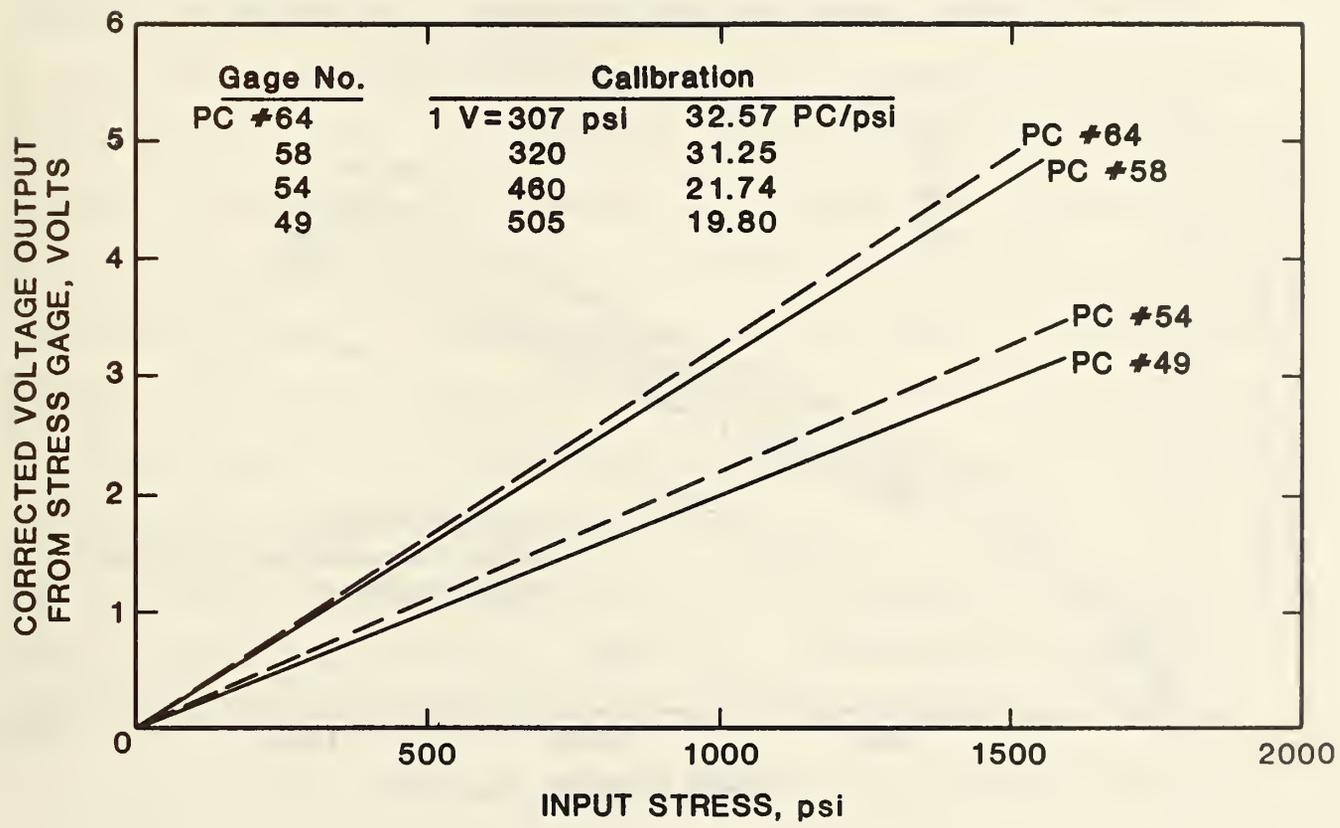
Figure 32 Summary of NBS Polymer Gages Calibrated for Field Testing
