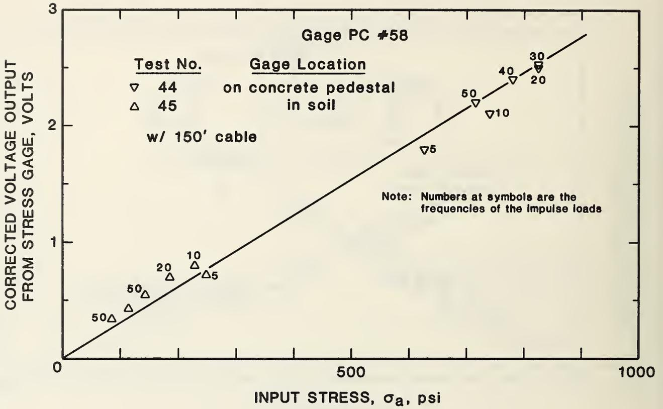
Figure 31 NBS Polymer Gage Test Results - Effect of Frequency, Gage PC #58
