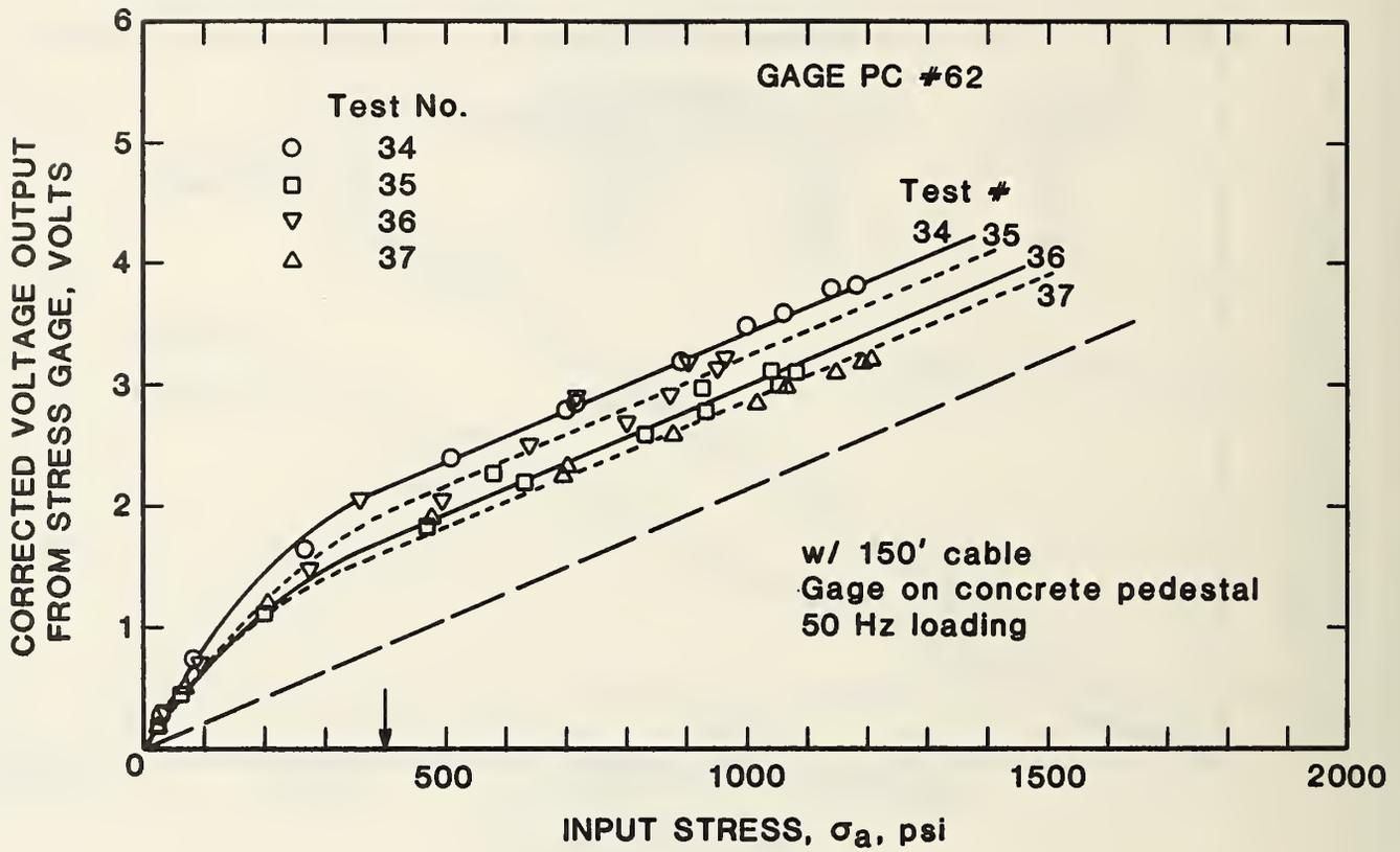
Figure 33 Non-linear Characteristics of The Gage Exhibited During The Testing of Gage PC #62
