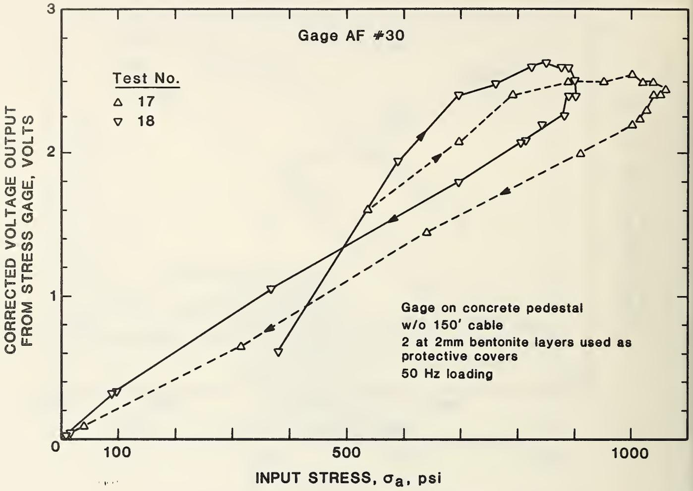
Figure 21 NBS Polymer Gage Test Results - Bentonite Layers Used as a Protective Covering with The Test Cylinder Not Insulated
